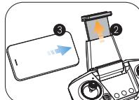
Expand the phone holder and place your mobile phone in it. Adjust the clamp to secure your mobile phone.
