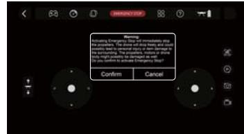
Note: When the **Emergency Stop** is triggered, the propellers **will** immediately stop spinning, and the drone **will** lose control, falling freely from its current height. This could potentially hit people or objects nearby, leading to injury or damage to valuable items. The drone may be broken and the propellers, motors and drone body may be damaged.
