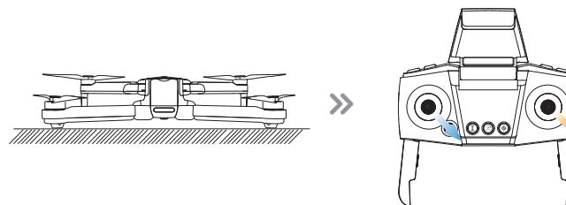
Make sure to place the drone on a level surface before calibrating the gyro. Simultaneously push the left joystick and the right joystick to the bottom right corner to calibrate the gyro. The indicator lights on the drone will blink, then turn solid, which indicates that the calibration is completed.
