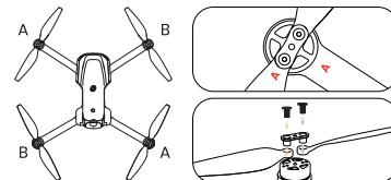
The drone will not fly unless the correct propeller is installed on the correct motor shaft. Each propeller is labeled with either an "A" or "B." Secure the propeller onto the motor shaft using screws, turning each screw clockwise.
