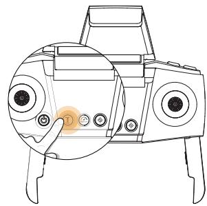
Short press the
