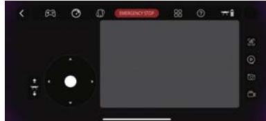
Draw a line freely within the designated box, and the drone will follow the drawn trajectory. During Tap Fly, the drone cannot be manually controlled. Please ensure that there are no people or obstacles within a radius of 16ft, while using this feature to prevent potential injury or damage to the drone. Tap TapFly again to exit Tap Fly mode, the drone will be manually control immediately.
