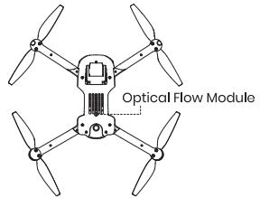
The Optical Flow Positioning System consists of a camera module, which acquires the position information of the drone through visual images to ensure precise positioning of the drone. The optimal usage height for Optical Flow Mode is 1.6-9.8ft.
