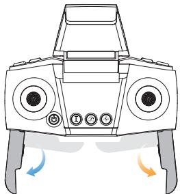
Expand the foldable handles on the transmitter separately.
