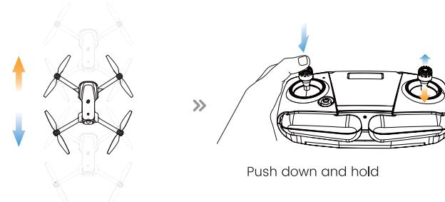
④ **Deactivate Trim Mode:** Once adjustments are made, release the left joystick to exit trim mode.
