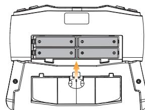
Remove the battery cover on the back of the transmitter. Put in four AAA batteries (not included). Then, put the cover back on.
