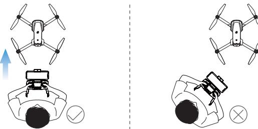
The pilot should stay facing the same direction that the drone's head points to when it takes off.
