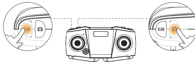
**Record Video:** Short press the
