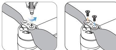
For propeller removal, use a screwdriver (provided) to rotate the screws counter-clockwise and remove the propellers. Be sure to hold the motor while detaching the propeller.
