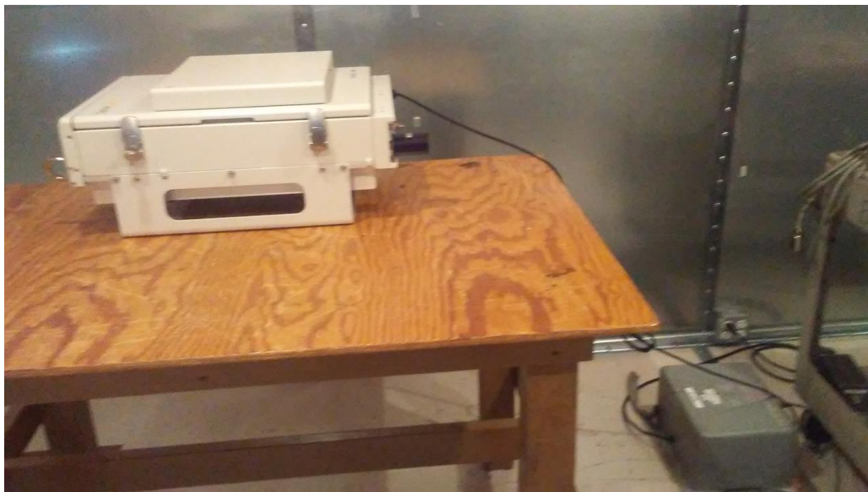
Photograph 1. Conducted Emissions, Test Setup
