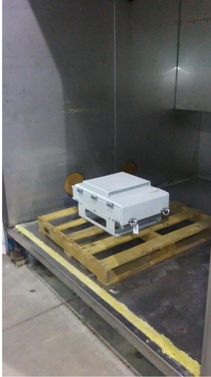
Photograph 4. Temperature Variation, Frequency Stability, Test Setup
