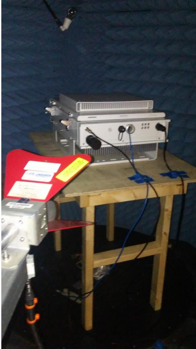
Photograph 3. Radiated Spurious Emissions, Test Setup, Above 1 GHz
