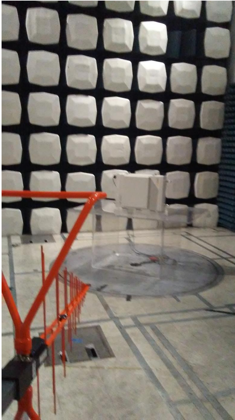
Photograph 2. Radiated Spurious Emissions, Test Setup, 30 MHz – 1 GHz
