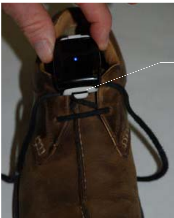
Figure 22. Attaching the Shoe Clip to the Shoe
