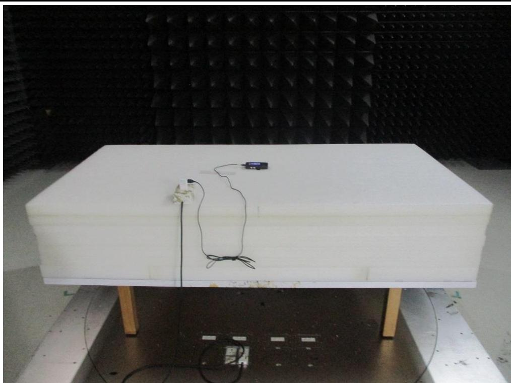
**Radiated Emission Below 1GHz Test**
