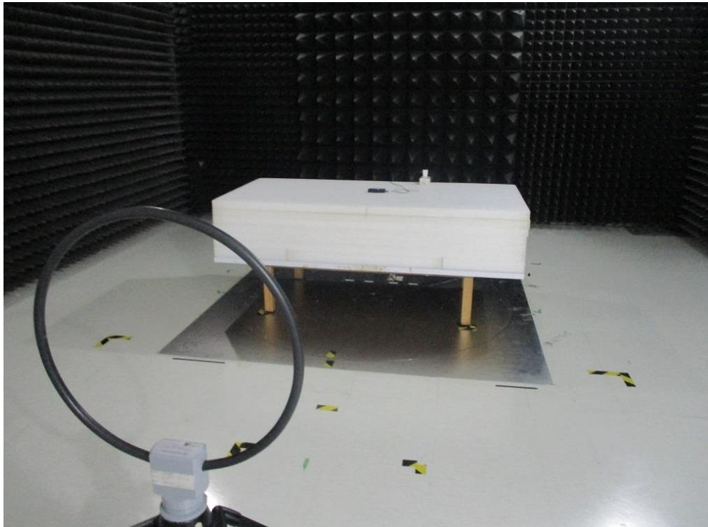
**Radiated Emission Below 1GHz Test**
