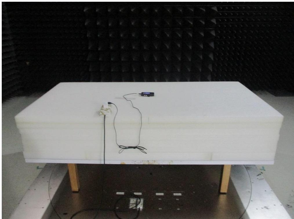
**Radiated Emission Below 30MHz Test**
