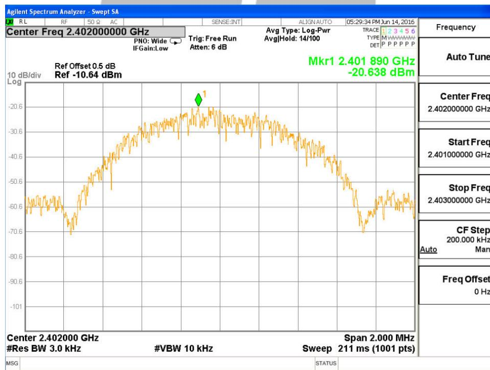
**POWER SPECTRAL DENSITY ( GFSK MODE CH Mid)**
