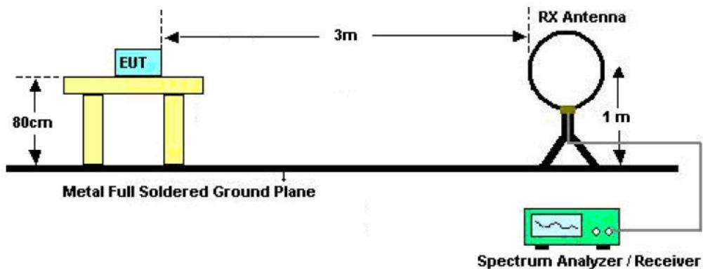
For radiated emission from 30MHz to 1GHz
