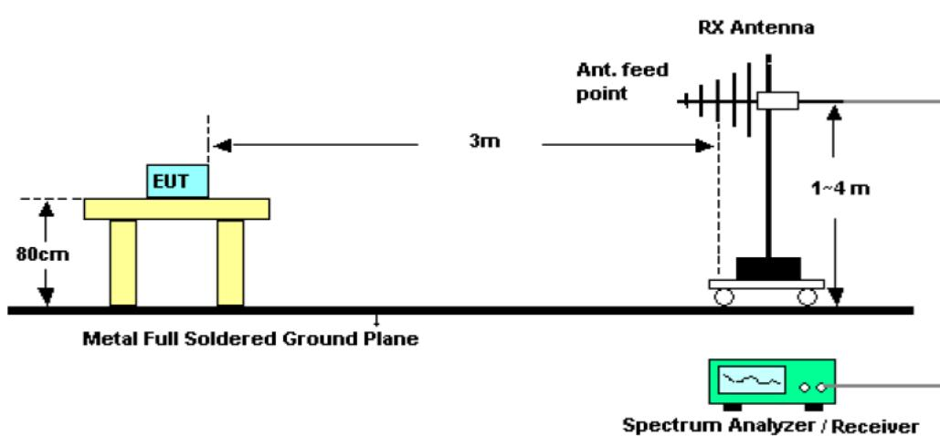
For radiated emission from above 1GHz:
