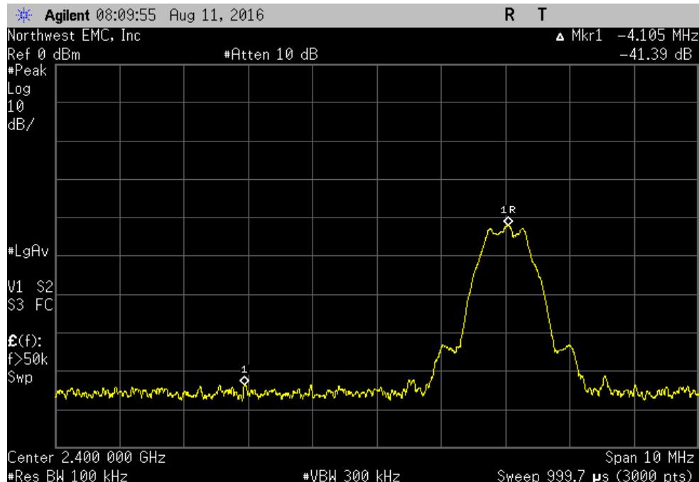
BLE/GFSK High Channel, 2480 MHz
