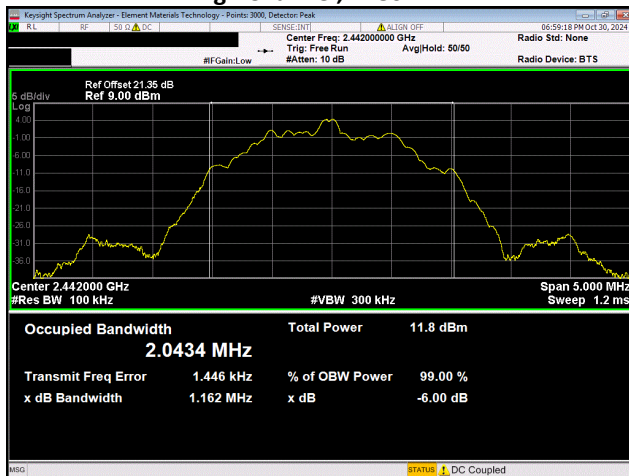
BLE/GFSK 2 Mbps Mid Channel, 2442 MHz
