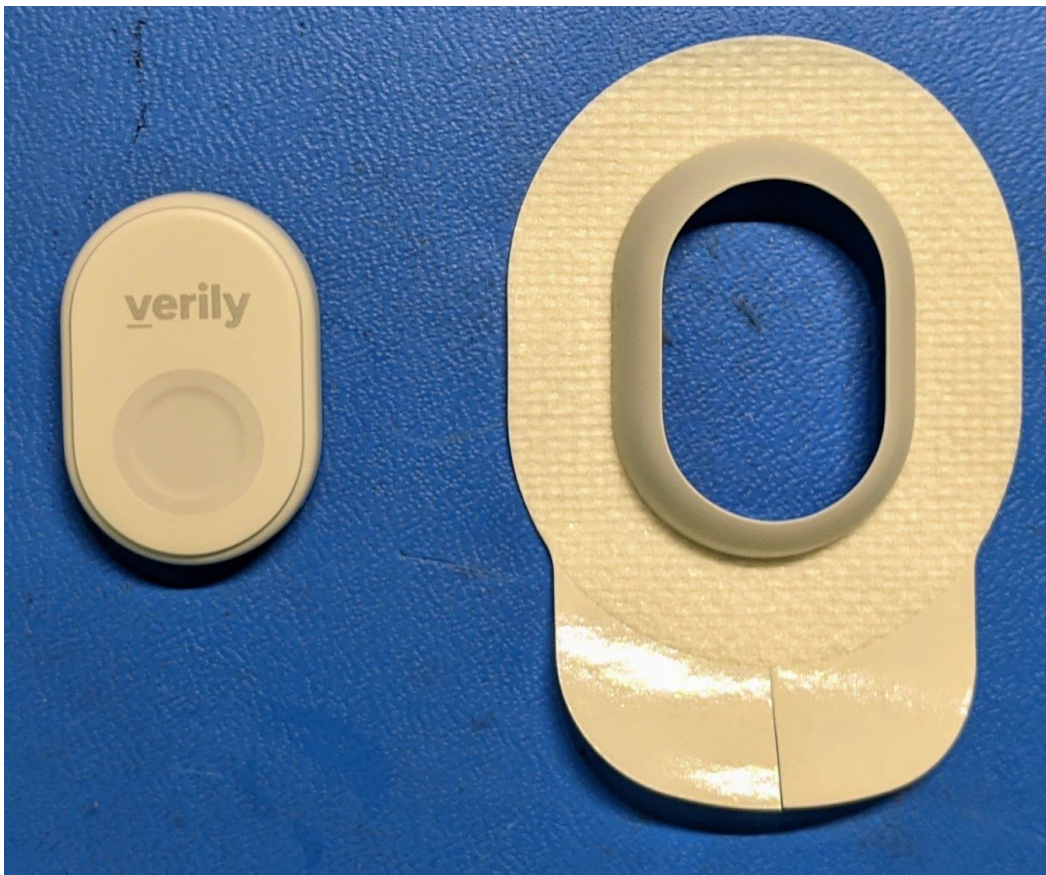
Figure 3: Verily Patch Sensor and adhesive carrier - Front View
