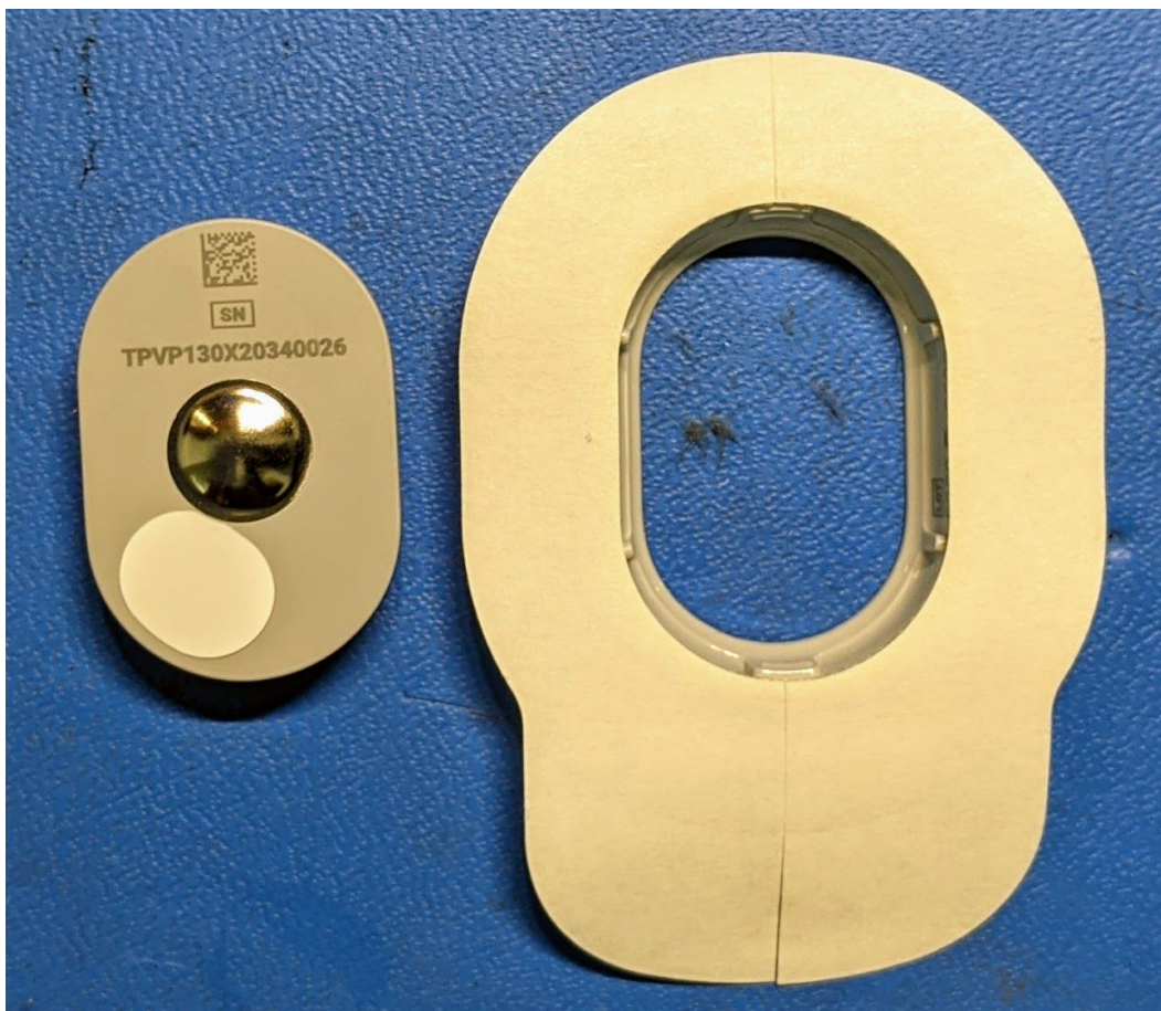
Figure 4: Verily Patch Sensor and adhesive carrier - Back View
