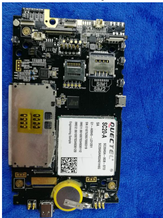
Mainboard with Shielding - Front View
