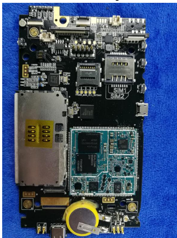
Mainboard without Shielding - Front View
