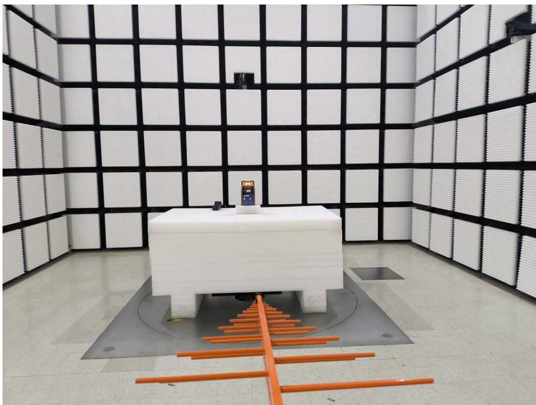
Radiated Emission Above 1GHz View
