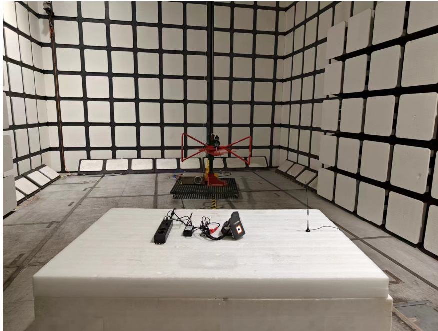
Radiated Emissions View (Below 1 GHz)
