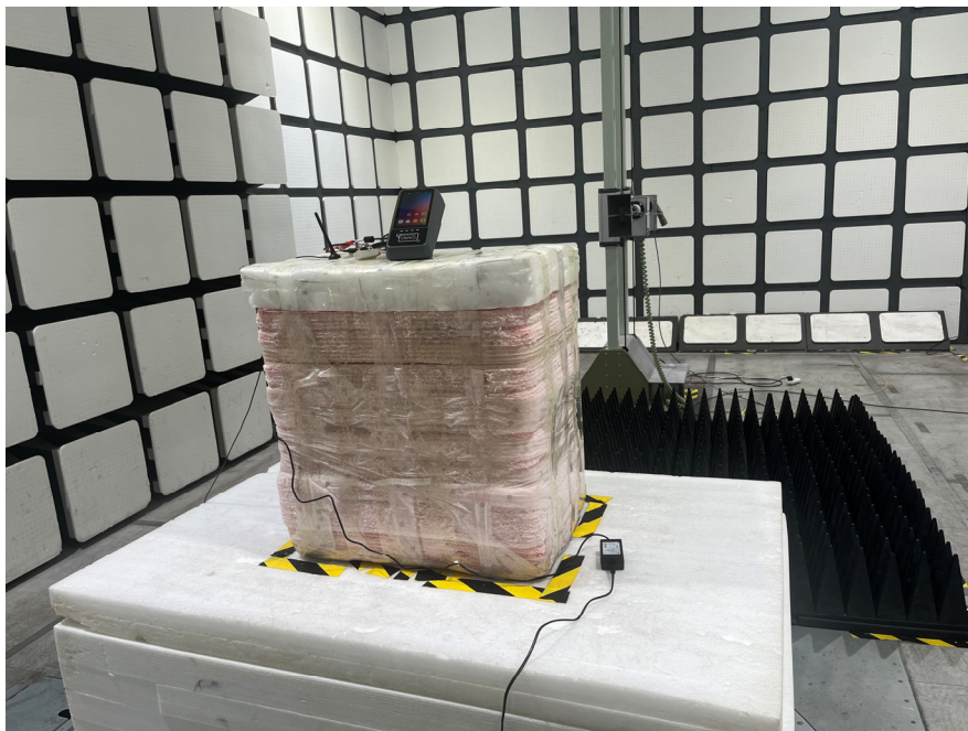
Radiated Emissions View (1-18 GHz)
