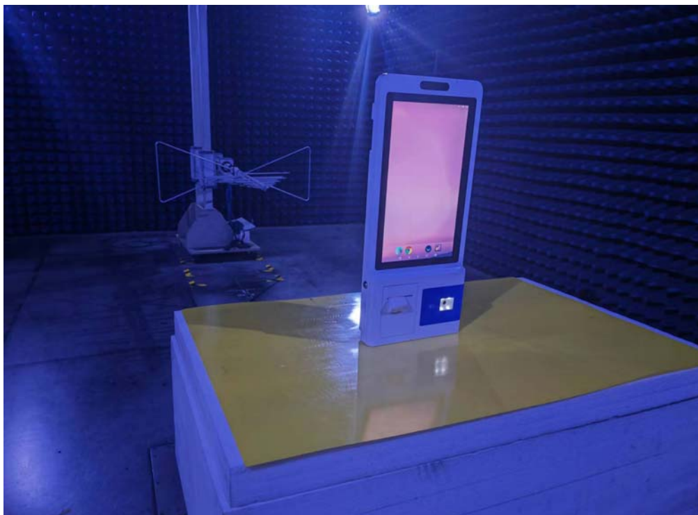
Photo of Radiated Emission Measurement (Above 1G)
