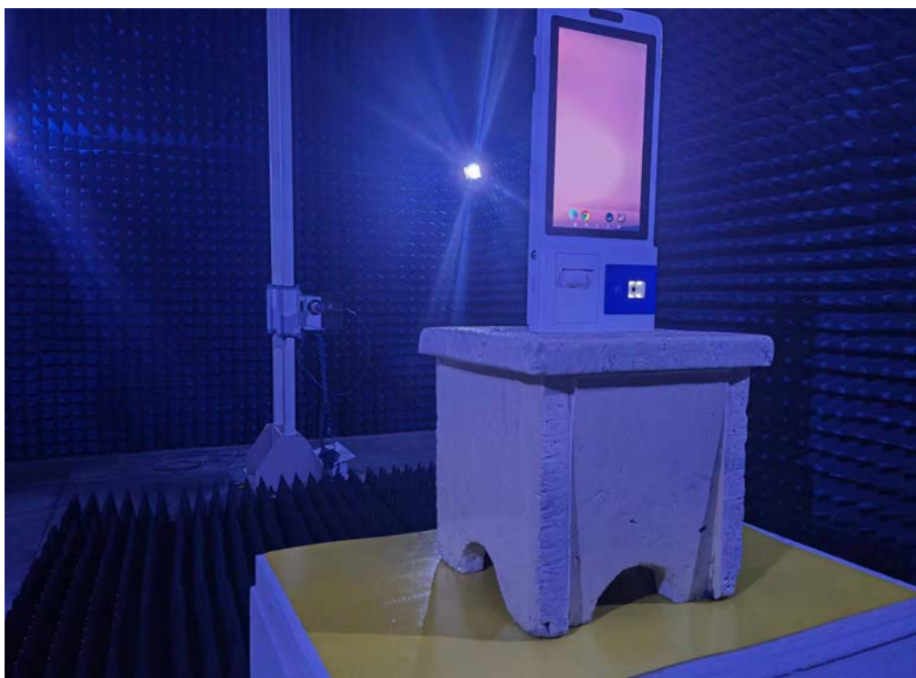
Photo of Radiated Emission Measurement (Above 1G)
