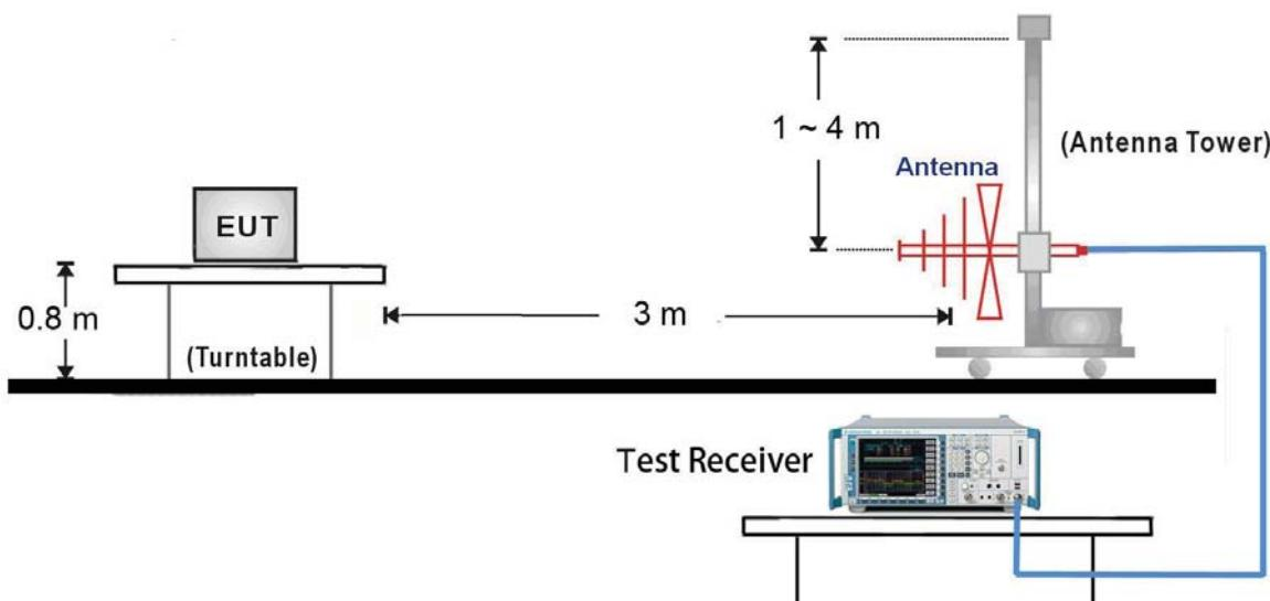
1GHz ~ 25GHz Test Setup:
