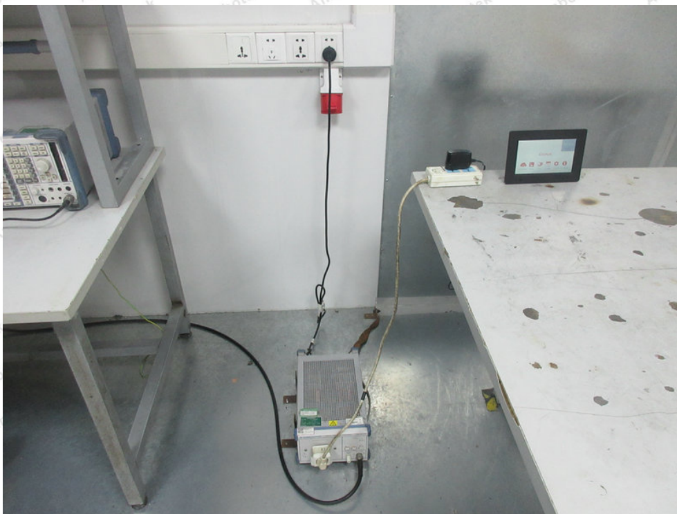
Photo of Power Line Conducted Emission Test
