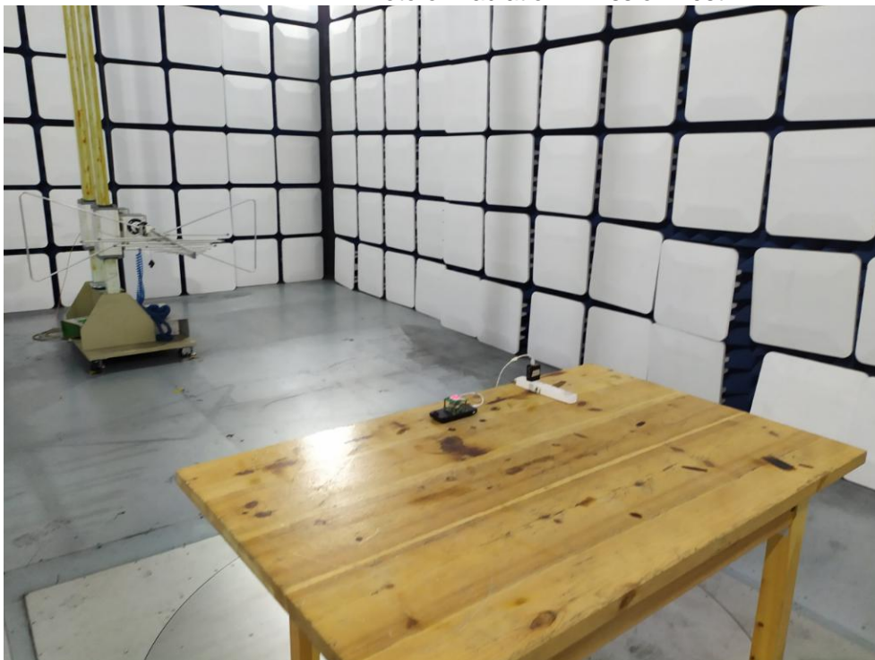
Photo of Radiation Emission Test
