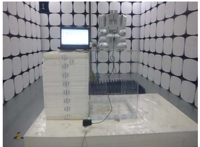
Radiated Spurious Emissions Test Above 1GHz
