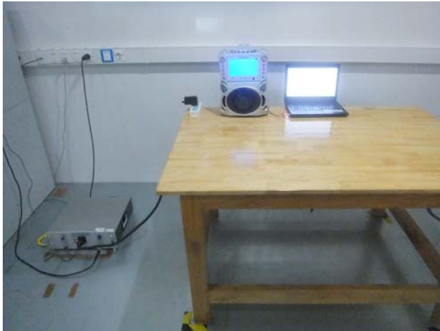
Conducted Emissions Test Setup – Front View
