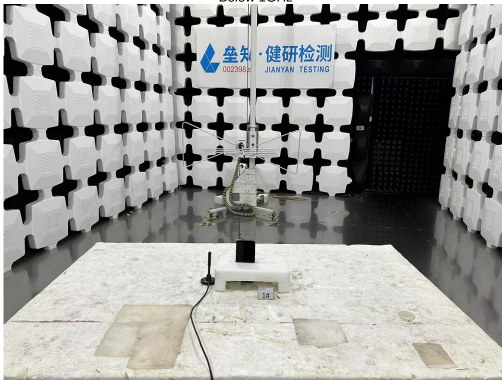
Radiated Spurious Emission Below 1GHz
