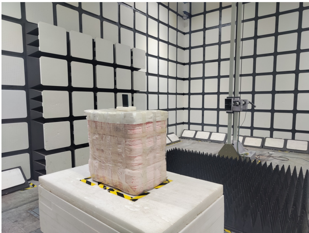
Radiated Emissions View (1-18 GHz)
