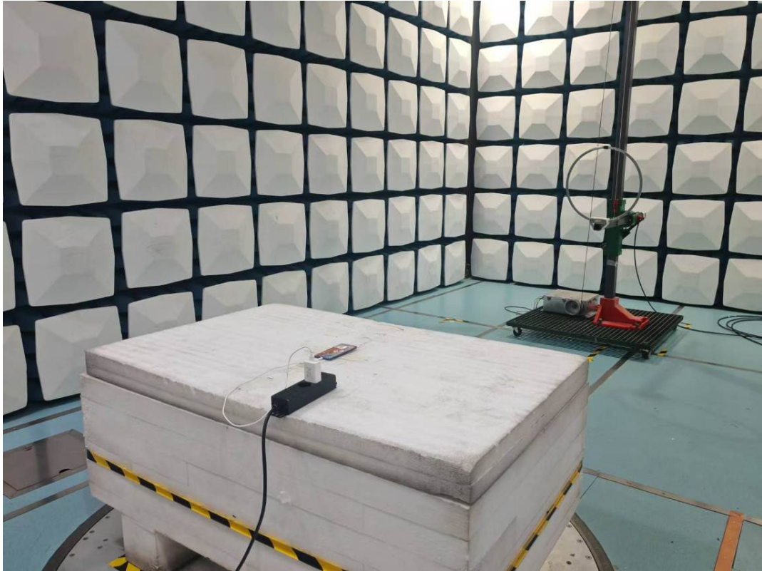
Radiated Emission 9k-30MHz Perpendicular View
