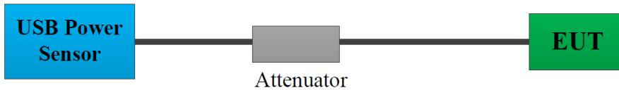
A short RF cable with low cable loss connected to the EUT antenna port, which was provided by manufacturer. The insert loss of this RF cable/attenuator was offset into the setting of test equipment.
