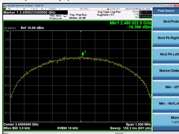
GFSK (BLE 1Mbps) HIGH CHANNEL
