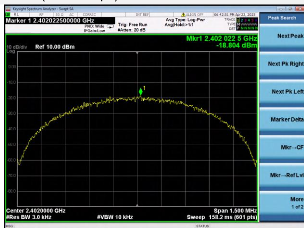
GFSK (BLE 1Mbps) LOW CHANNEL
