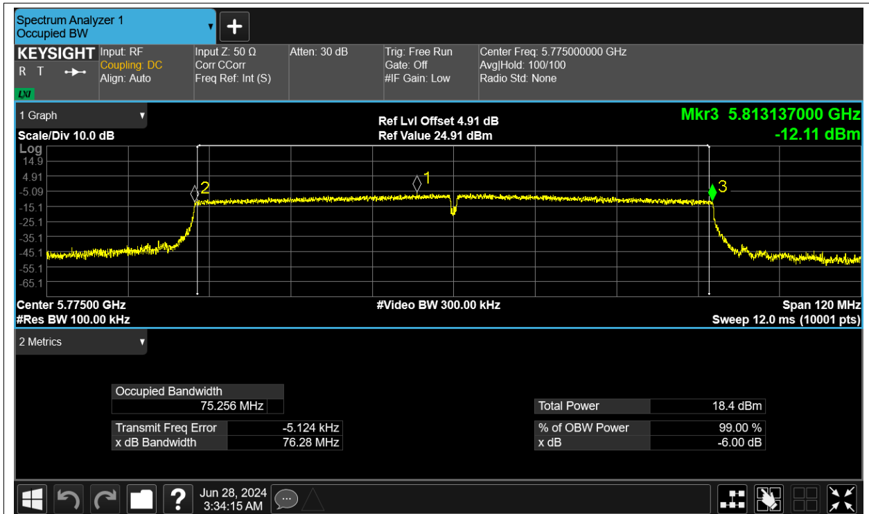
-6dB Bandwidth NVNT n20 5745MHz Ant1
