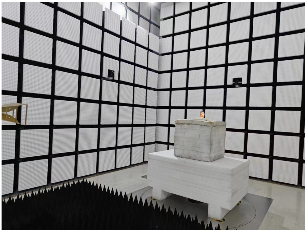
Radiated Emission Above 1GHz View
