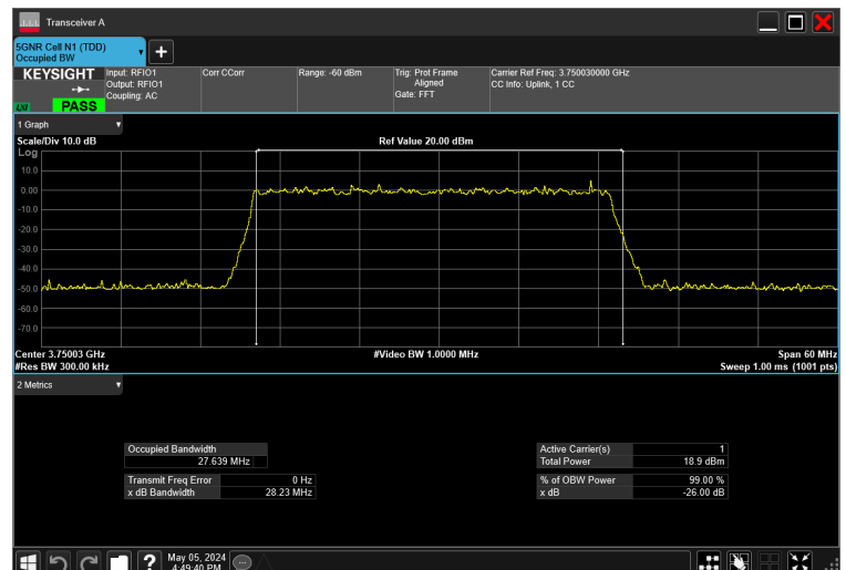
30MHz_30kHz_3750MHz_DFT-s-OFDM \pi/2 BPSK_RB75@0 27.639 MHz
