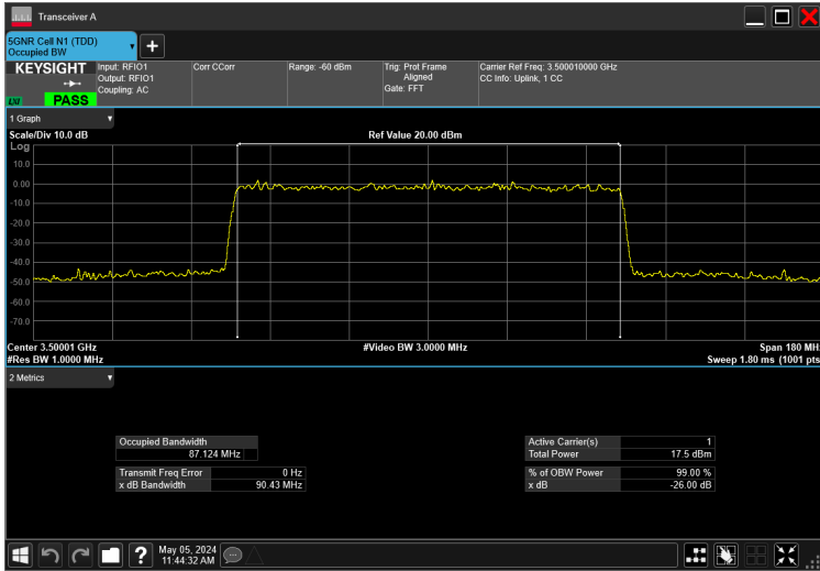
90MHz_30kHz_3500MHz_CP-OFDM 16 QAM_RB245@0 87.124 MHz
