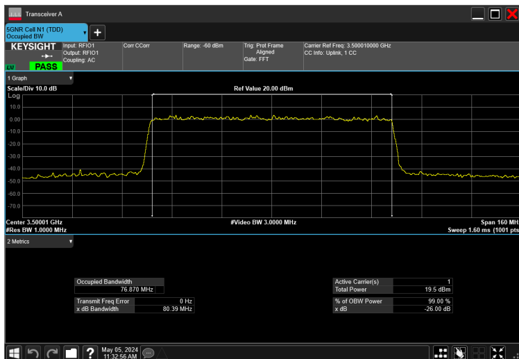
80MHz_30kHz_3500MHz_DFT-s-OFDM QPSK_RB216@0 76.870 MHz
