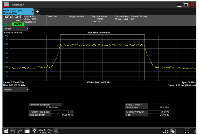
15MHz_30kHz_3750MHz_CP-OFDM 16 QAM_RB38@0 13.562 MHz
