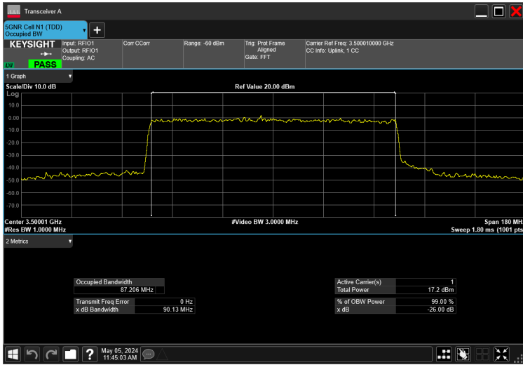
90MHz_30kHz_3500MHz_CP-OFDM 64 QAM_RB245@0 87.206 MHz
