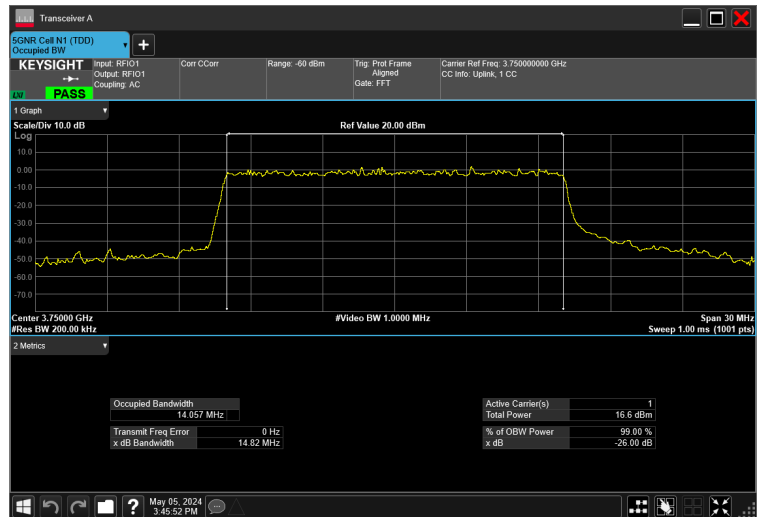
15MHz_15kHz_3750MHz_CP-OFDM QPSK_RB79@0 14.057 MHz
