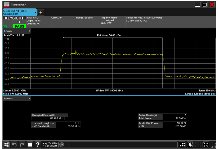
90MHz_30kHz_3500MHz_CP-OFDM QPSK_RB245@0 87.203 MHz
