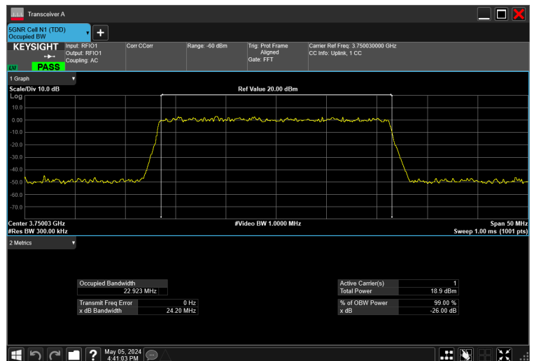
25MHz_30kHz_3750MHz_DFT-s-OFDM \pi/2 BPSK_RB64@0 22.923 MHz
