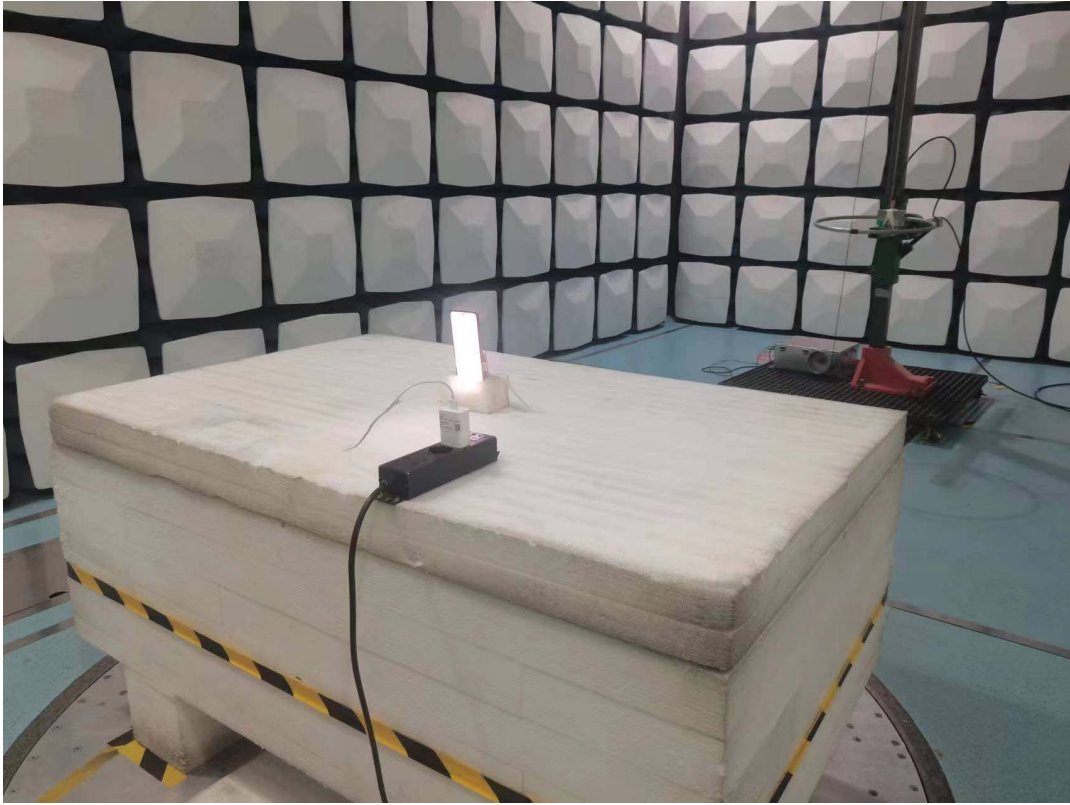
Radiated Emission 30M-1GHz front View
