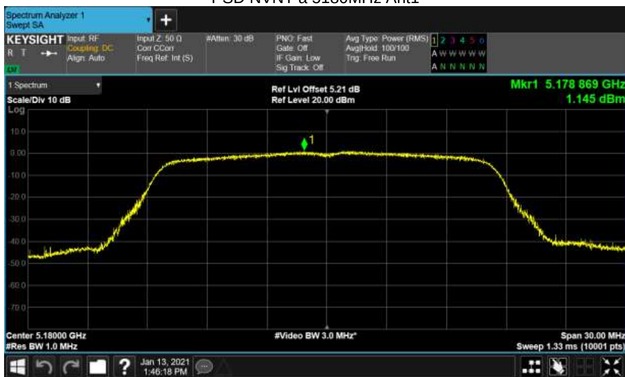
PSD NVNT a 5180MHz Ant1
