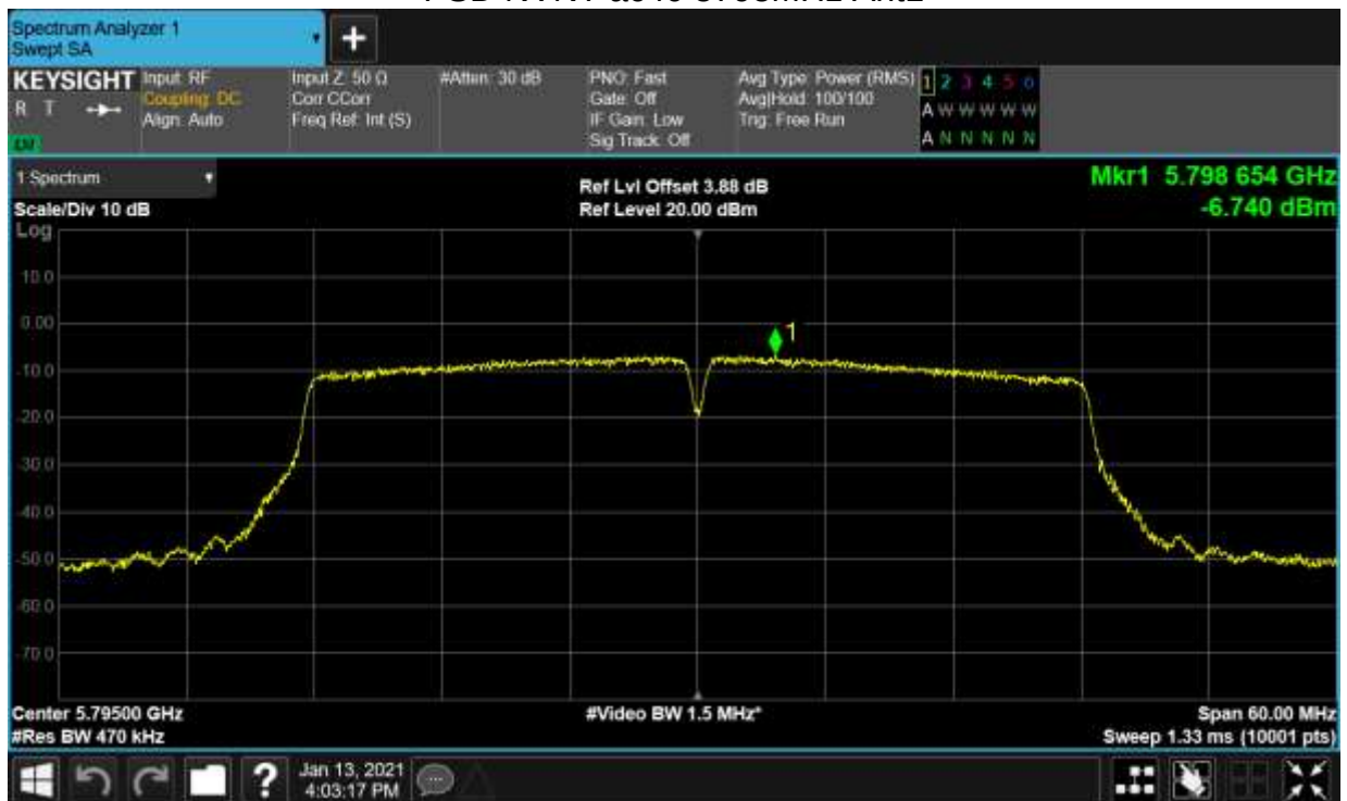
PSD NVNT ac40 5795MHz Ant1
