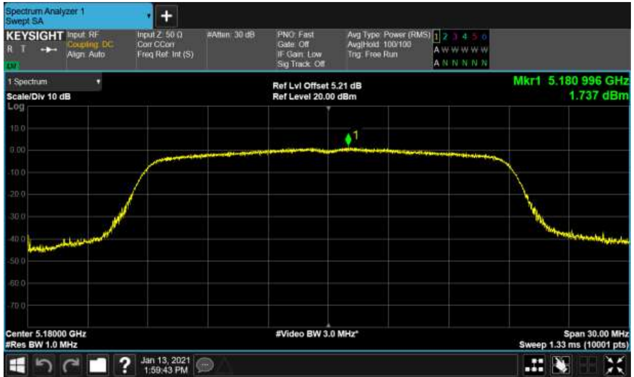
PSD NVNT ac20 5200MHz Ant1
