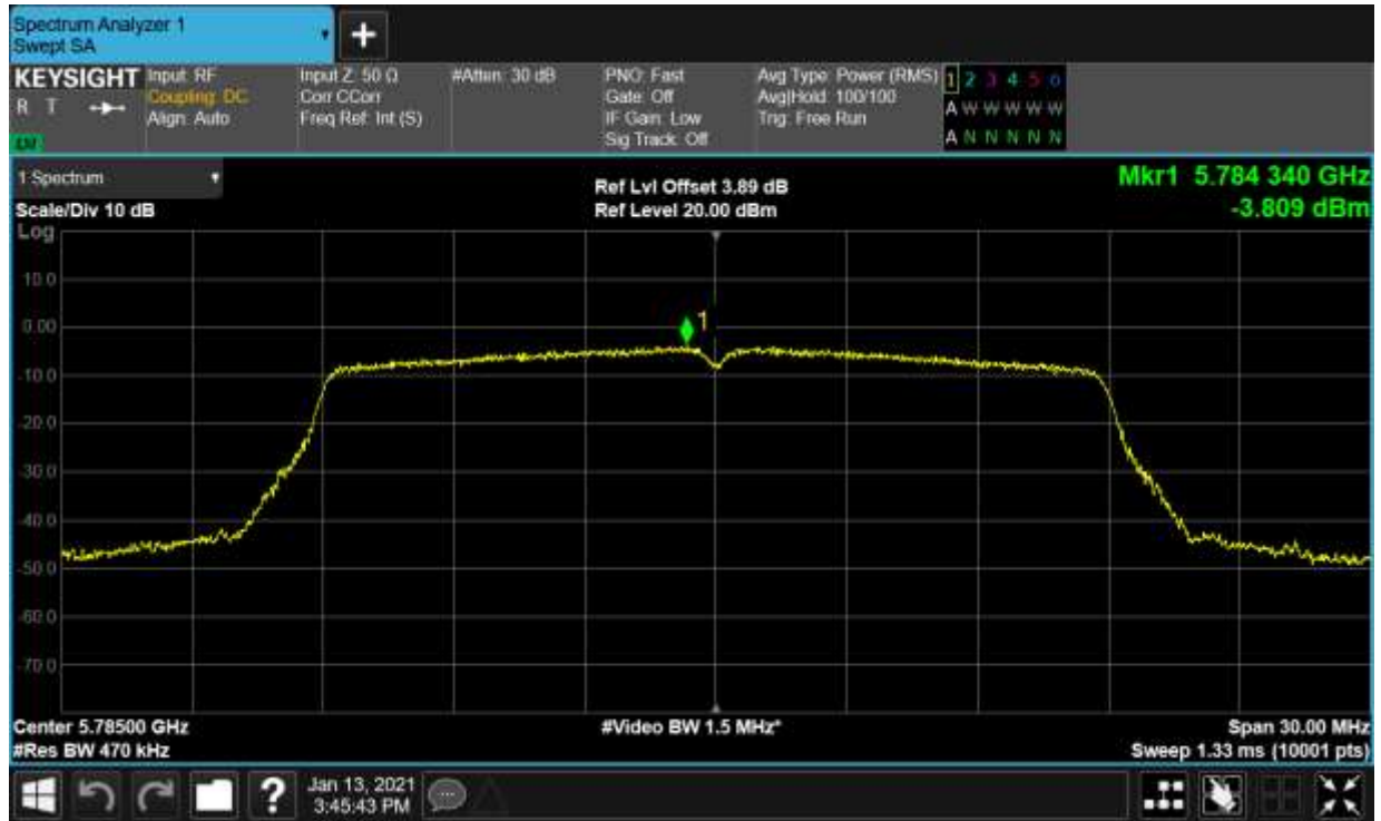
PSD NVNT ac20 5825MHz Ant1
