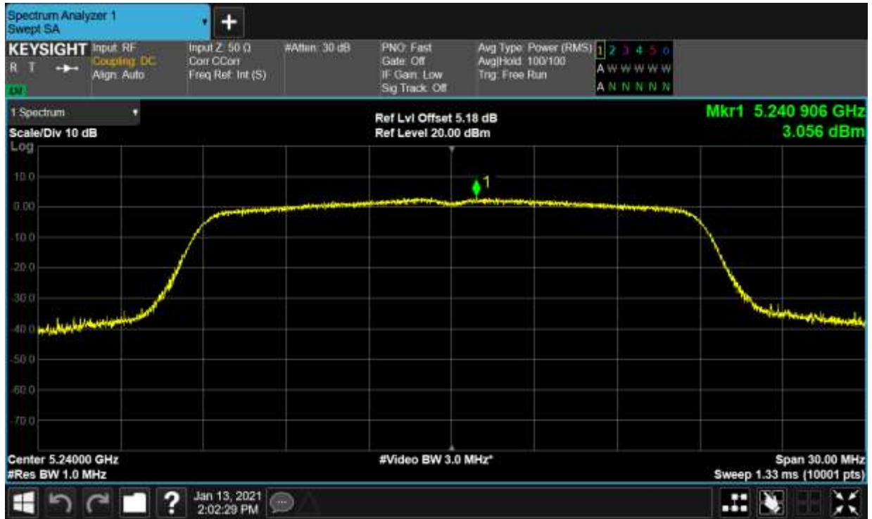
PSD NVNT ac40 5190MHz Ant1
