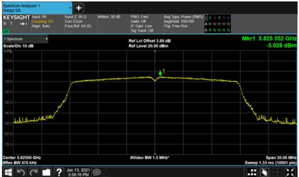
PSD NVNT n20 5825MHz Ant1
