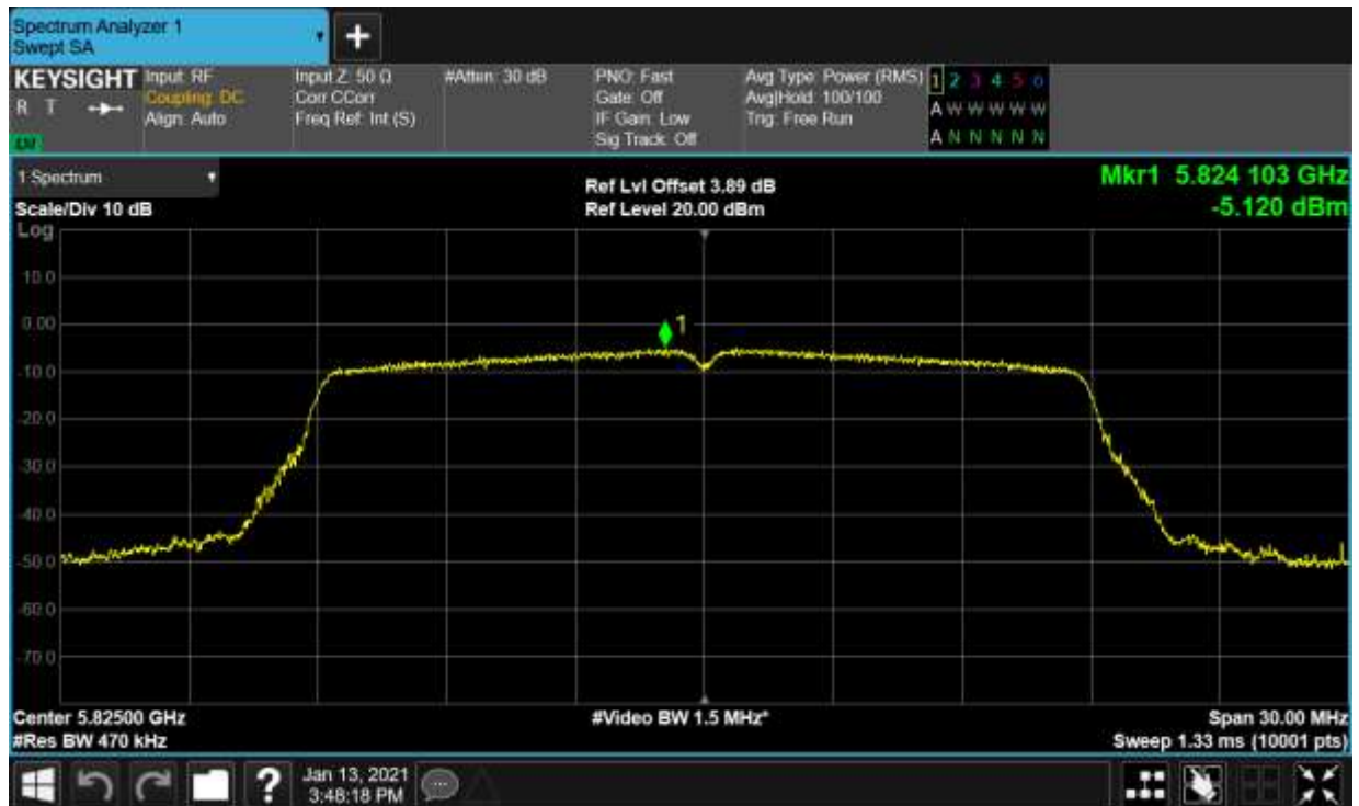
PSD NVNT ac20 5825MHz Ant1
