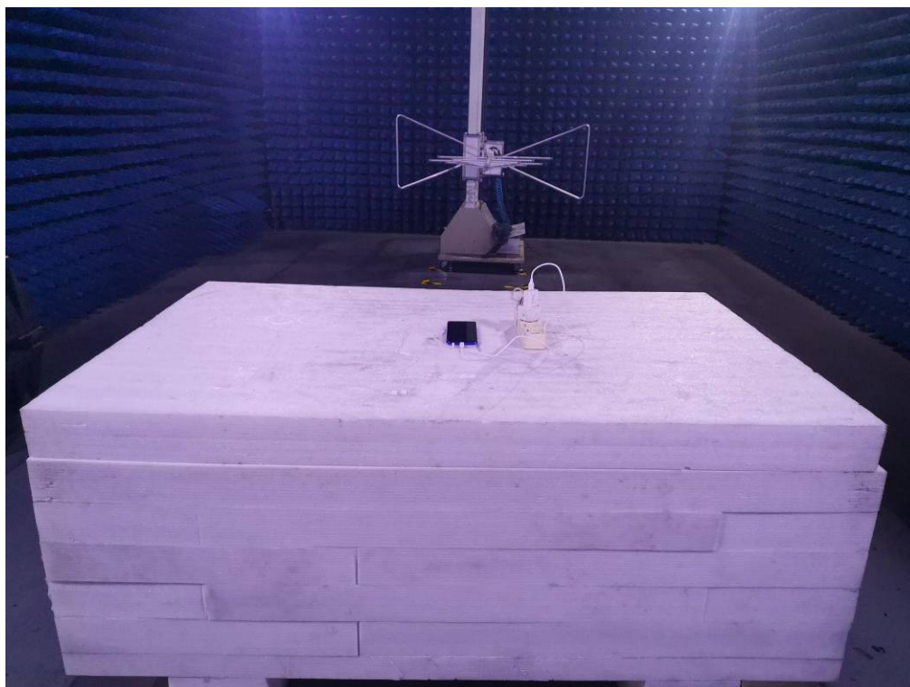
Photo of Radiated Emission Measurement (Above 1G)
