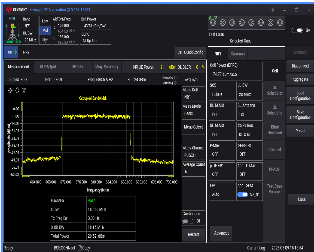
n71 SCS=15kHz DFT_QAM256 BW=15MHz Channel=136100 RB=75@0
