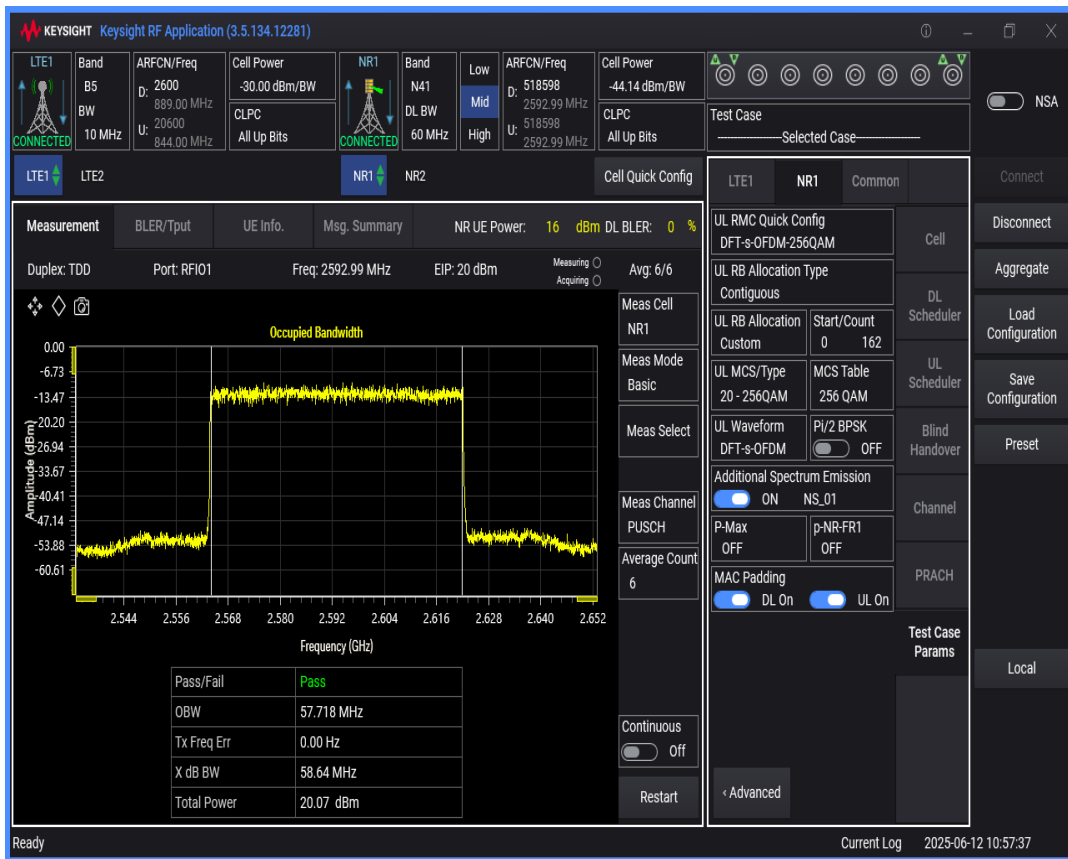
n41 SCS=30kHz DFT_QAM256 BW=50MHz Channel=518598 RB=128@0
