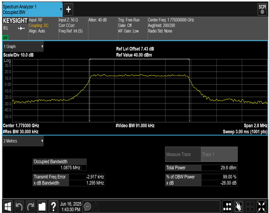
Band66 QAM16 BW=10MHz Channel=132022 RB Size=50 Position=#0
