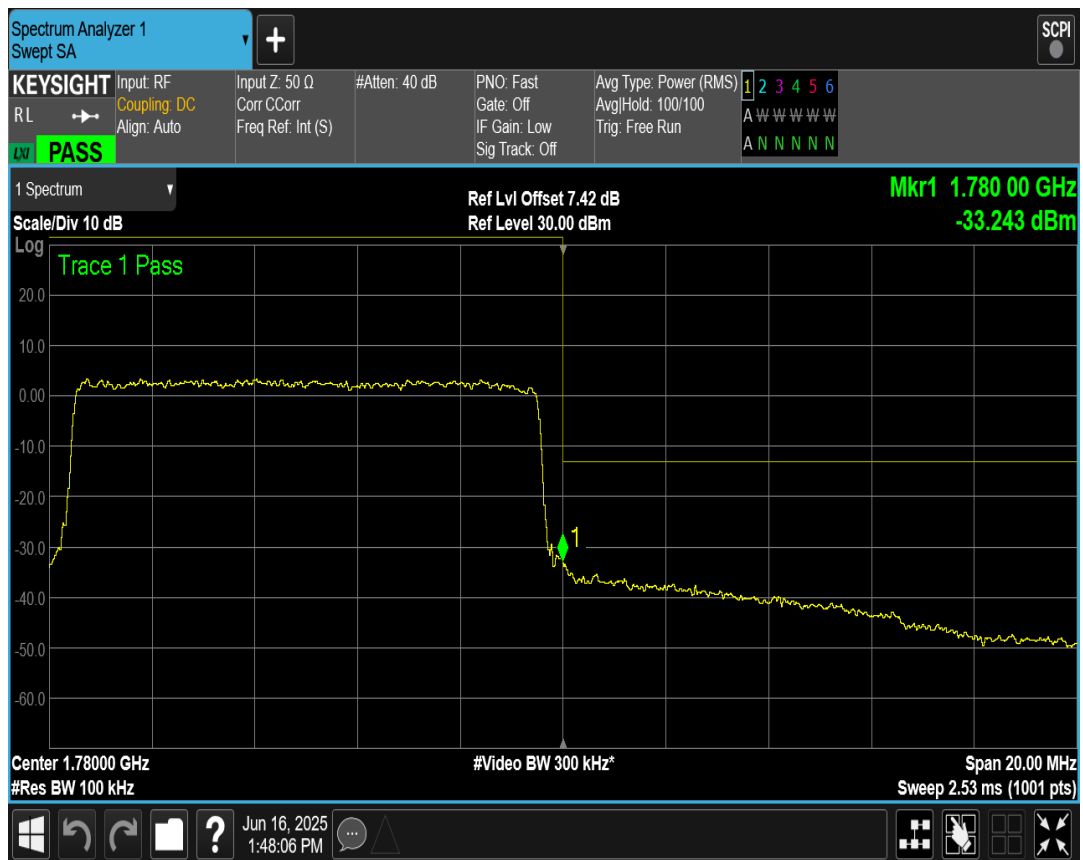
Band66 QAM16 BW=15MHz Channel=132047 RB Size=75 Position=#0
