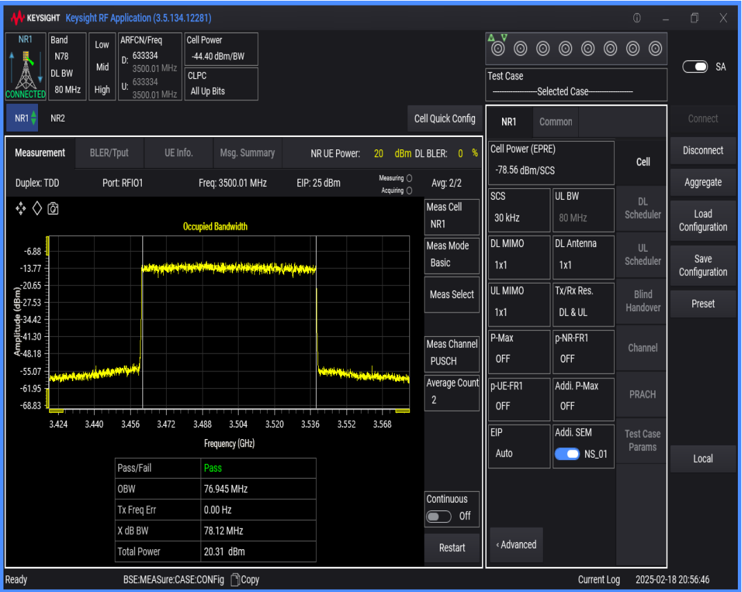
n78(3450-3550) SCS=30kHz DFT_QAM256 BW=90MHz Channel=633334 RB=240@0
