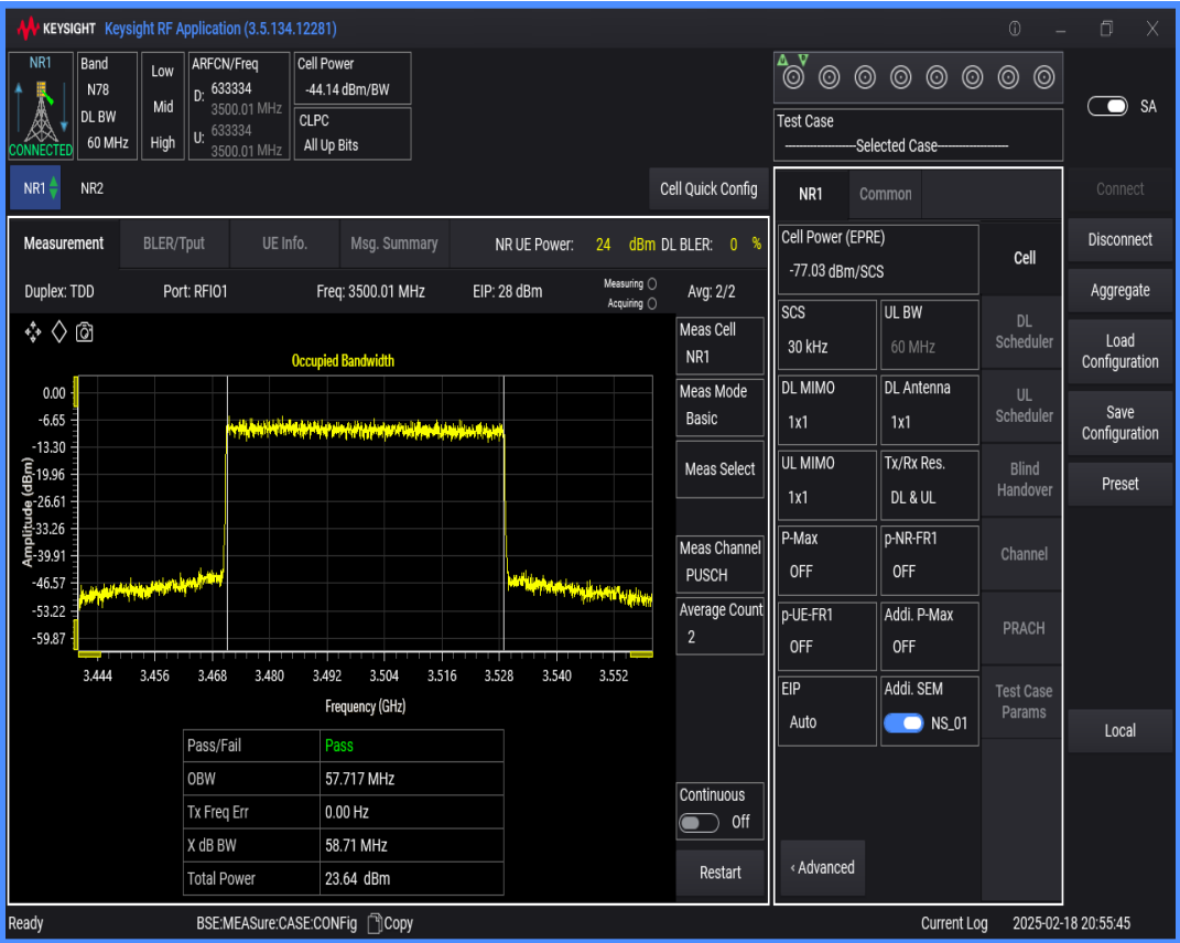
n78(3450-3550) SCS=30kHz DFT_QPSK BW=50MHz Channel=633334 RB=128@0
