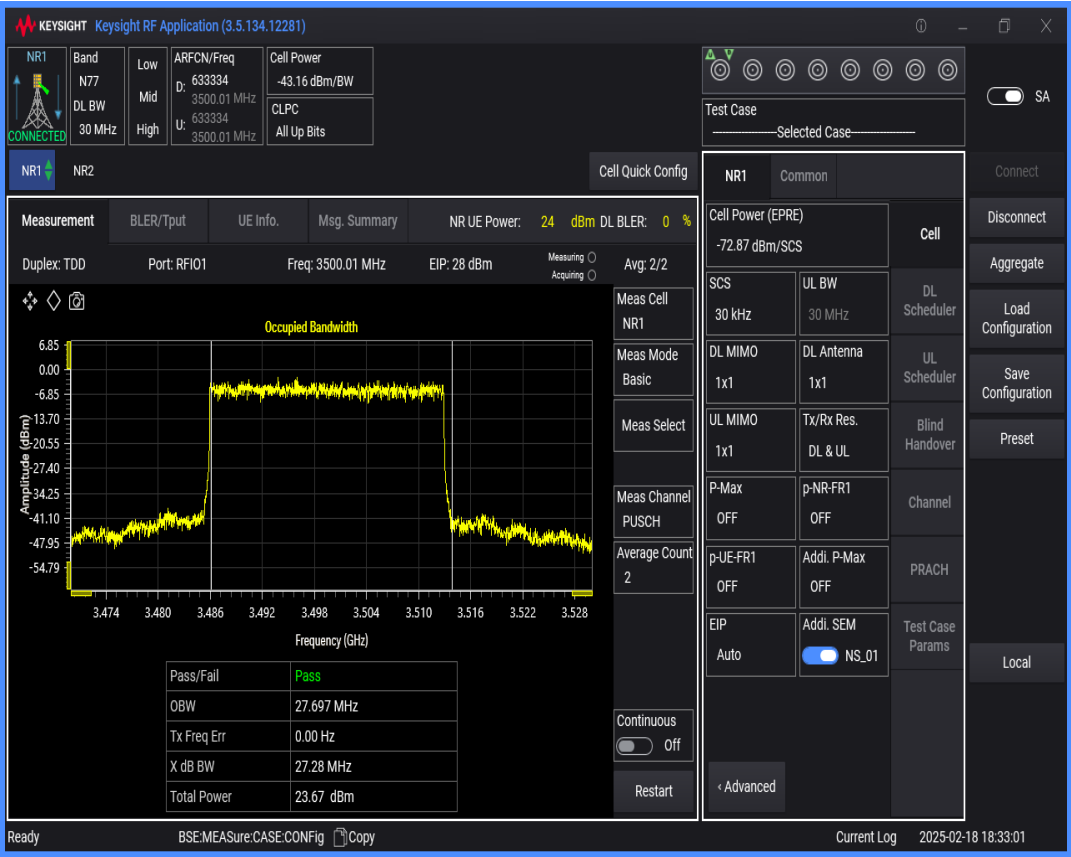
n77(3450-3550) SCS=30kHz DFT_QPSK BW=40MHz Channel=633334 RB=100@0
