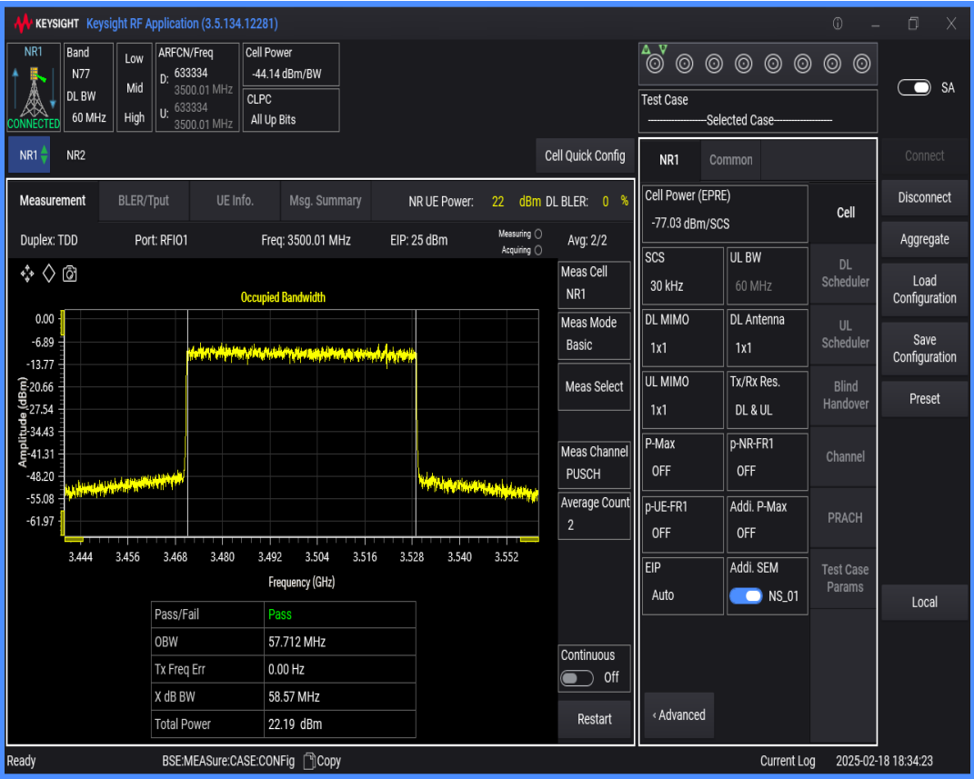
n77(3450-3550) SCS=30kHz DFT_QPSK BW=100MHz Channel=633334 RB=270@0
