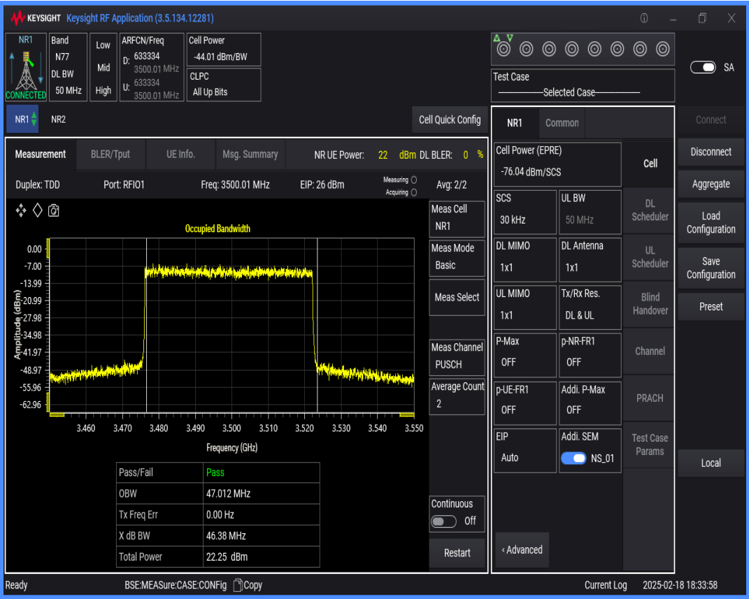
n77(3450-3550) SCS=30kHz DFT_QAM64 BW=80MHz Channel=633334 RB=216@0
