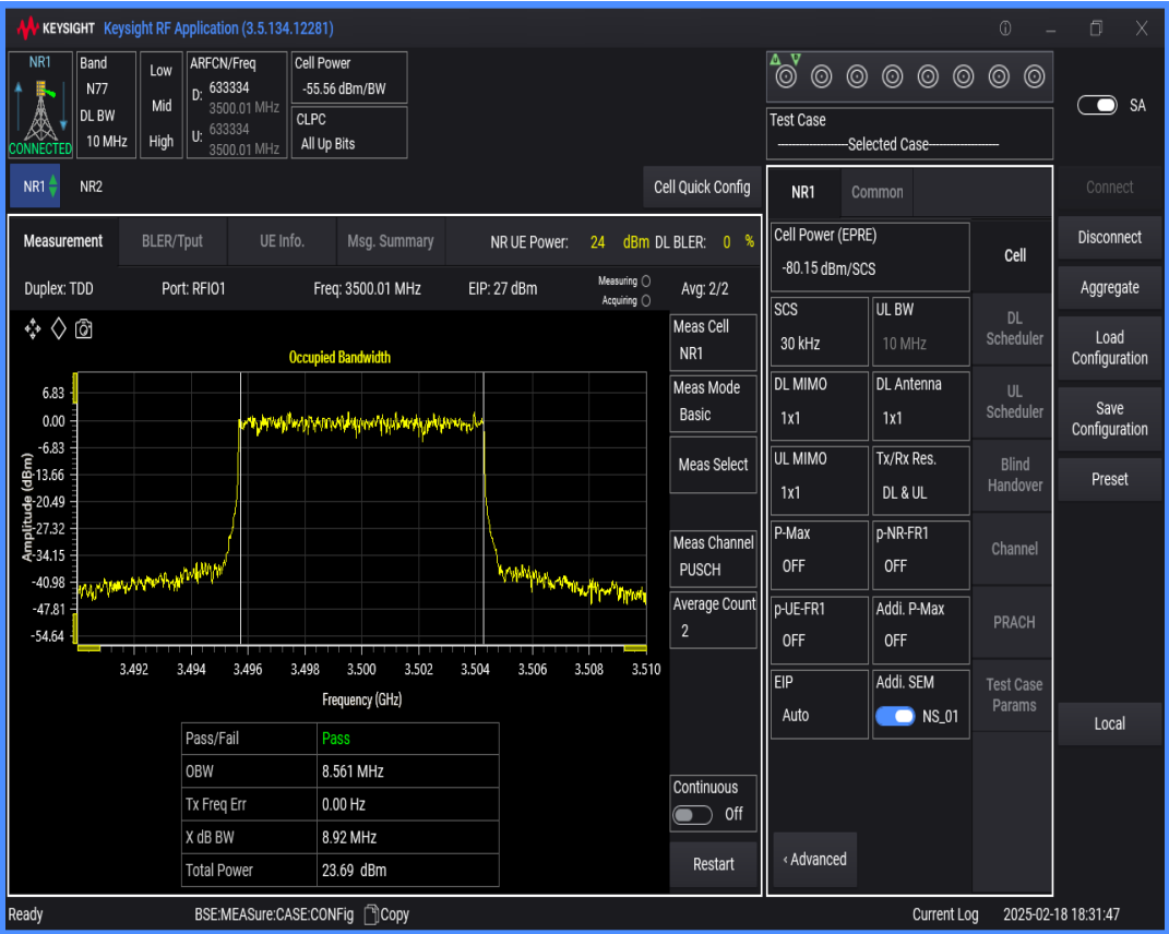
n77(3450-3550) SCS=30kHz DFT_QPSK BW=15MHz Channel=633334 RB=36@0
