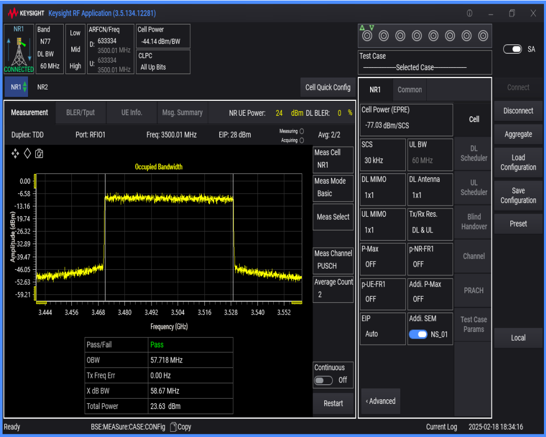
n77(3450-3550) SCS=30kHz DFT_QPSK BW=50MHz Channel=633334 RB=128@0
