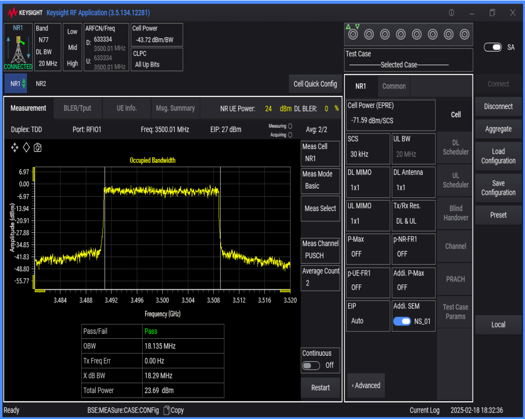
n77(3450-3550) SCS=30kHz DFT_QPSK BW=30MHz Channel=633334 RB=75@0
