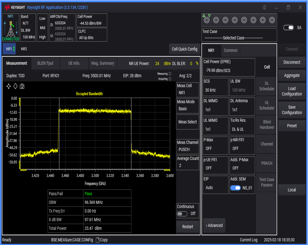
n77(3450-3550) SCS=30kHz DFT_QAM64 BW=90MHz Channel=633334 RB=240@0
