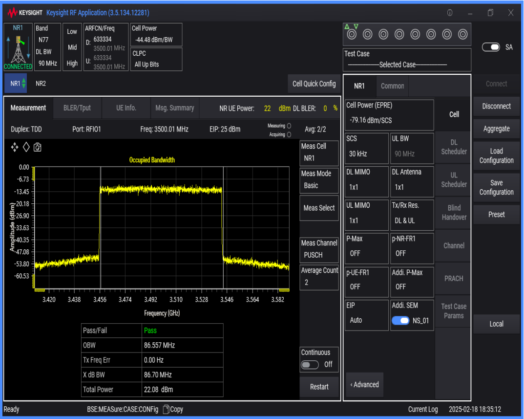
n77(3450-3550) SCS=30kHz DFT_QPSK BW=10MHz Channel=633334 RB=24@0
