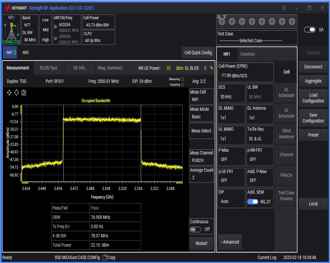
n77(3450-3550) SCS=30kHz DFT_QAM64 BW=60MHz Channel=633334 RB=162@0
