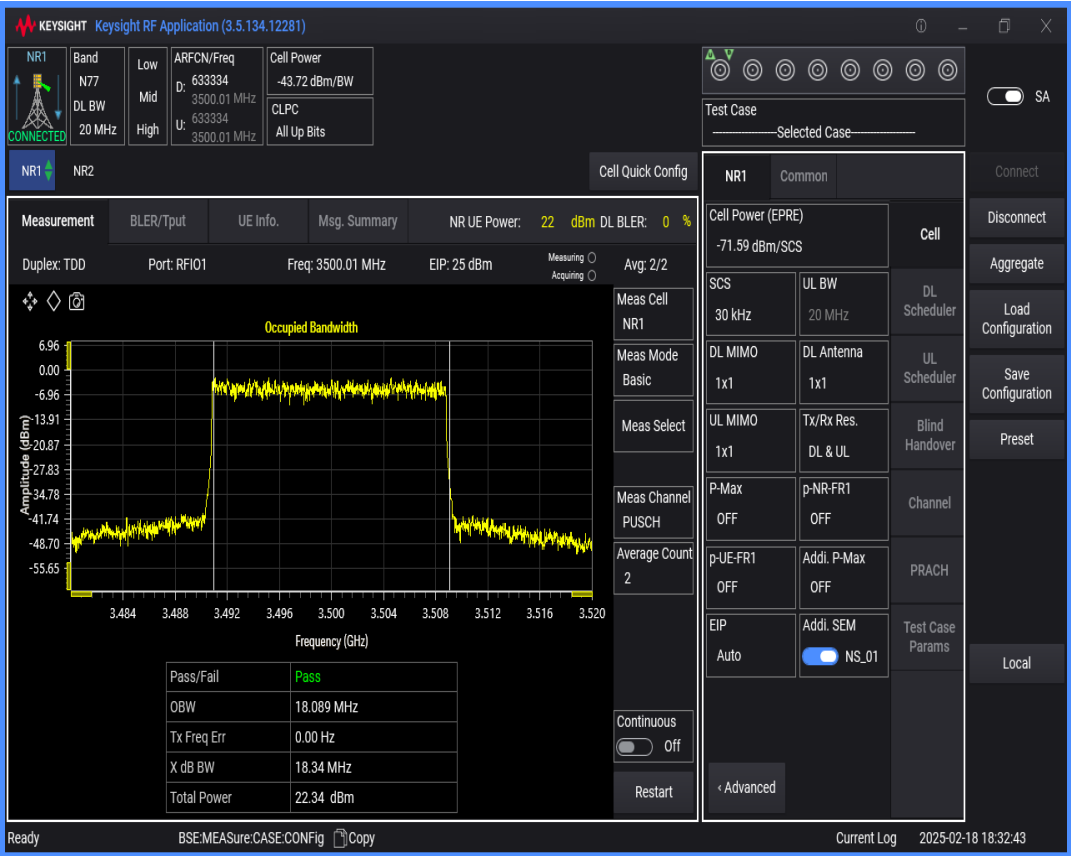
n77(3450-3550) SCS=30kHz DFT_QAM64 BW=50MHz Channel=633334 RB=128@0
