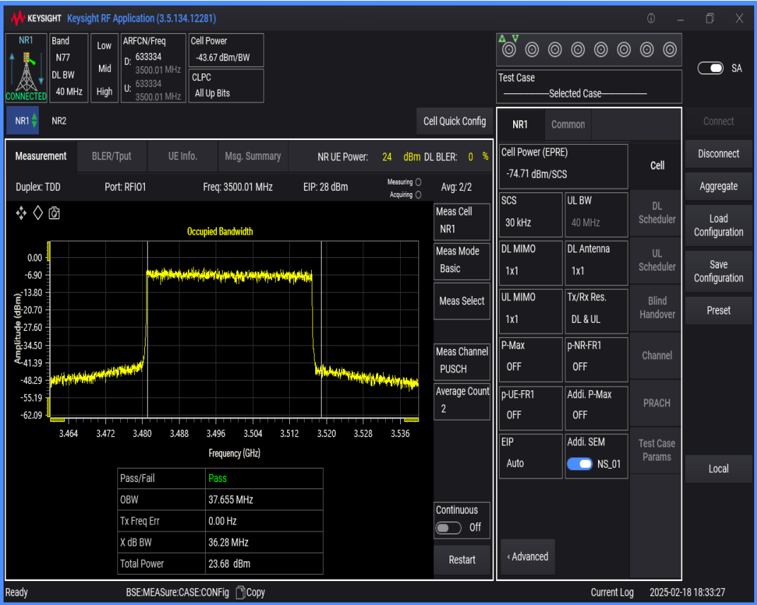
n77(3450-3550) SCS=30kHz DFT_QPSK BW=60MHz Channel=633334 RB=162@0
