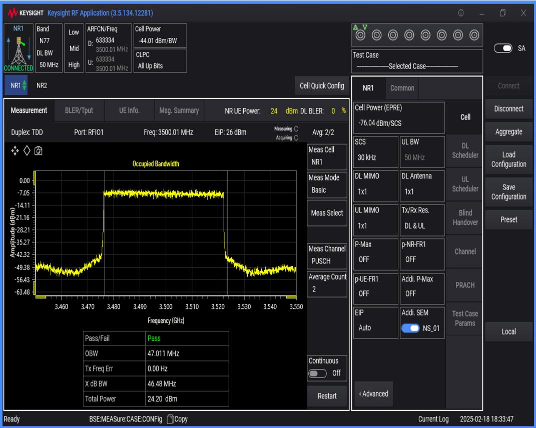
n77(3450-3550) SCS=30kHz DFT_BPSK BW=90MHz Channel=633334 RB=240@0
