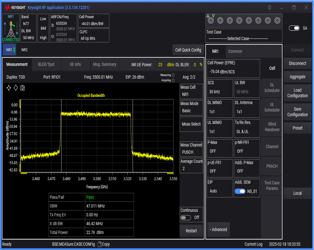
n77(3450-3550) SCS=30kHz DFT_QAM256 BW=100MHz Channel=633334 RB=270@0
