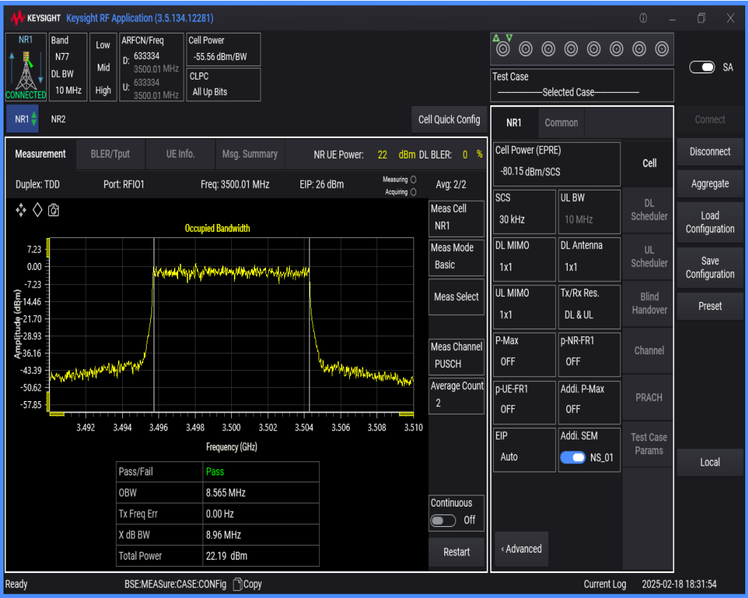
n77(3450-3550) SCS=30kHz DFT_QAM64 BW=40MHz Channel=633334 RB=100@0
