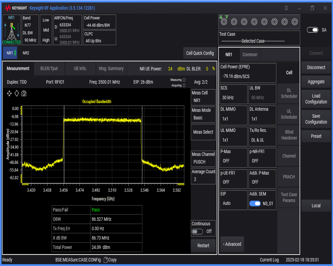
n77(3450-3550) SCS=30kHz DFT_BPSK BW=80MHz Channel=633334 RB=216@0
