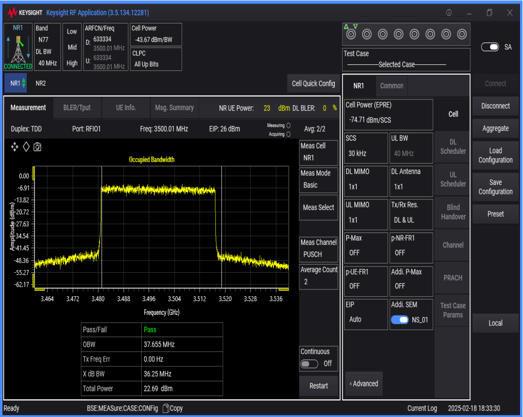
n77(3450-3550) SCS=30kHz DFT_QAM16 BW=50MHz Channel=633334 RB=128@0
