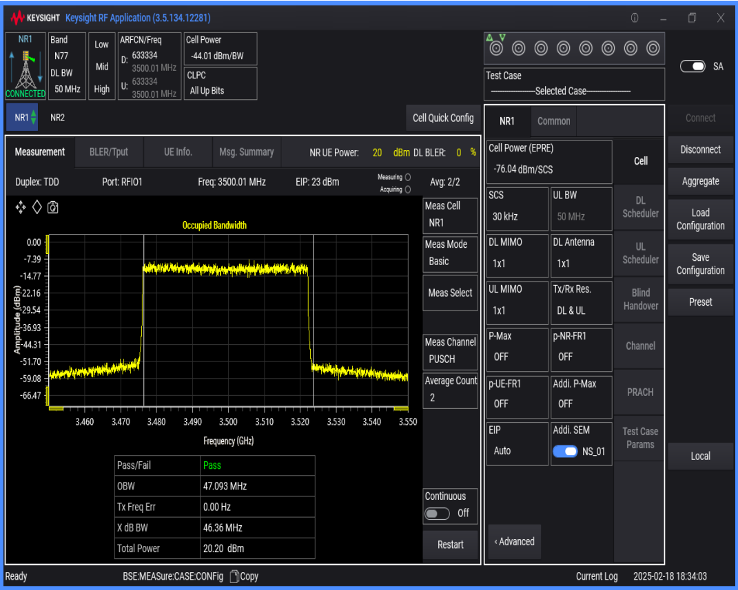
n77(3450-3550) SCS=30kHz DFT_QAM64 BW=100MHz Channel=633334 RB=270@0
