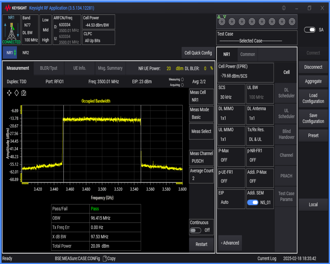
n77(3450-3550) SCS=30kHz DFT_QAM16 BW=90MHz Channel=633334 RB=240@0
