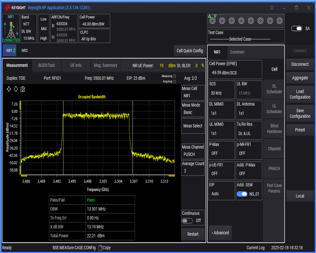
n77(3450-3550) SCS=30kHz DFT_QAM64 BW=10MHz Channel=633334 RB=24@0
