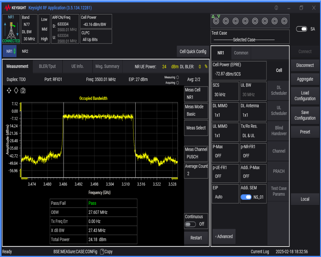
n77(3450-3550) SCS=30kHz DFT_BPSK BW=60MHz Channel=633334 RB=162@0
