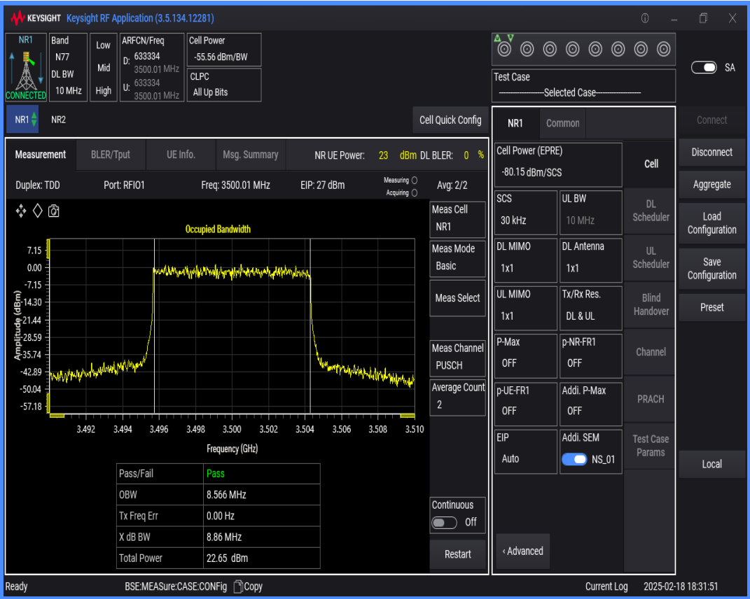
n77(3450-3550) SCS=30kHz DFT_QAM16 BW=100MHz Channel=633334 RB=270@0
