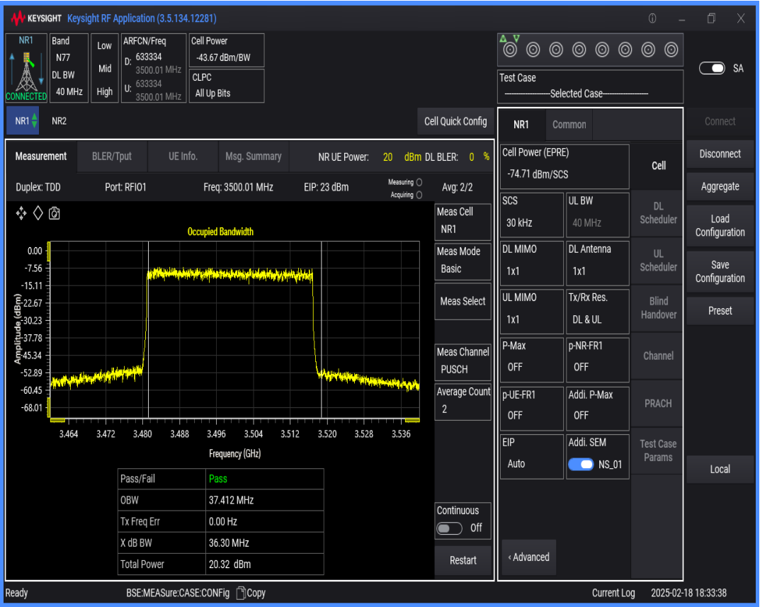
n77(3450-3550) SCS=30kHz DFT_QAM256 BW=30MHz Channel=633334 RB=75@0
