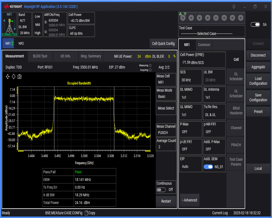
n77(3450-3550) SCS=30kHz DFT_BPSK BW=15MHz Channel=633334 RB=36@0
