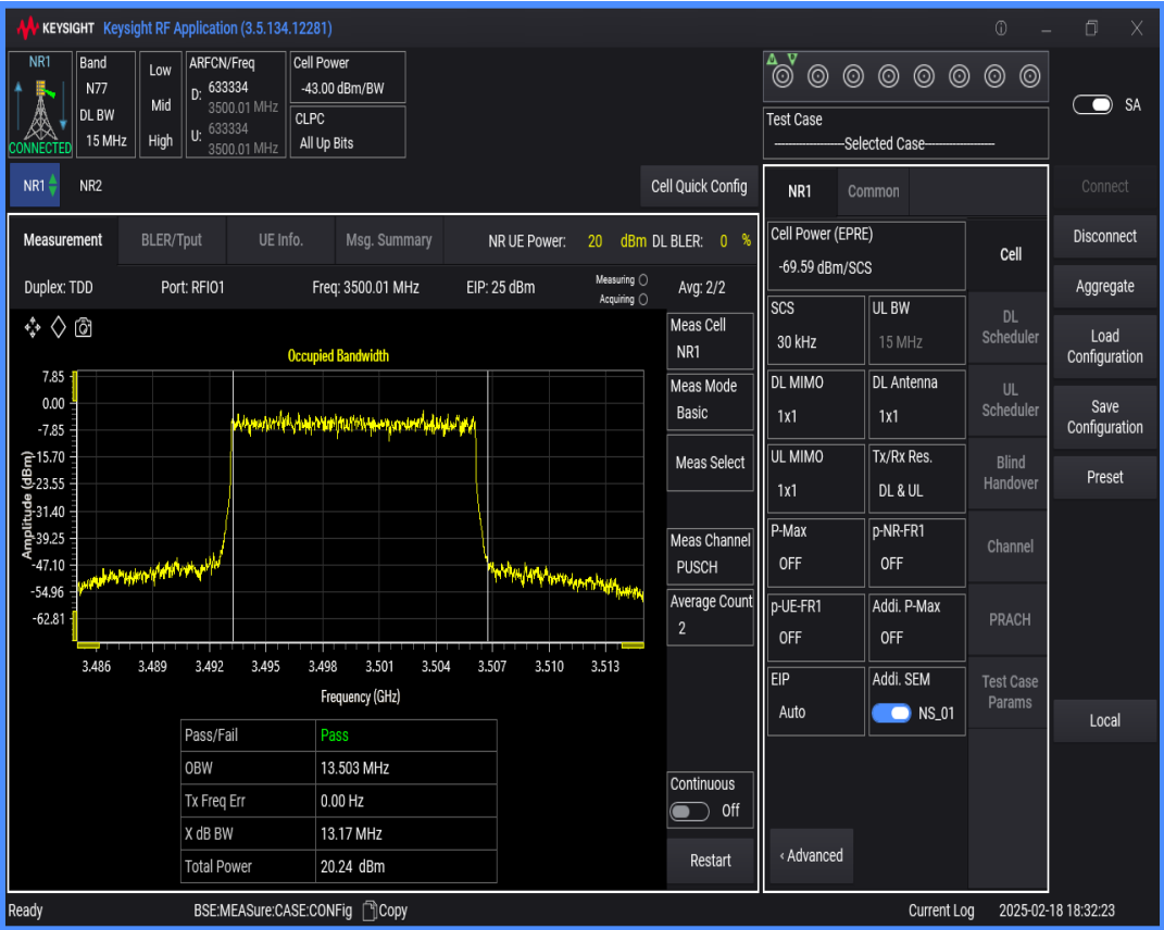
n77(3450-3550) SCS=30kHz DFT_QAM256 BW=10MHz Channel=633334 RB=24@0
