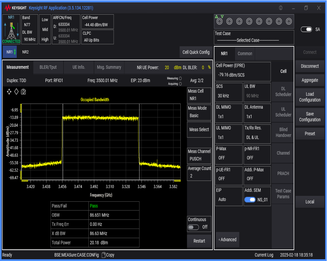
n77(3450-3550) SCS=30kHz DFT_QAM64 BW=15MHz Channel=633334 RB=36@0
