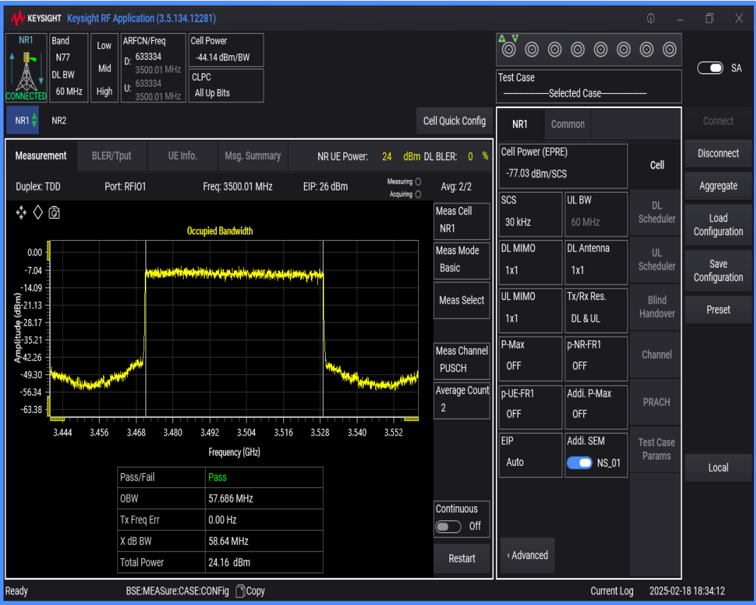
n77(3450-3550) SCS=30kHz DFT_BPSK BW=50MHz Channel=633334 RB=128@0
