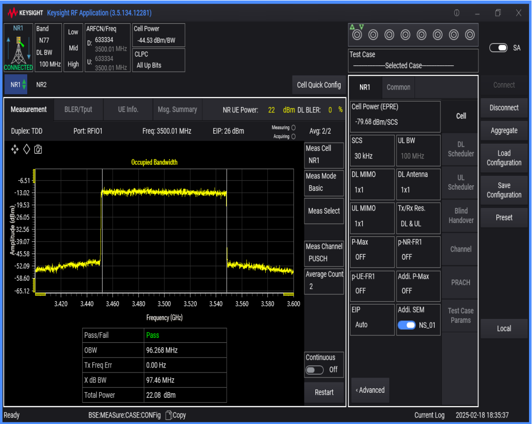
n77(3450-3550) SCS=30kHz DFT_QAM256 BW=90MHz Channel=633334 RB=240@0
