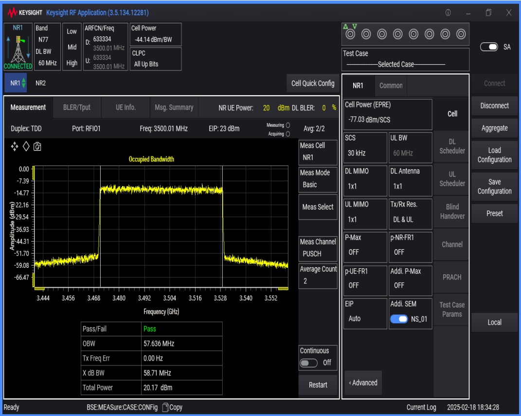
n77(3450-3550) SCS=30kHz DFT_QAM256 BW=50MHz Channel=633334 RB=128@0
