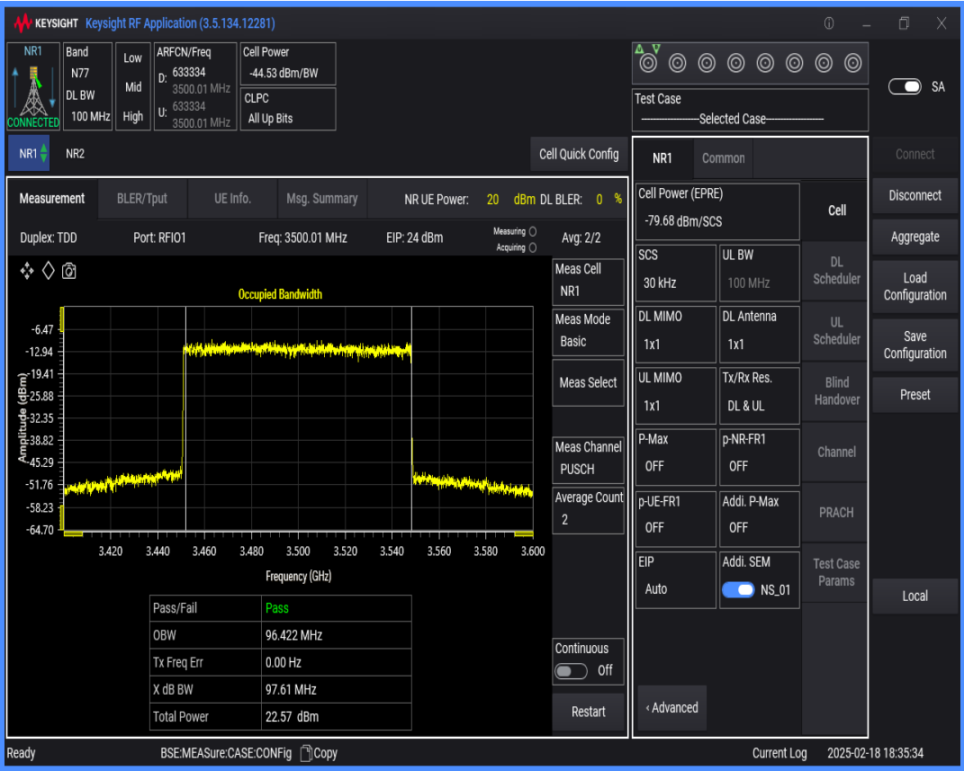
n77(3450-3550) SCS=30kHz DFT_QAM16 BW=30MHz Channel=633334 RB=75@0
