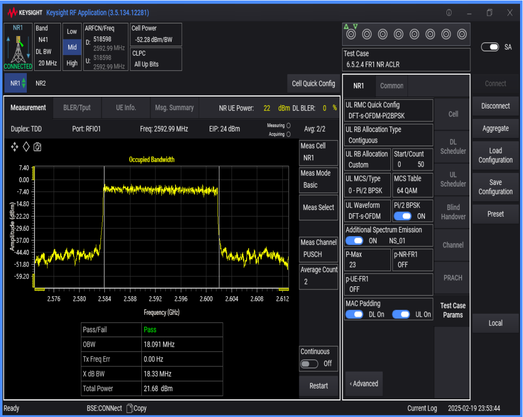
n41 SCS=30kHz DFT_BPSK BW=100MHz Channel=518598 RB=270@0
