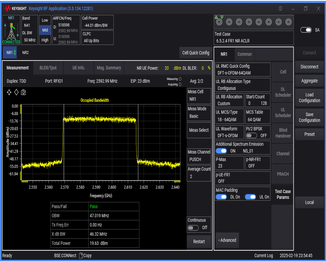
n41 SCS=30kHz DFT_QAM64 BW=40MHz Channel=518598 RB=100@0
