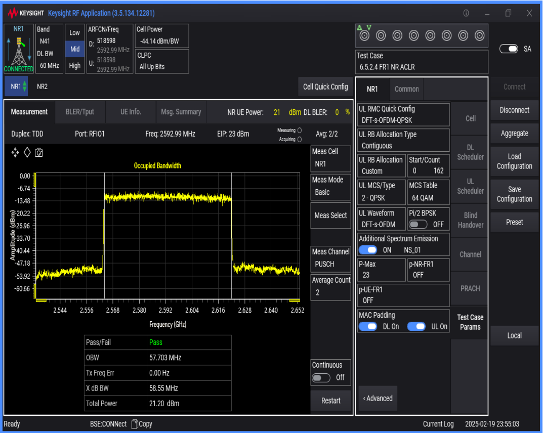
n41 SCS=30kHz DFT_QPSK BW=80MHz Channel=518598 RB=216@0
