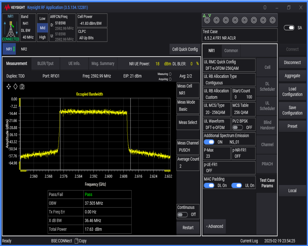
n41 SCS=30kHz DFT_QAM256 BW=60MHz Channel=518598 RB=162@0
