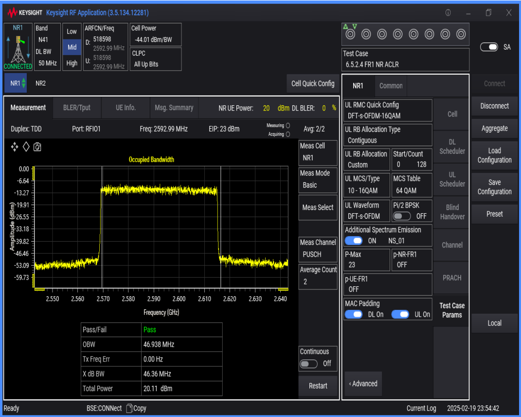
n41 SCS=30kHz DFT_QAM16 BW=60MHz Channel=518598 RB=162@0
