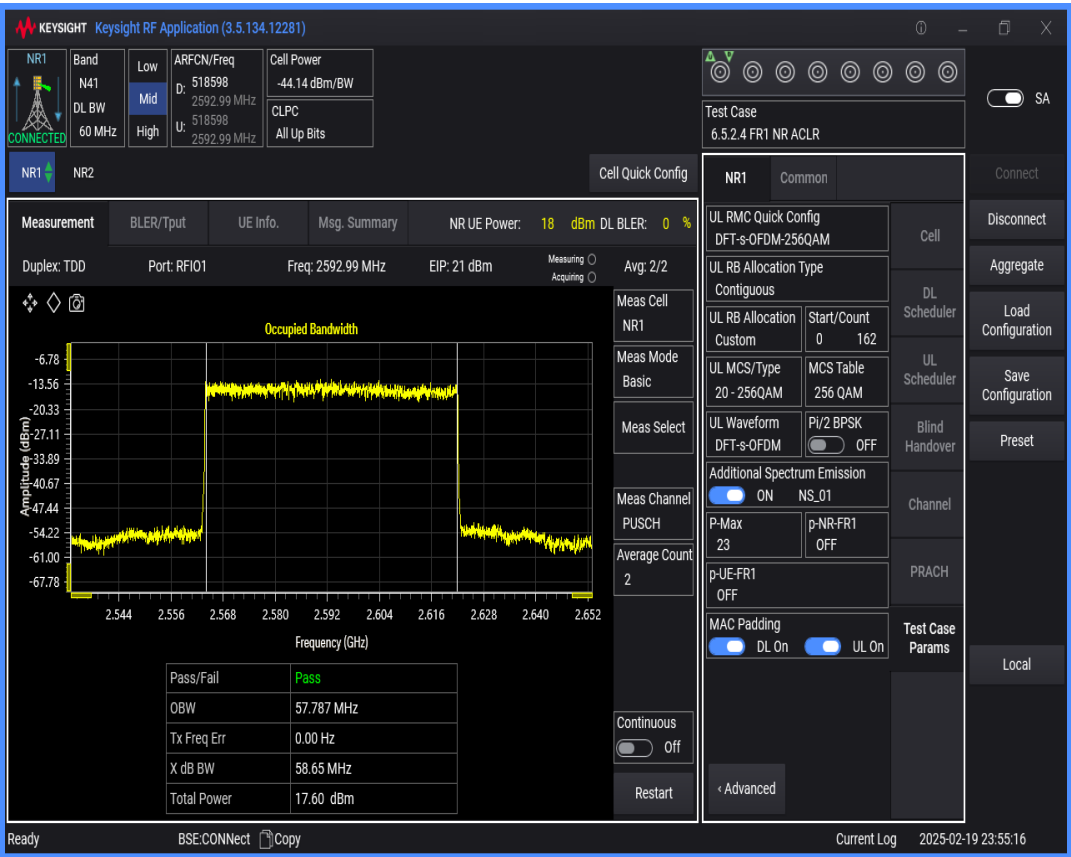
n41 SCS=30kHz DFT_QAM256 BW=50MHz Channel=518598 RB=128@0
