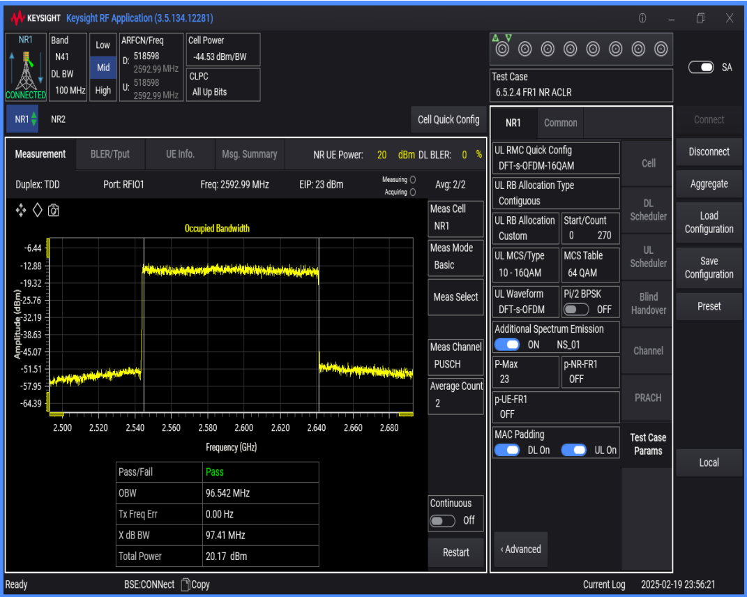
n41 SCS=30kHz DFT_QAM16 BW=40MHz Channel=518598 RB=100@0
