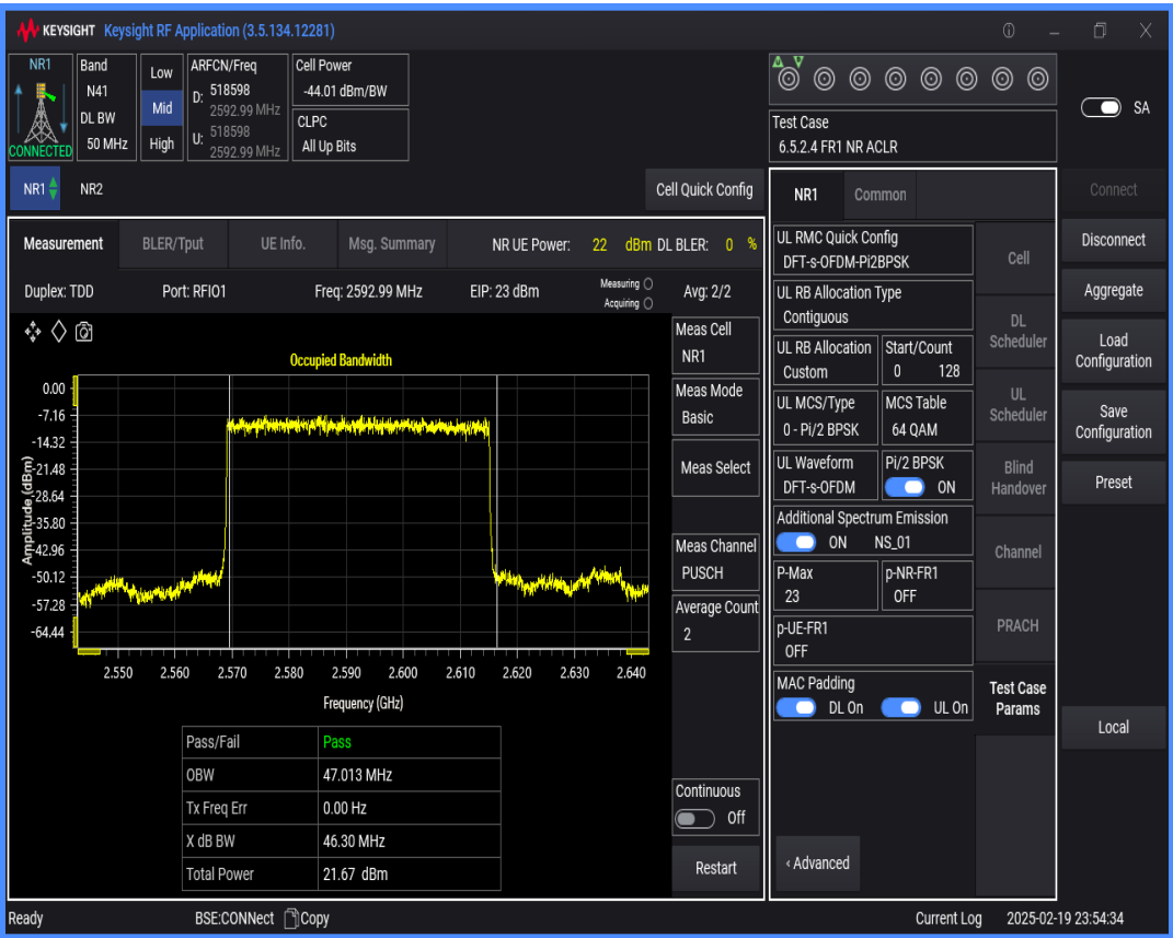
n41 SCS=30kHz DFT_BPSK BW=60MHz Channel=518598 RB=162@0
