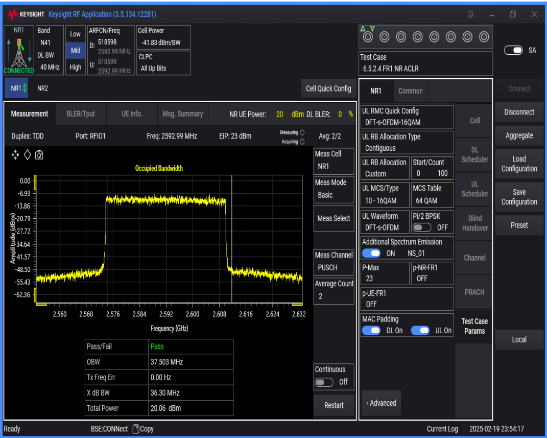
n41 SCS=30kHz DFT_QAM16 BW=50MHz Channel=518598 RB=128@0
