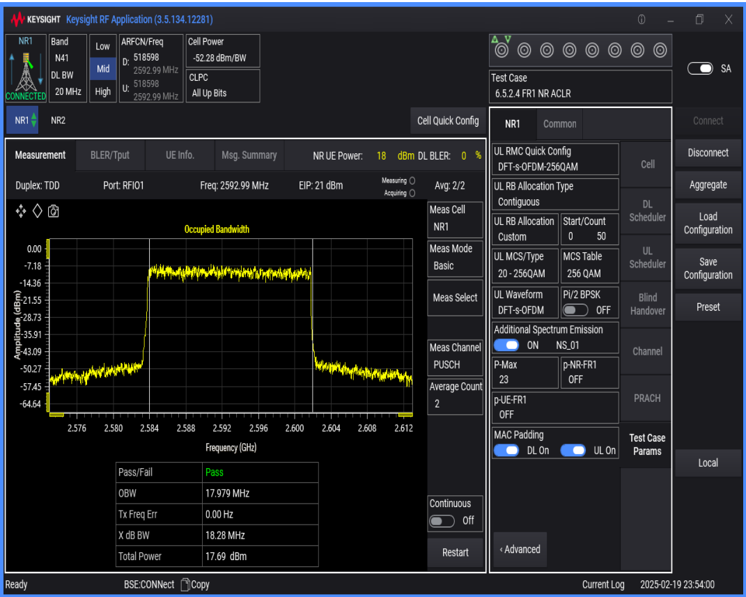
n41 SCS=30kHz DFT_QAM256 BW=40MHz Channel=518598 RB=100@0
