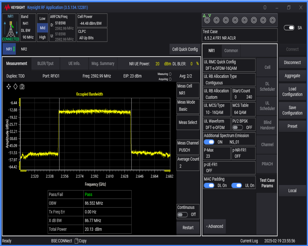
n41 SCS=30kHz DFT_QAM16 BW=80MHz Channel=518598 RB=216@0
