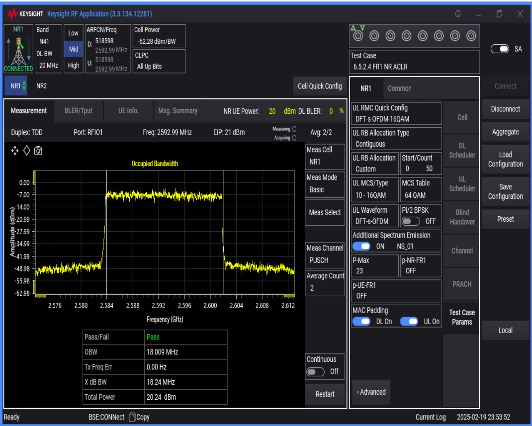
n41 SCS=30kHz DFT_QAM16 BW=100MHz Channel=518598 RB=270@0
