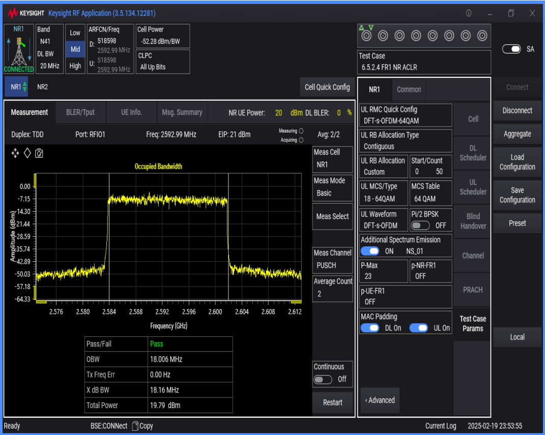
n41 SCS=30kHz DFT_QAM64 BW=50MHz Channel=518598 RB=128@0
