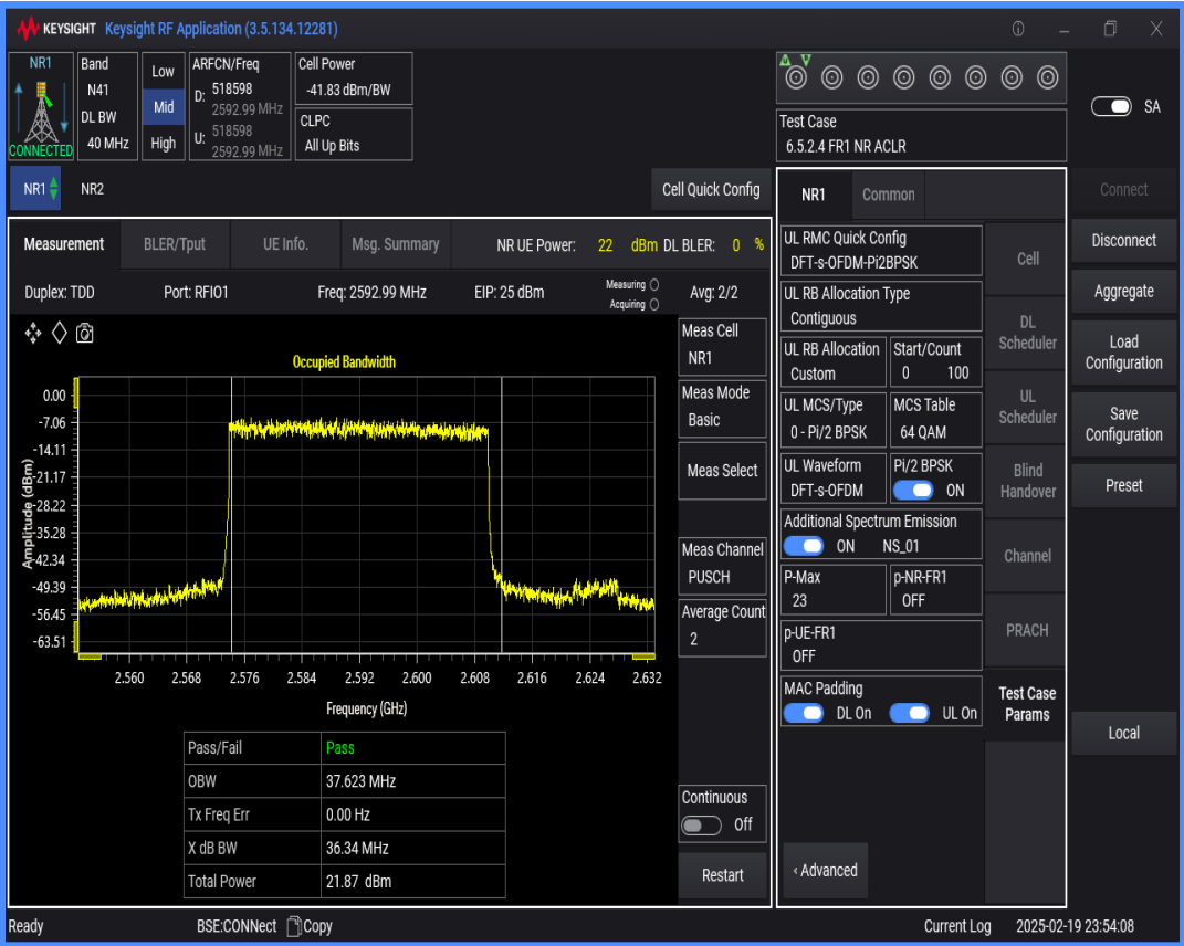
n41 SCS=30kHz DFT_BPSK BW=50MHz Channel=518598 RB=128@0
