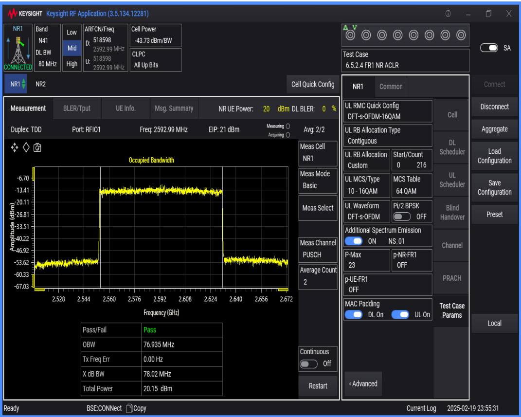
n41 SCS=30kHz DFT_QAM256 BW=100MHz Channel=518598 RB=270@0
