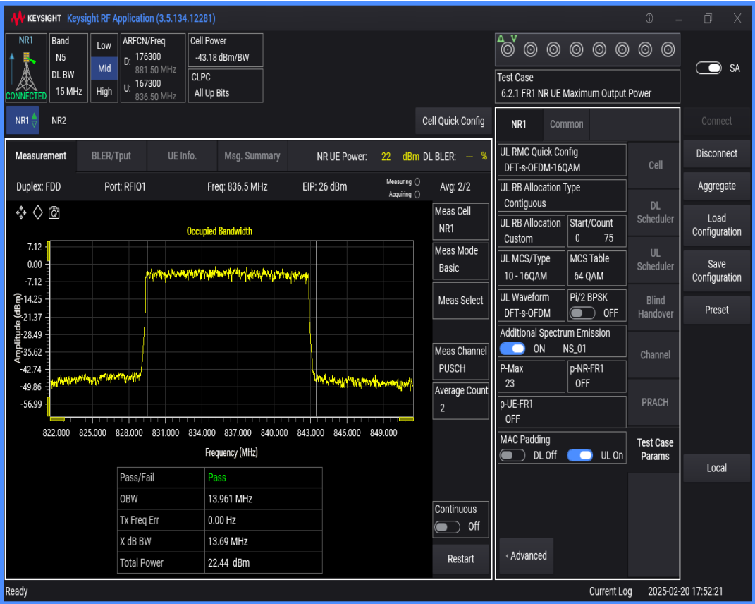
n5 SCS=15kHz DFT_QAM16 BW=5MHz Channel=167300 RB=25@0
