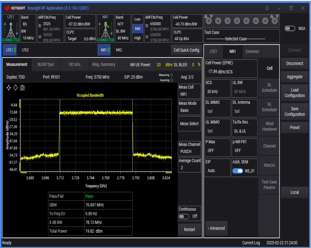
n77 SCS=30kHz DFT_QAM64 BW=60MHz Channel=650000 RB=162@0
