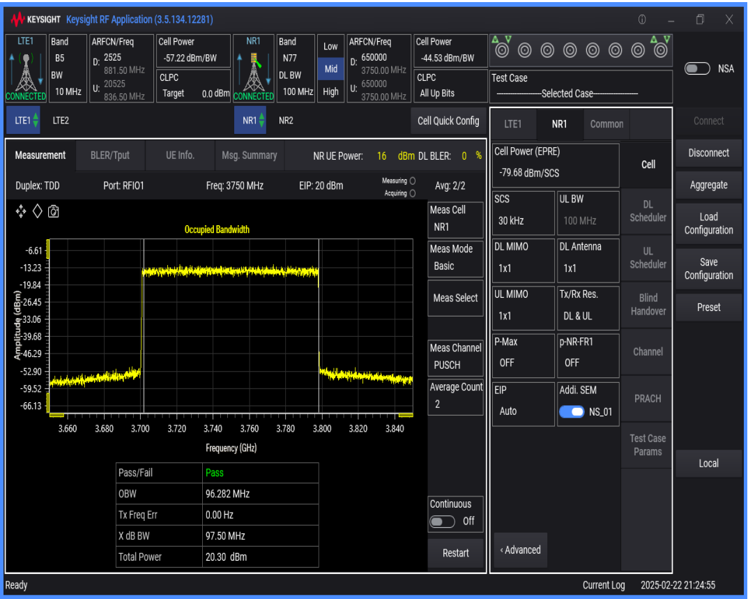
n77 SCS=30kHz DFT_BPSK BW=90MHz Channel=650000 RB=240@0
