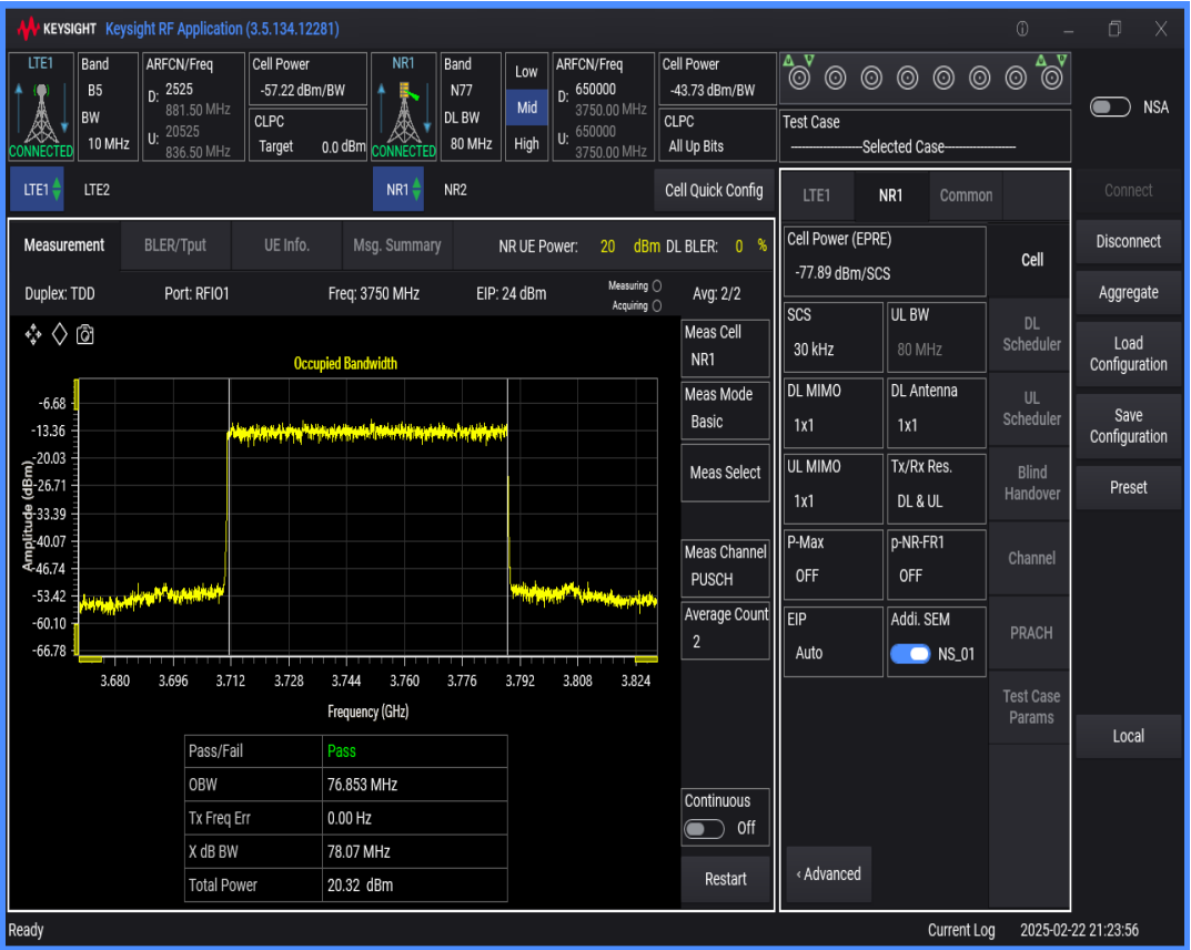
n77 SCS=30kHz DFT_QAM16 BW=60MHz Channel=650000 RB=162@0
