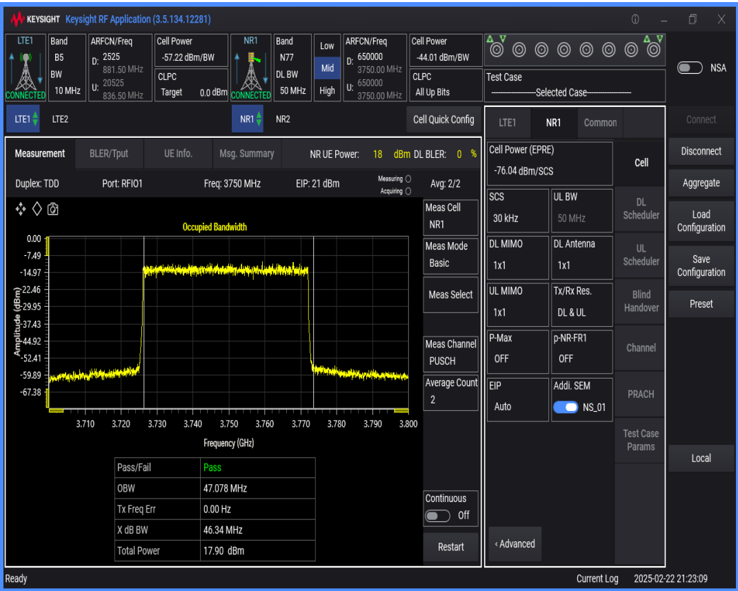
n77 SCS=30kHz DFT_QAM256 BW=80MHz Channel=650000 RB=216@0
