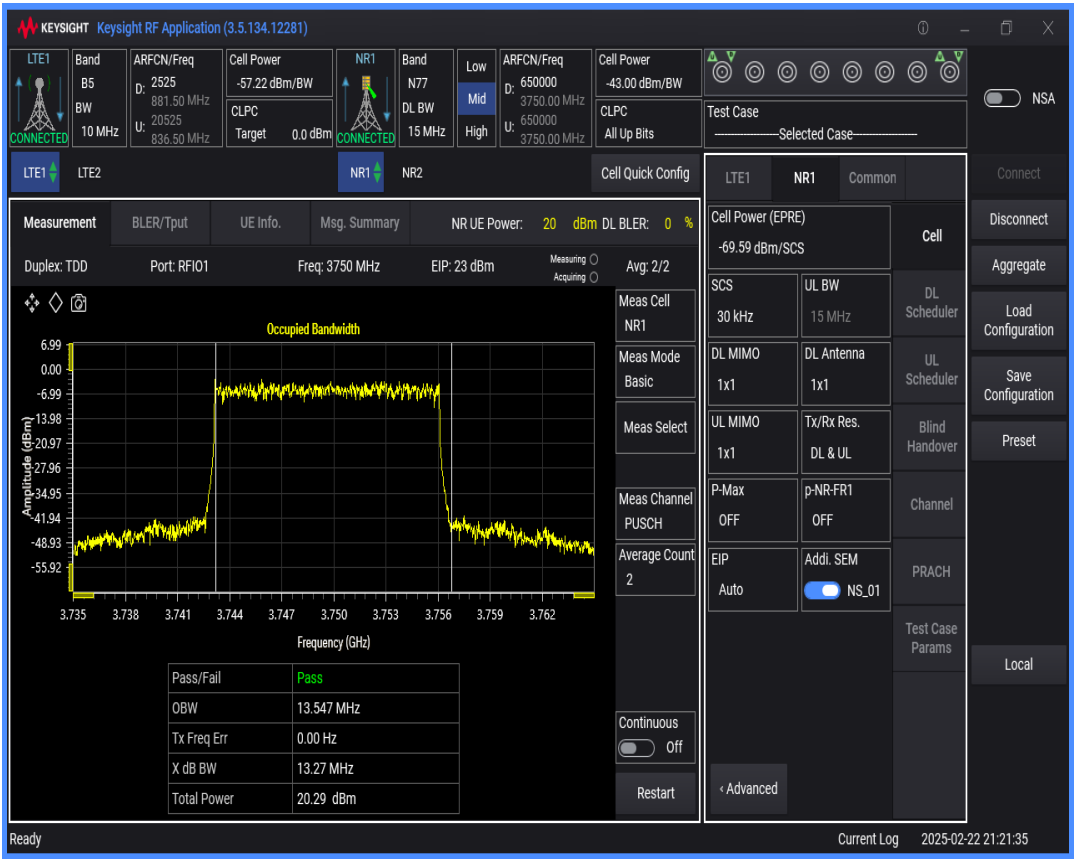
n77 SCS=30kHz DFT_QAM16 BW=10MHz Channel=650000 RB=24@0
