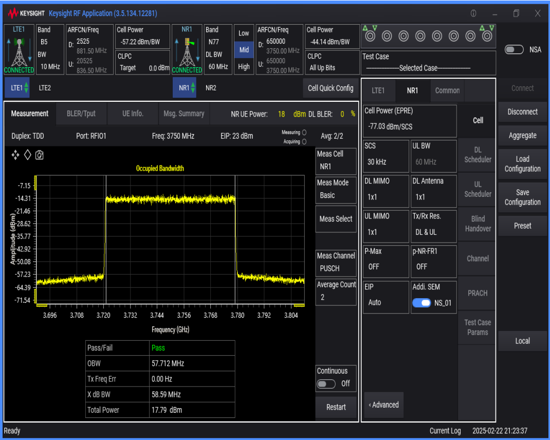
n77 SCS=30kHz DFT_QAM256 BW=50MHz Channel=650000 RB=128@0
