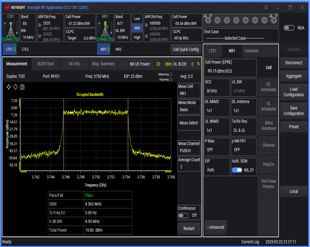
n77 SCS=30kHz DFT_QAM64 BW=100MHz Channel=650000 RB=270@0
