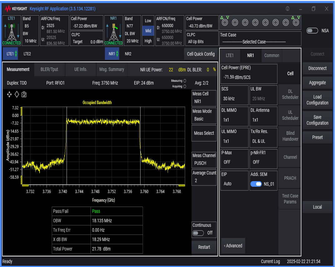
n77 SCS=30kHz DFT_QAM16 BW=100MHz Channel=650000 RB=270@0
