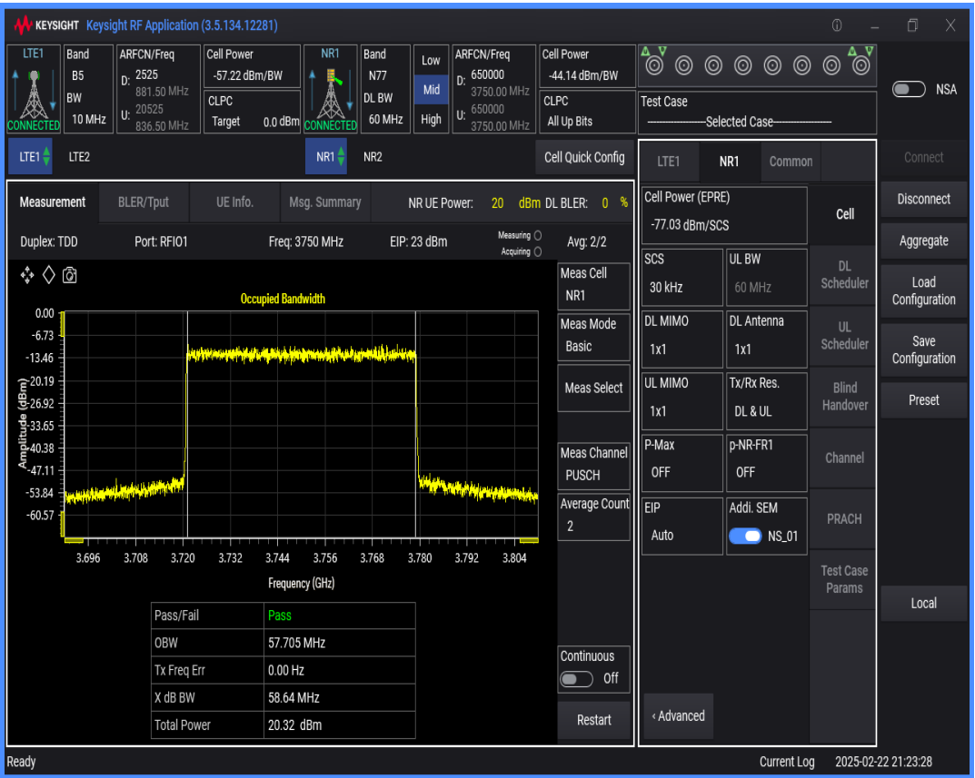
n77 SCS=30kHz DFT_QAM256 BW=100MHz Channel=650000 RB=270@0
