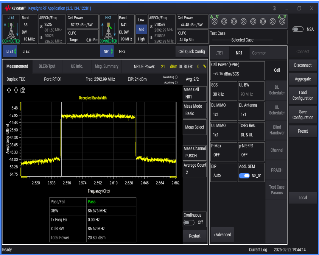
n41 SCS=30kHz DFT_QAM64 BW=80MHz Channel=518598 RB=216@0
