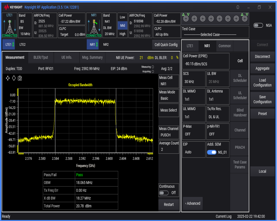
n41 SCS=30kHz DFT_QAM64 BW=50MHz Channel=518598 RB=128@0
