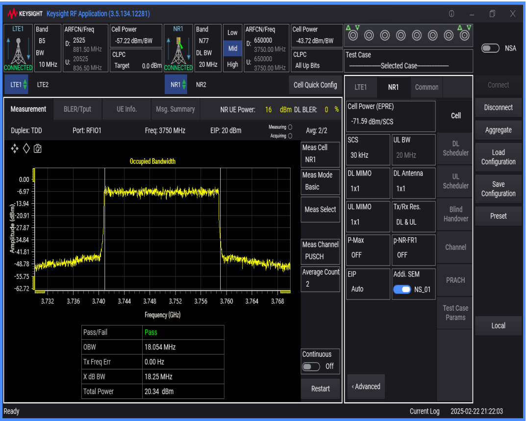
n77 SCS=30kHz DFT_QAM16 BW=80MHz Channel=650000 RB=216@0
