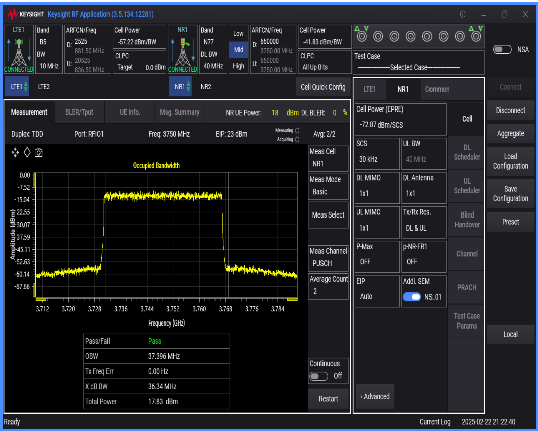
n77 SCS=30kHz DFT_QAM256 BW=80MHz Channel=650000 RB=216@0
