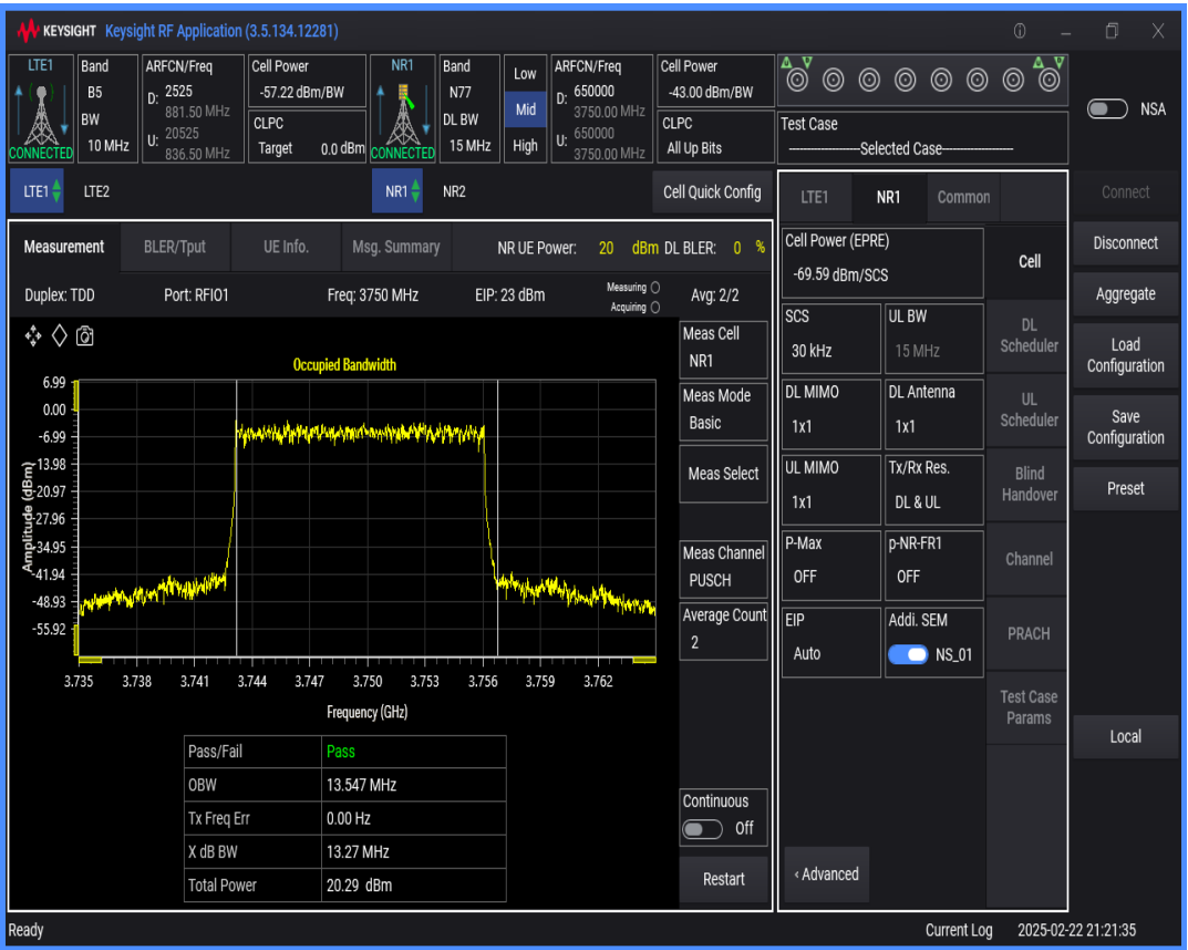
n77 SCS=30kHz DFT_QAM16 BW=20MHz Channel=650000 RB=50@0
