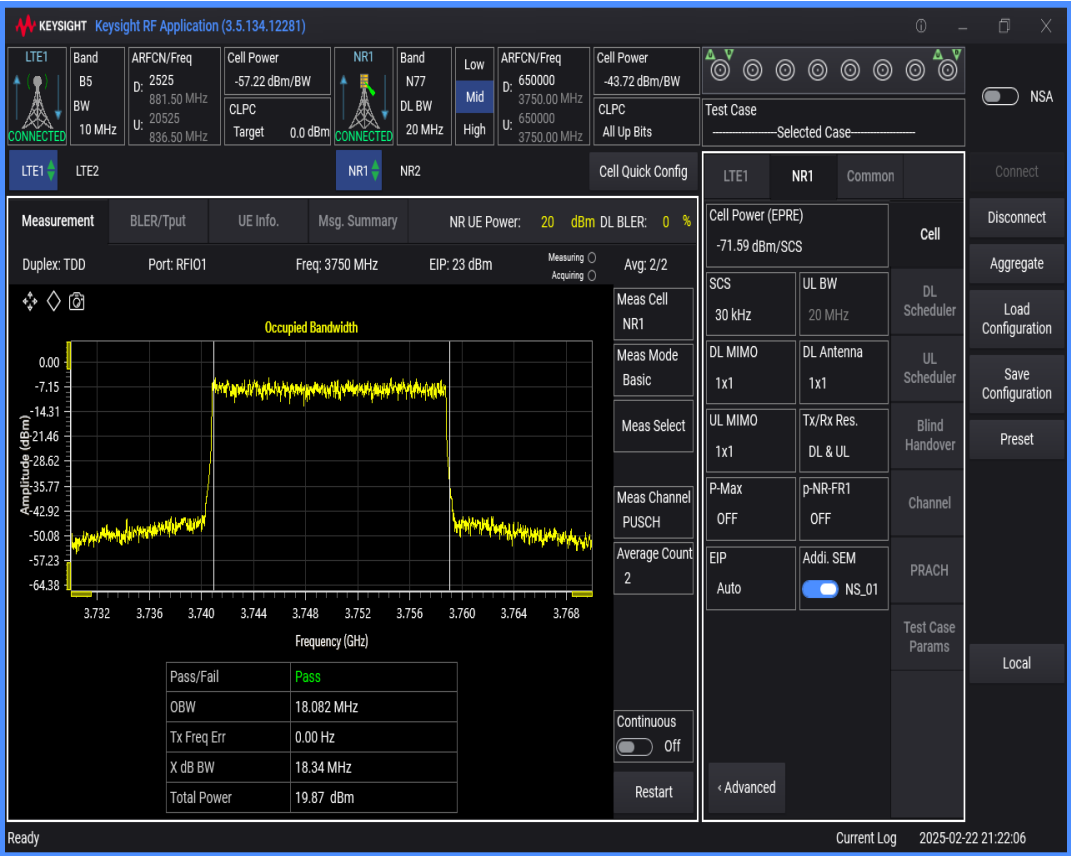
n77 SCS=30kHz DFT_QAM64 BW=15MHz Channel=650000 RB=36@0
