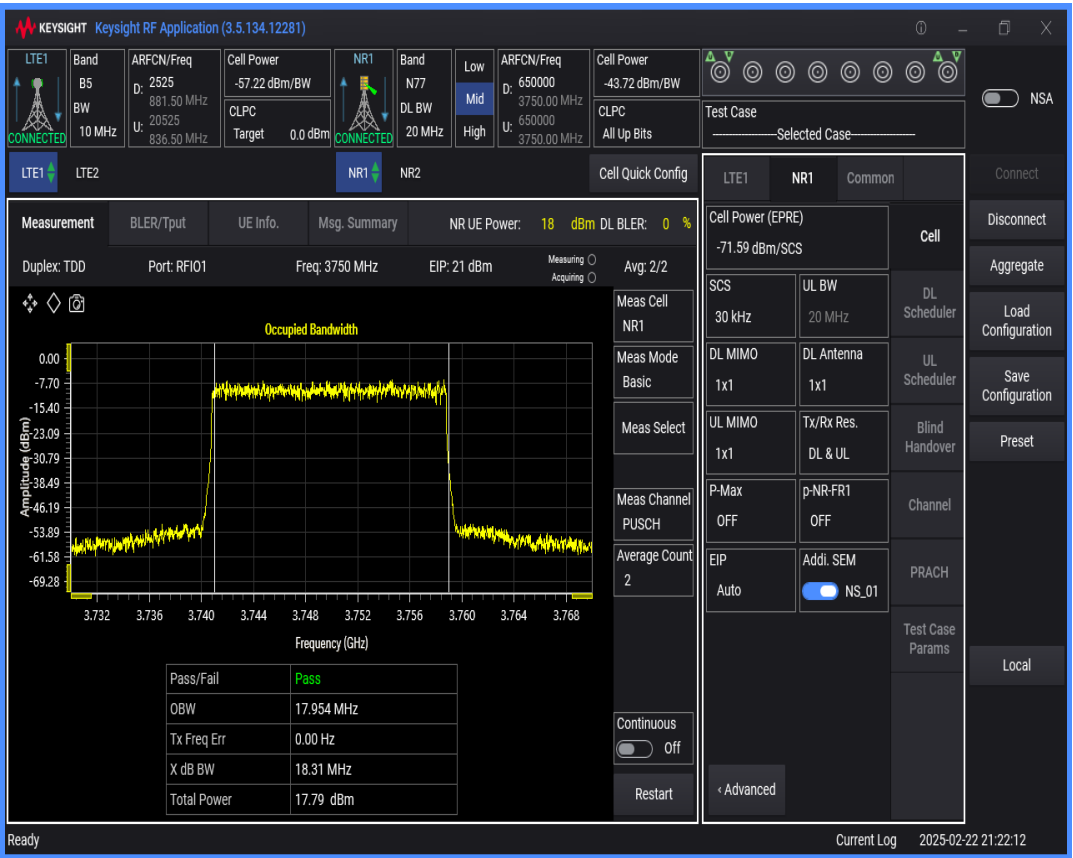
n77 SCS=30kHz DFT_QAM256 BW=50MHz Channel=650000 RB=128@0
