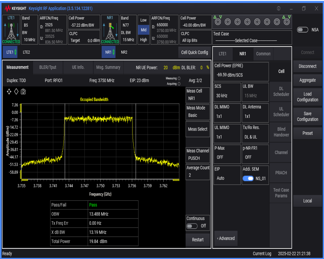
n77 SCS=30kHz DFT_QAM64 BW=50MHz Channel=650000 RB=128@0
