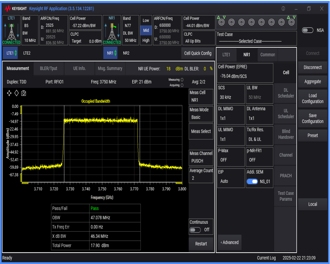
n77 SCS=30kHz DFT_QAM256 BW=40MHz Channel=650000 RB=100@0
