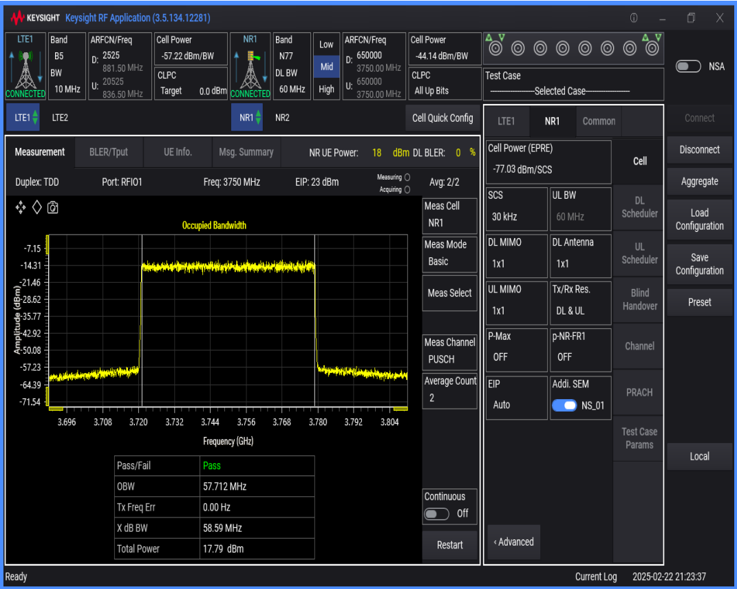
n77 SCS=30kHz DFT_QAM64 BW=100MHz Channel=650000 RB=270@0
