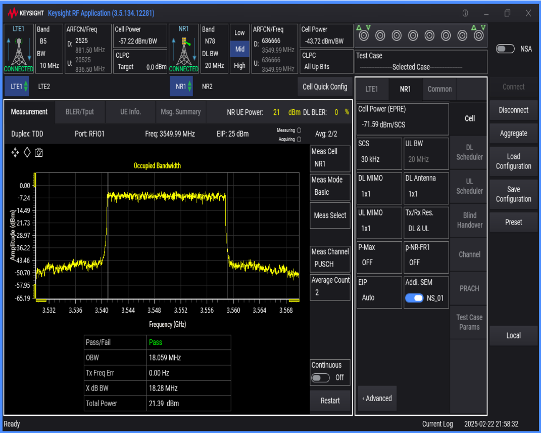
n78 SCS=30kHz DFT_QPSK BW=40MHz Channel=636666 RB=100@0
