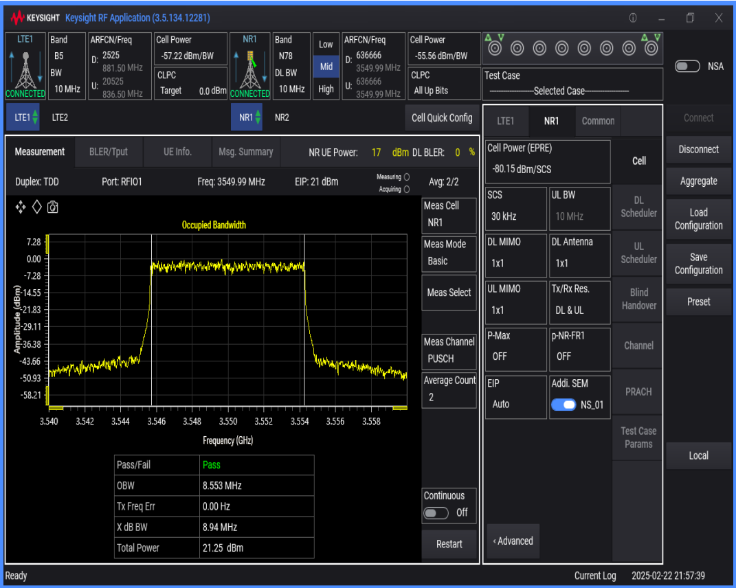
n78 SCS=30kHz DFT_QPSK BW=90MHz Channel=636666 RB=240@0
