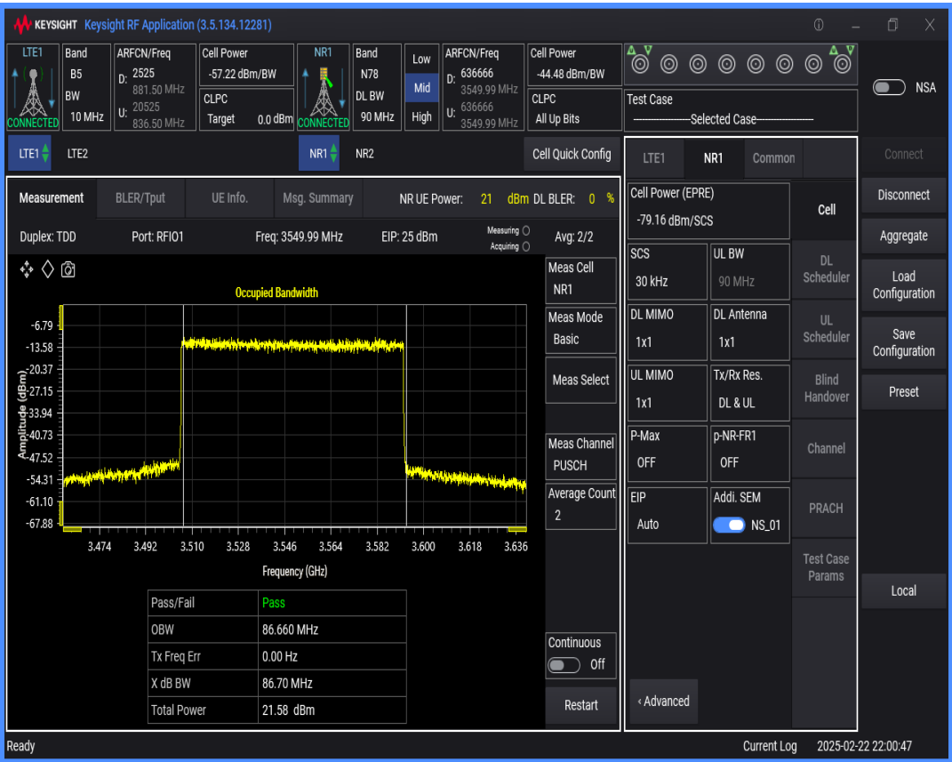
n78 SCS=30kHz DFT_QPSK BW=80MHz Channel=636666 RB=216@0
