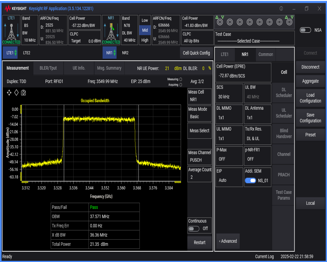
n78 SCS=30kHz DFT_QPSK BW=50MHz Channel=636666 RB=128@0
