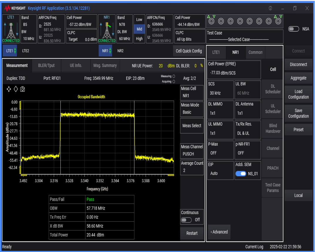
n78 SCS=30kHz DFT_QAM16 BW=80MHz Channel=636666 RB=216@0
