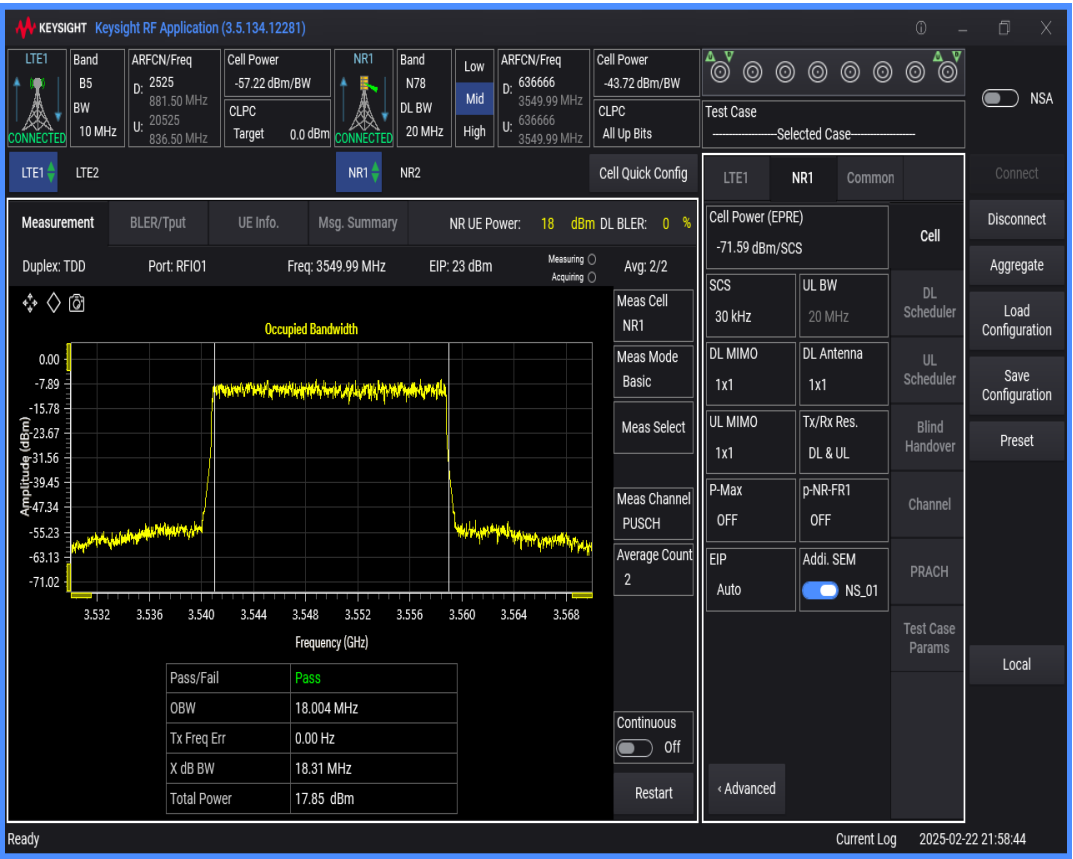
n78 SCS=30kHz DFT_QAM256 BW=40MHz Channel=636666 RB=100@0
