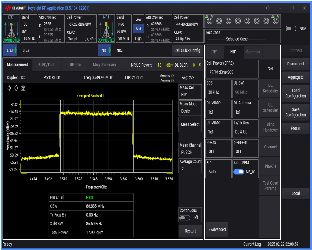
n78 SCS=30kHz DFT_QAM64 BW=15MHz Channel=636666 RB=36@0
