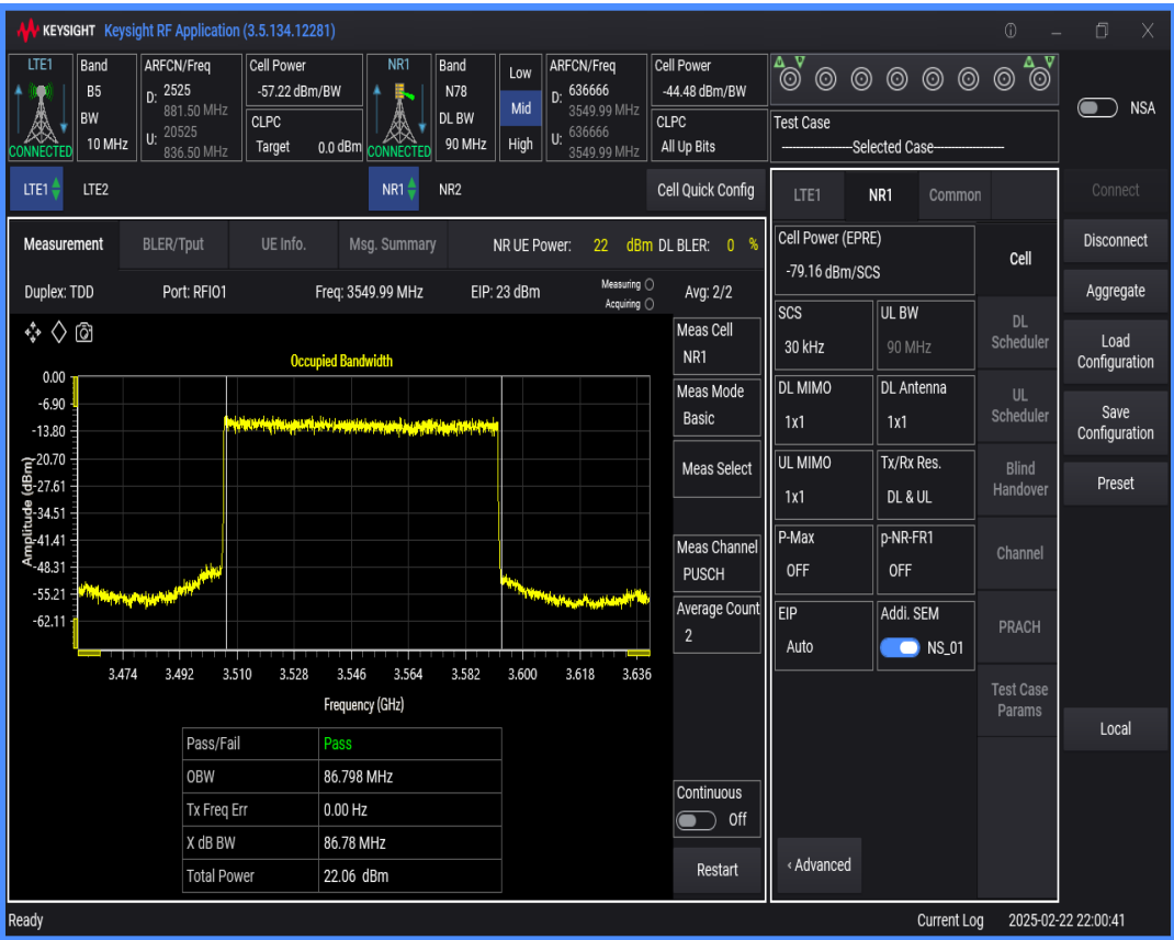
n78 SCS=30kHz DFT_BPSK BW=50MHz Channel=636666 RB=128@0
