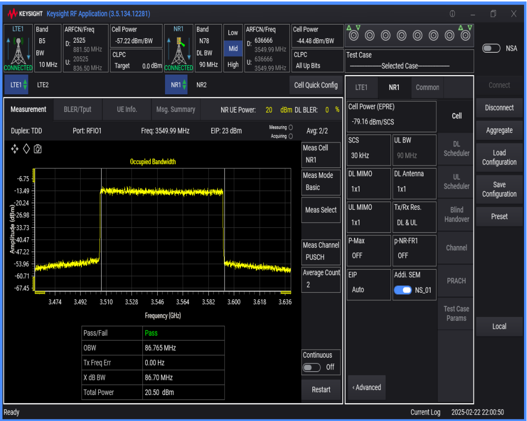
n78 SCS=30kHz DFT_QAM256 BW=100MHz Channel=636666 RB=270@0
