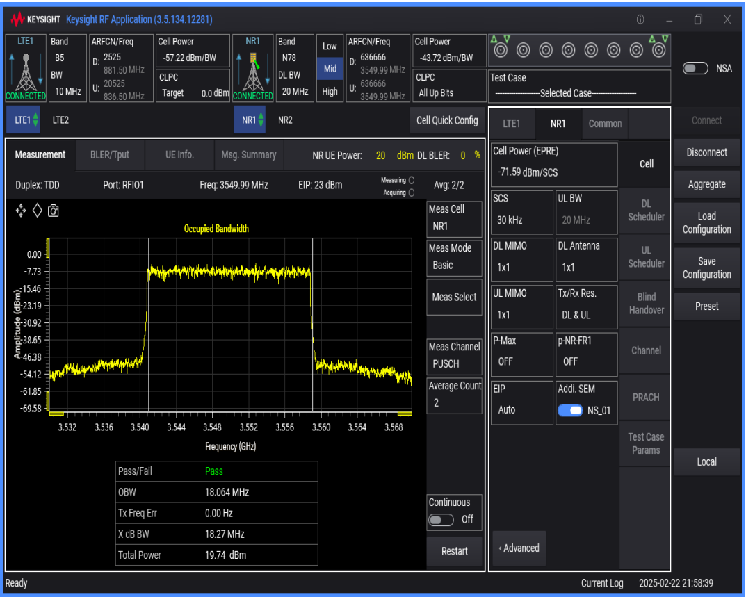
n78 SCS=30kHz DFT_QAM64 BW=100MHz Channel=636666 RB=270@0
