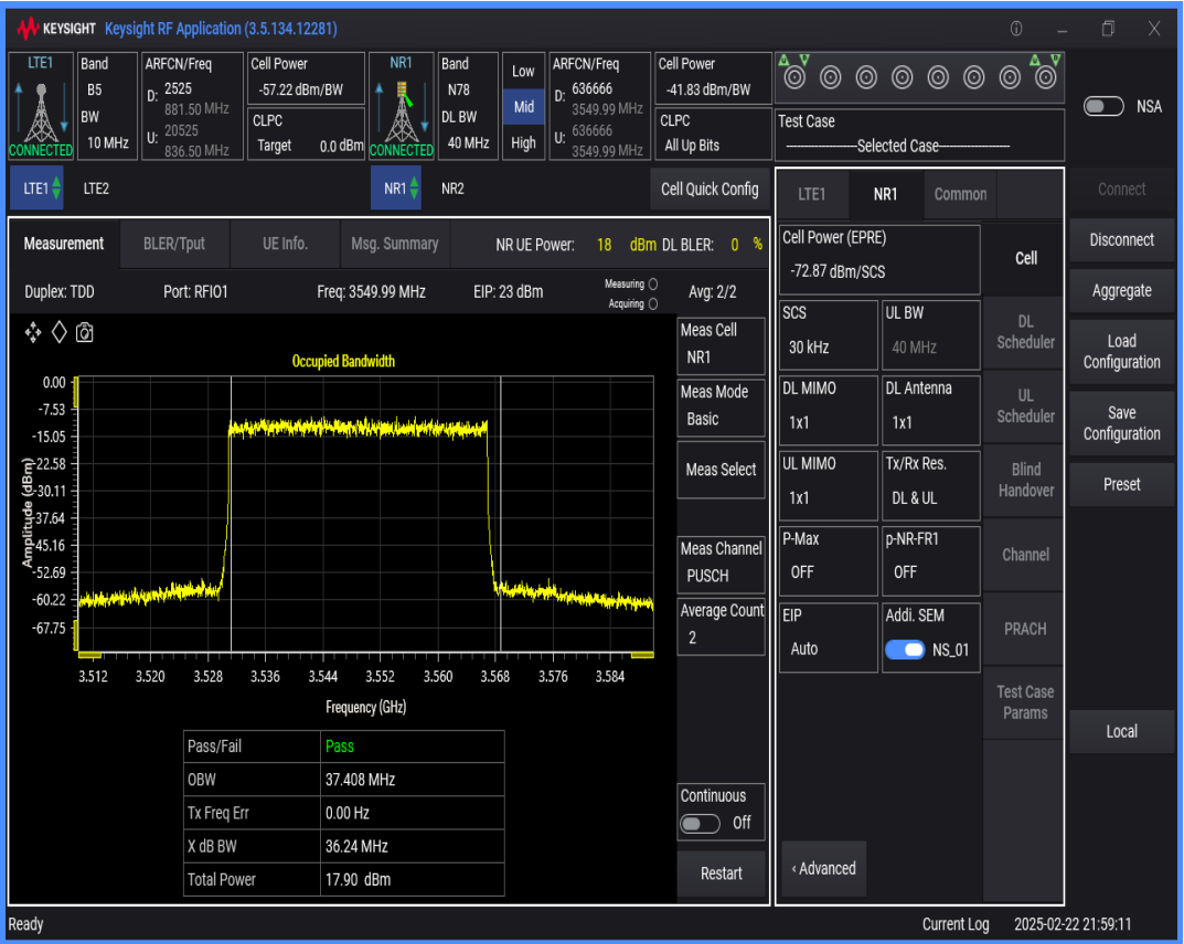
n78 SCS=30kHz DFT_QAM64 BW=50MHz Channel=636666 RB=128@0
