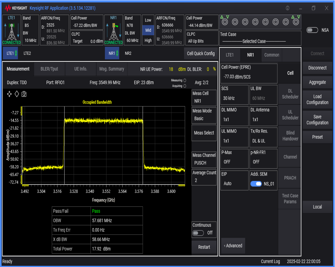
n78 SCS=30kHz DFT_QAM256 BW=80MHz Channel=636666 RB=216@0
