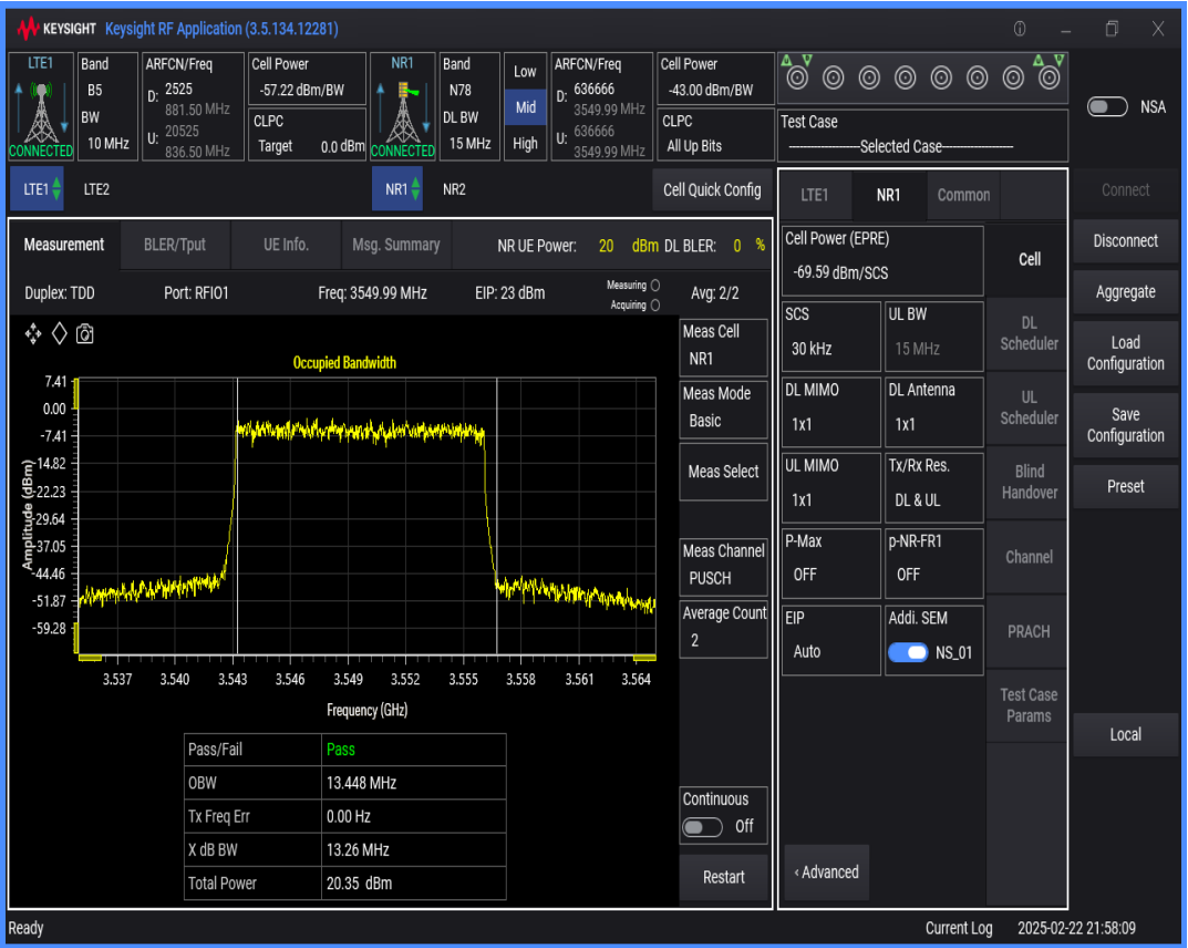
n78 SCS=30kHz DFT_QAM16 BW=90MHz Channel=636666 RB=240@0
