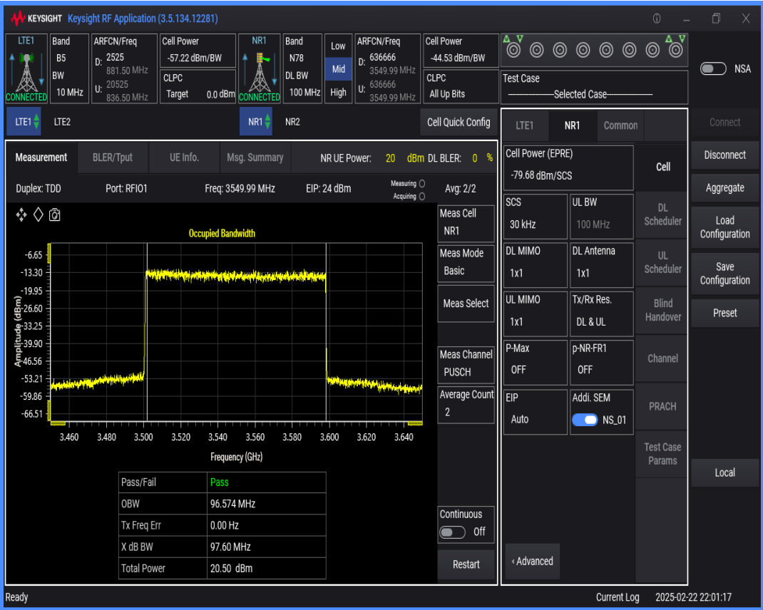
n78 SCS=30kHz DFT_BPSK BW=90MHz Channel=636666 RB=240@0
