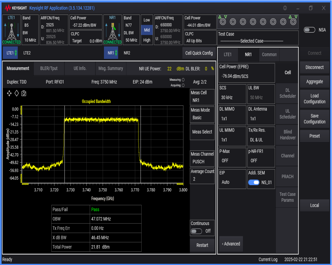
n77 SCS=30kHz DFT_QAM16 BW=10MHz Channel=650000 RB=24@0
