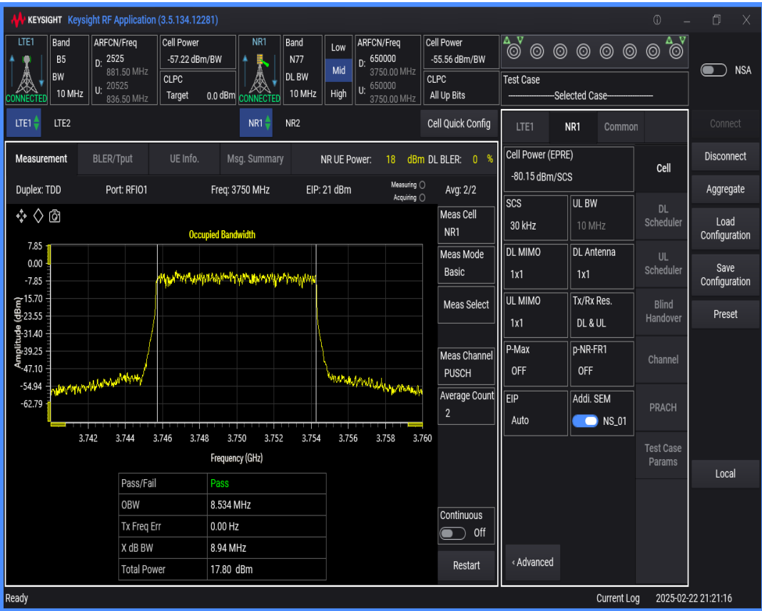
n77 SCS=30kHz DFT_QAM256 BW=100MHz Channel=650000 RB=270@0
