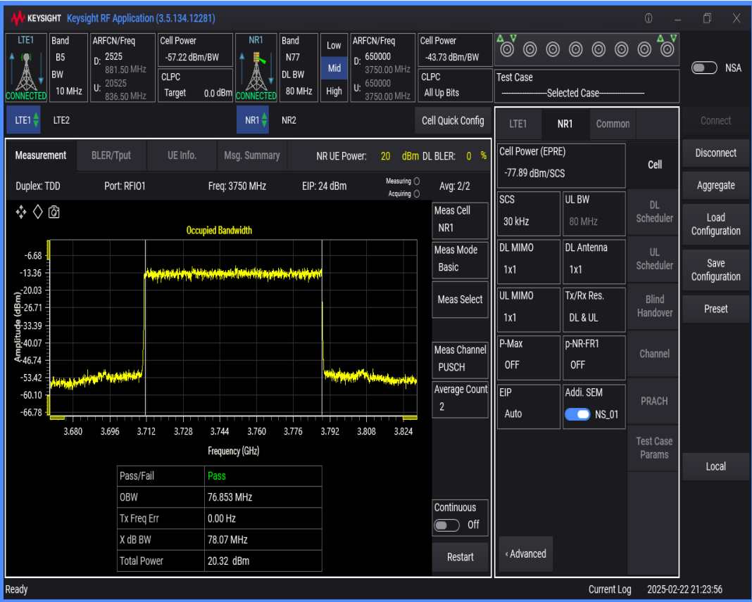
n77 SCS=30kHz DFT_QAM256 BW=10MHz Channel=650000 RB=24@0
