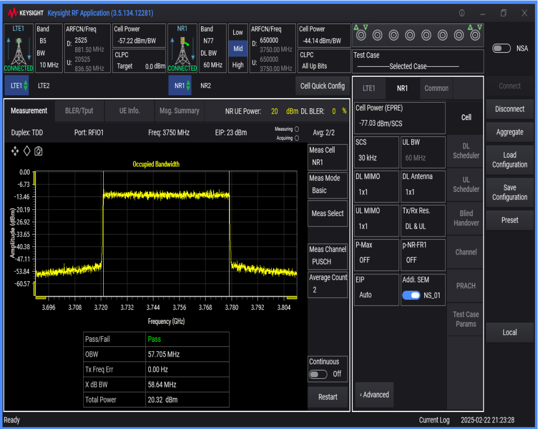
n77 SCS=30kHz DFT_QAM16 BW=90MHz Channel=650000 RB=240@0
