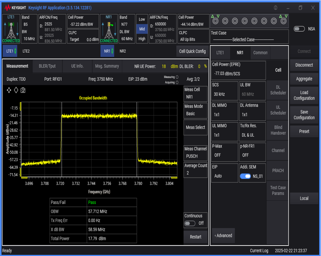
n77 SCS=30kHz DFT_QAM64 BW=100MHz Channel=650000 RB=270@0
