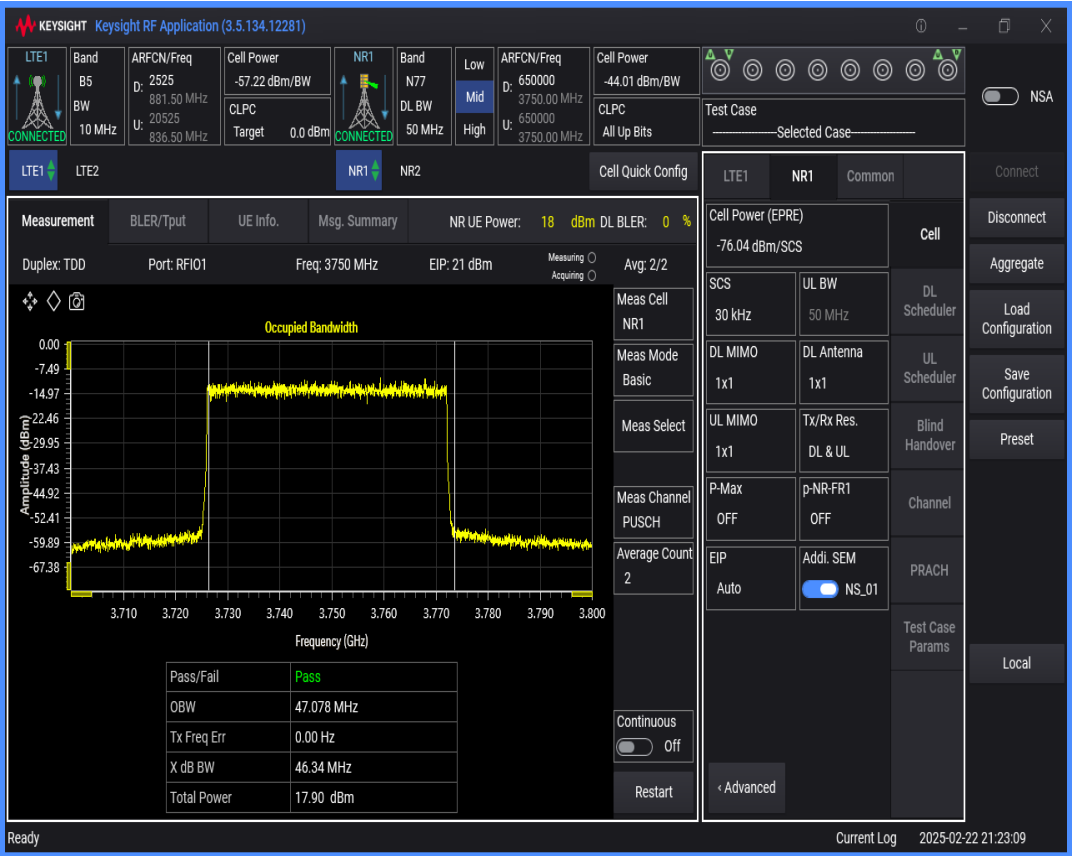
n77 SCS=30kHz DFT_QAM256 BW=80MHz Channel=650000 RB=216@0
