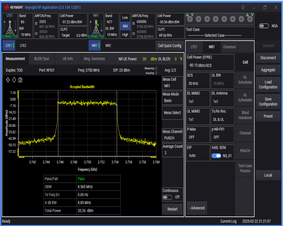
n77 SCS=30kHz DFT_QAM16 BW=20MHz Channel=650000 RB=50@0
