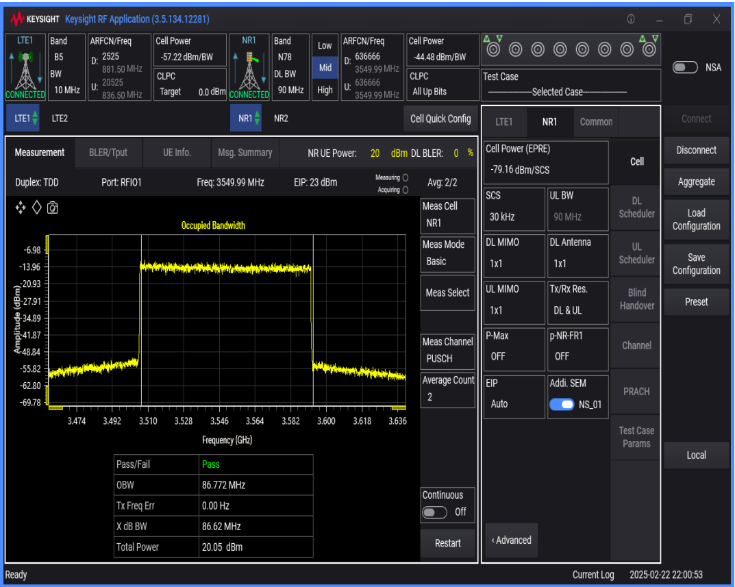
n78 SCS=30kHz DFT_QAM64 BW=80MHz Channel=636666 RB=216@0
