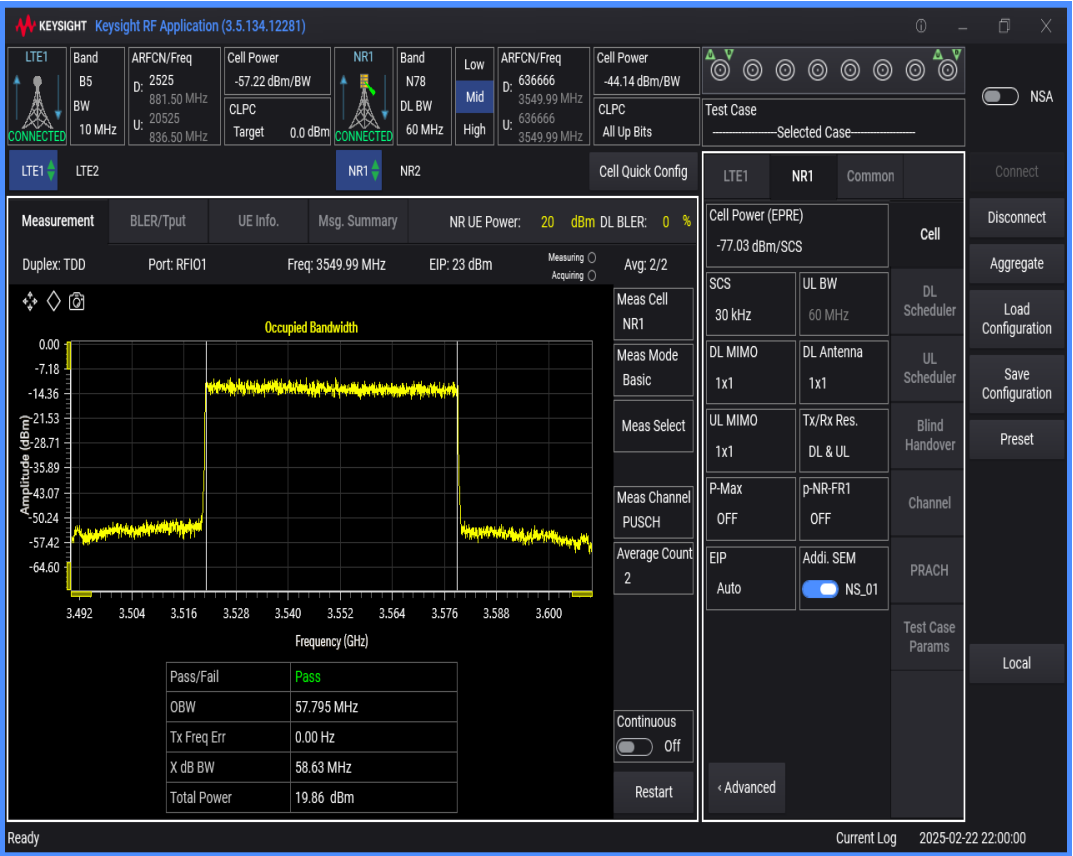
n78 SCS=30kHz DFT_QAM64 BW=90MHz Channel=636666 RB=240@0
