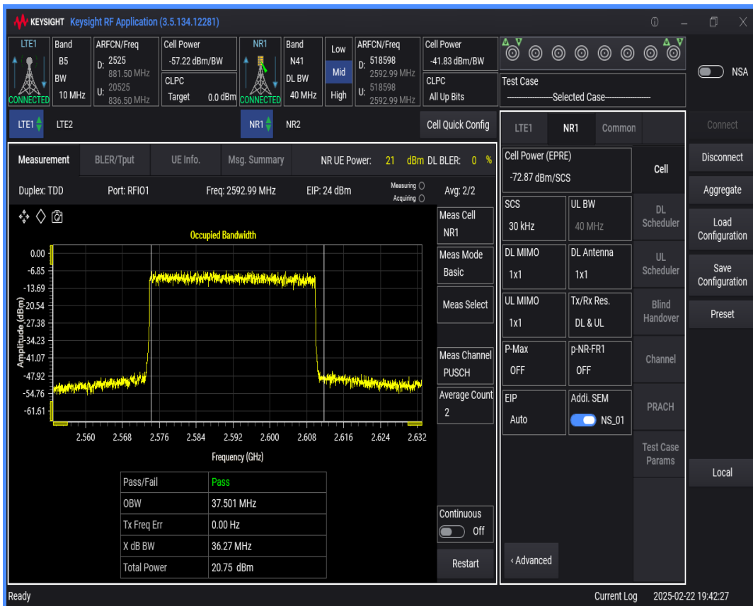
n41 SCS=30kHz DFT_QAM64 BW=80MHz Channel=518598 RB=216@0
