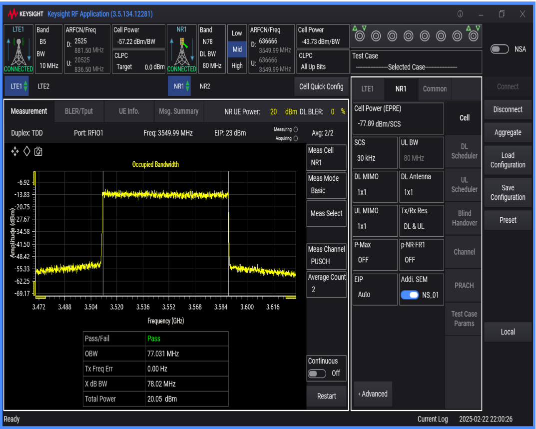
n78 SCS=30kHz DFT_QAM64 BW=90MHz Channel=636666 RB=240@0
