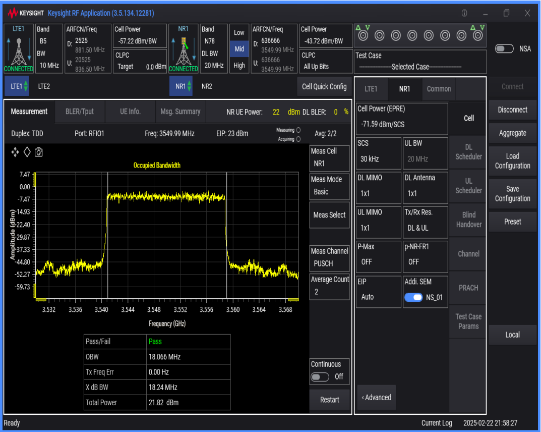
n78 SCS=30kHz DFT_BPSK BW=50MHz Channel=636666 RB=128@0
