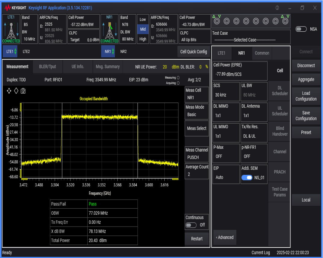
n78 SCS=30kHz DFT_QAM16 BW=60MHz Channel=636666 RB=162@0
