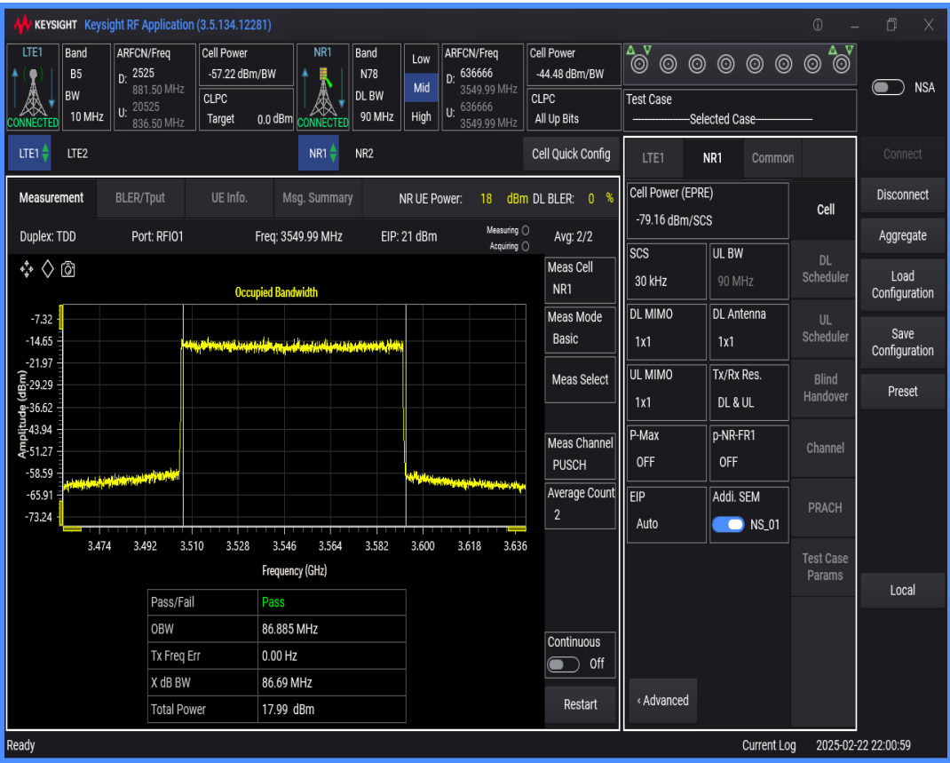
n78 SCS=30kHz DFT_QAM64 BW=10MHz Channel=636666 RB=24@0
