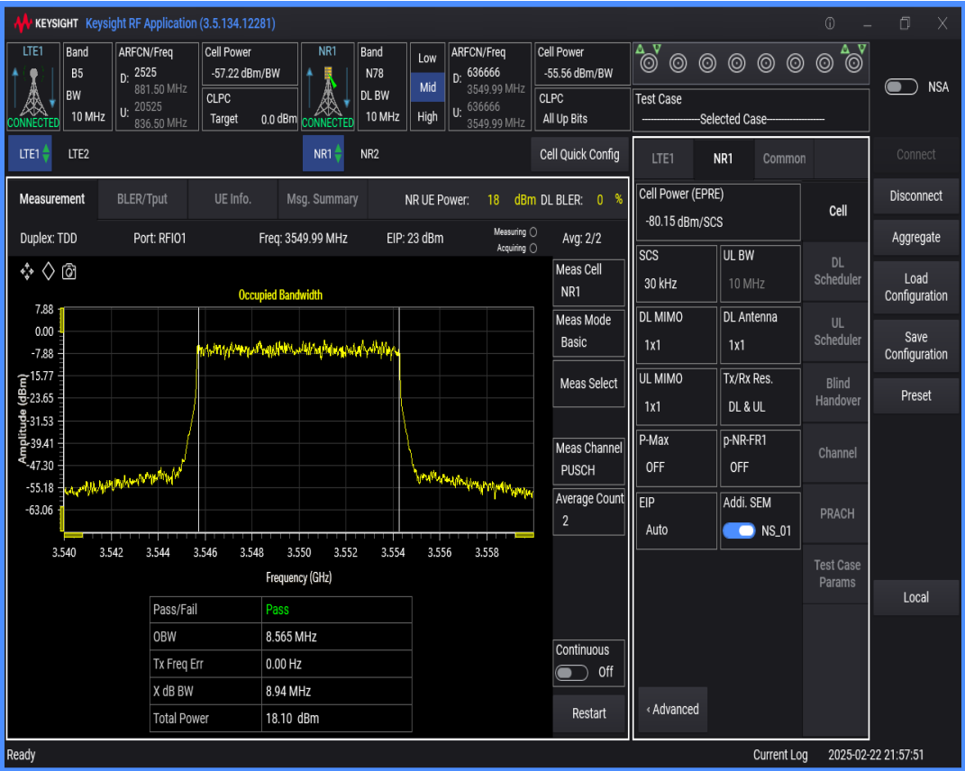
n78 SCS=30kHz DFT_QAM256 BW=15MHz Channel=636666 RB=36@0
