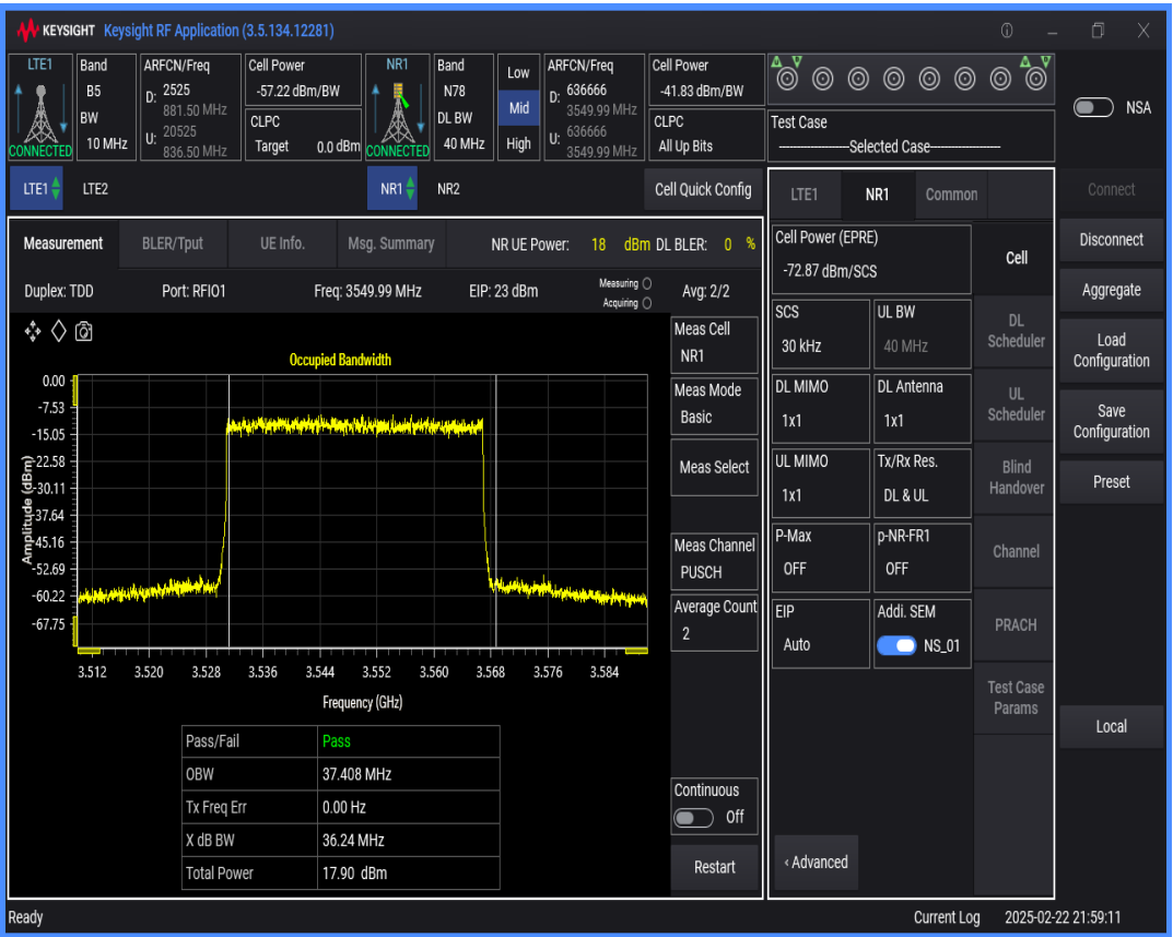
n78 SCS=30kHz DFT_QAM256 BW=50MHz Channel=636666 RB=128@0
