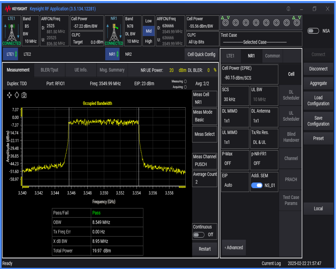
n78 SCS=30kHz DFT_QAM64 BW=100MHz Channel=636666 RB=270@0
