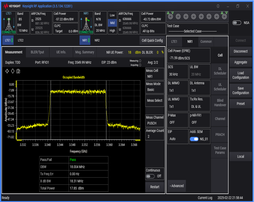
n78 SCS=30kHz DFT_QAM256 BW=40MHz Channel=636666 RB=100@0
