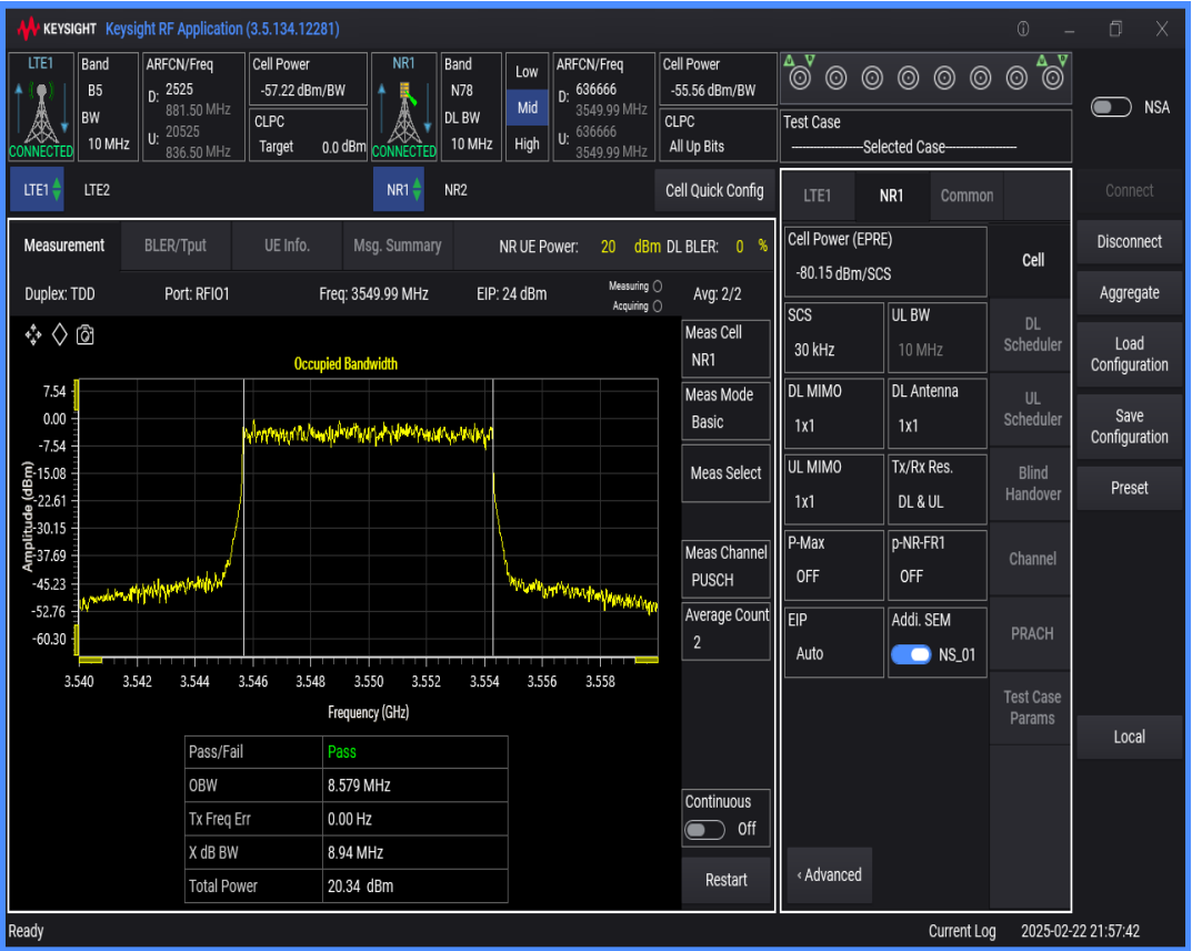
n78 SCS=30kHz DFT_QAM16 BW=100MHz Channel=636666 RB=270@0
