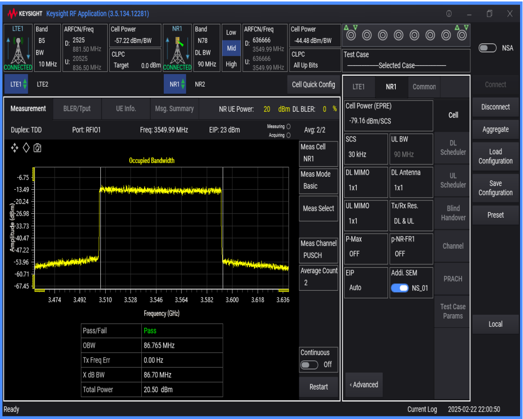
n78 SCS=30kHz DFT_QAM256 BW=10MHz Channel=636666 RB=24@0
