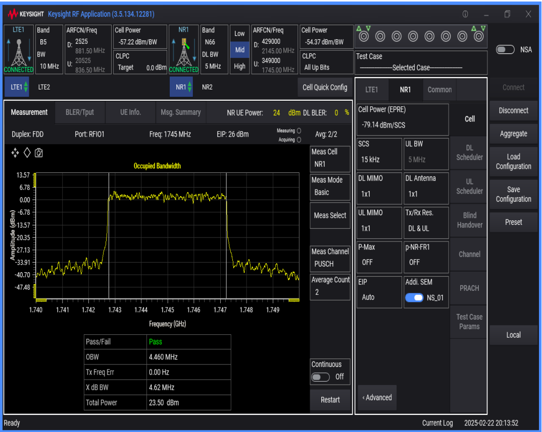
n66 SCS=15kHz DFT_BPSK BW=40MHz Channel=349000 RB=216@0
