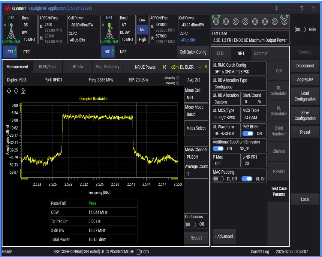
n7 SCS=15kHz DFT_BPSK BW=5MHz Channel=507000 RB=25@0
