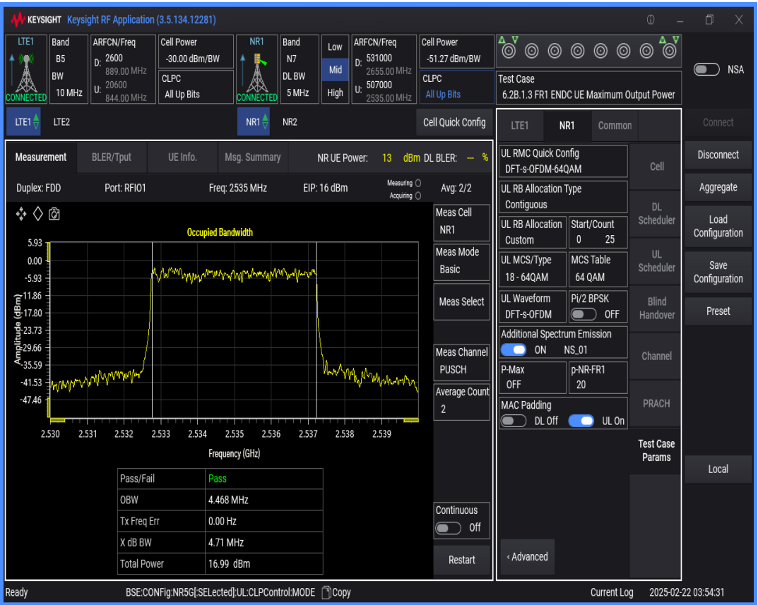
n7 SCS=15kHz DFT_QAM64 BW=20MHz Channel=507000 RB=100@0
