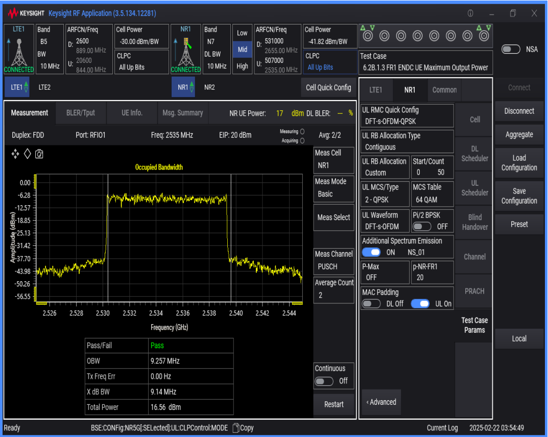
n7 SCS=15kHz DFT_QAM64 BW=5MHz Channel=507000 RB=25@0
