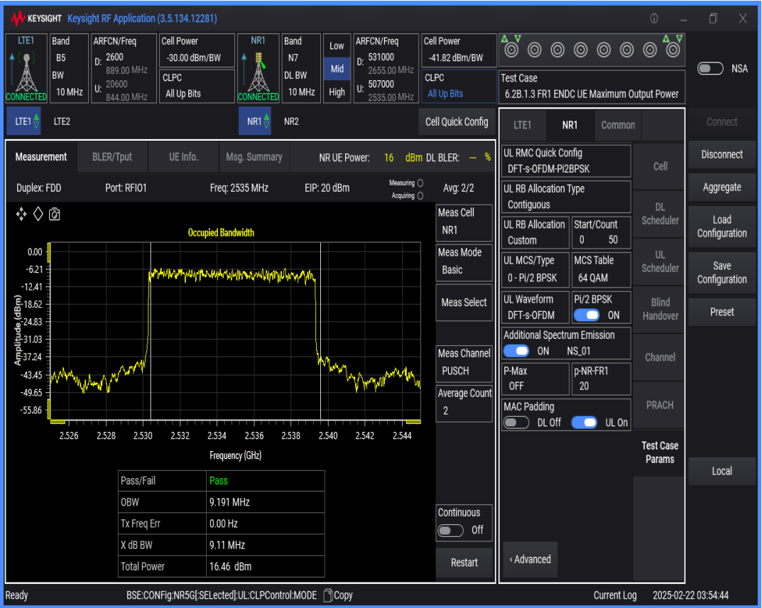
n7 SCS=15kHz DFT_BPSK BW=15MHz Channel=507000 RB=75@0
