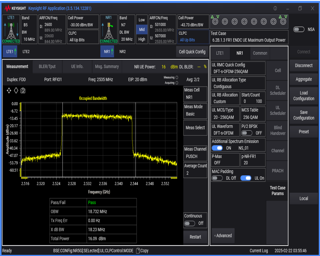
n7 SCS=15kHz DFT_QAM256 BW=15MHz Channel=507000 RB=75@0
