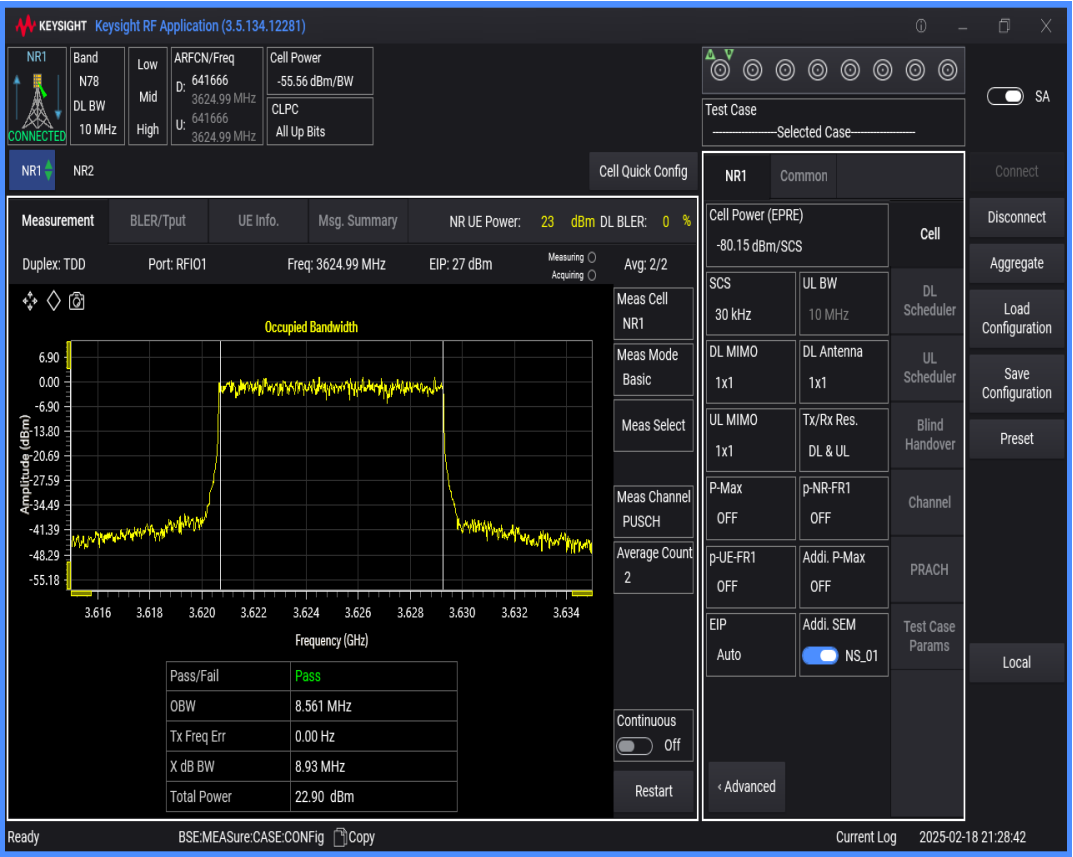
n78(3550-3700) SCS=30kHz DFT_QPSK BW=100MHz Channel=641666 RB=270@0
