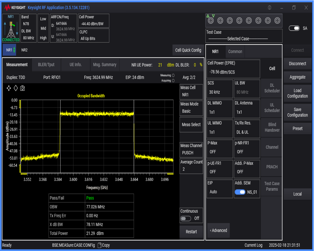
n78(3550-3700) SCS=30kHz DFT_QAM64 BW=90MHz Channel=641666 RB=240@0
