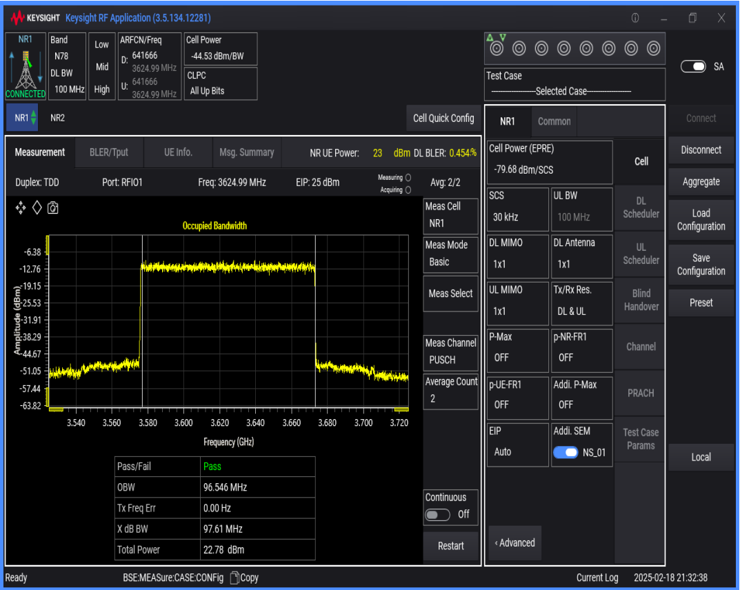
n78(3550-3700) SCS=30kHz DFT_QPSK BW=15MHz Channel=641666 RB=36@0
