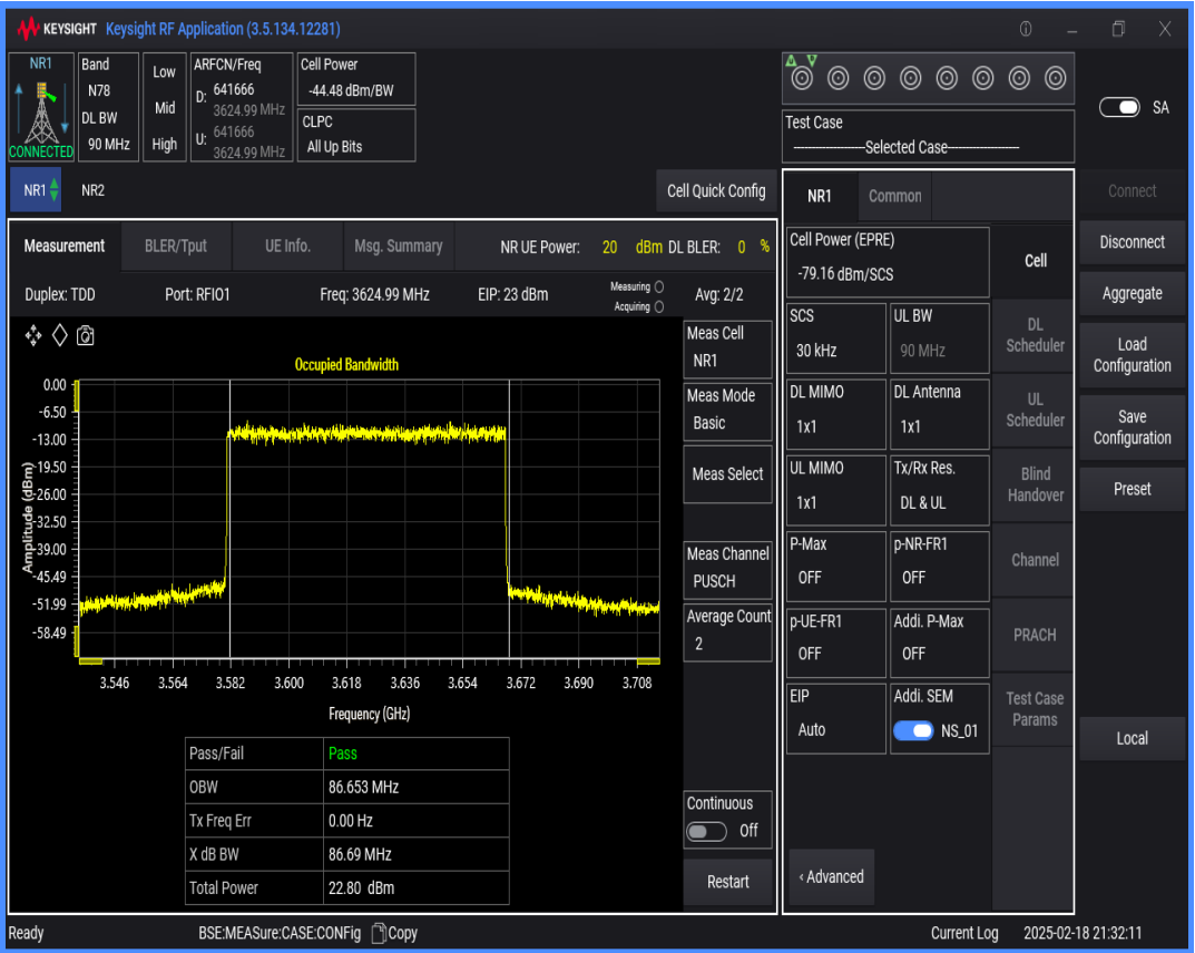
n78(3550-3700) SCS=30kHz DFT_QPSK BW=80MHz Channel=641666 RB=216@0
