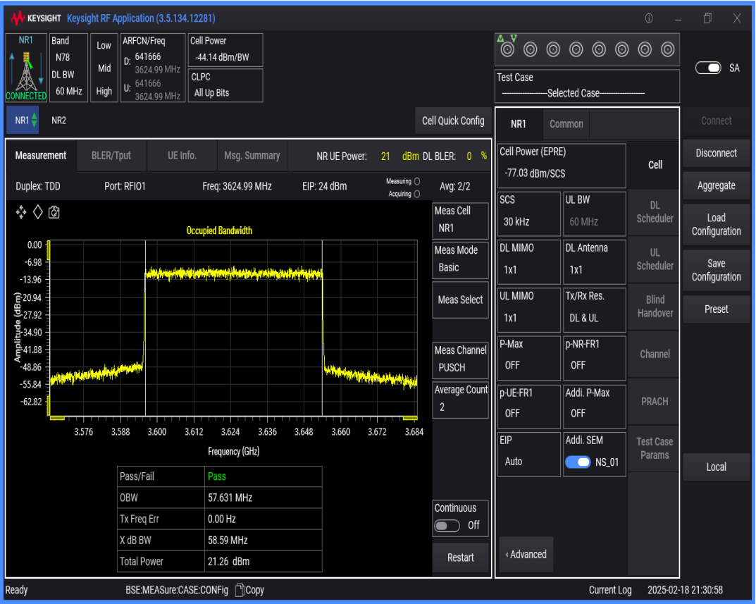
n78(3550-3700) SCS=30kHz DFT_QAM64 BW=70MHz Channel=641666 RB=180@0
