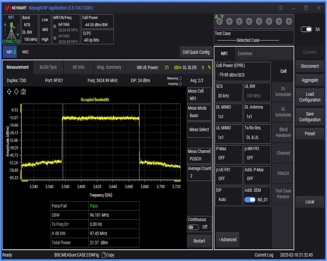
n78(3550-3700) SCS=30kHz DFT_QAM256 BW=80MHz Channel=641666 RB=216@0
