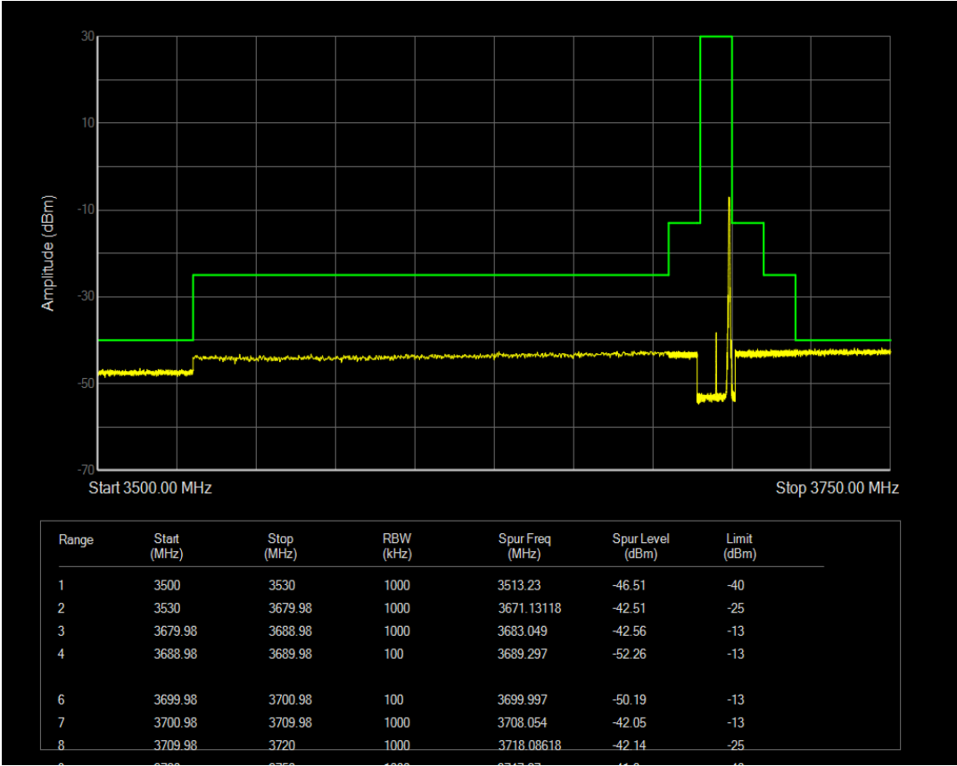
n78(3550-3700) SCS=30kHz CP_QPSK BW=50MHz Channel=638334 RB=133@0
