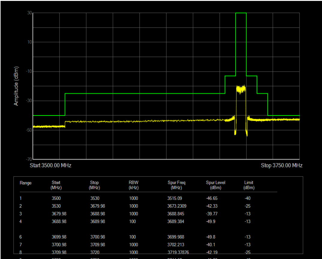
n78(3550-3700) SCS=30kHz CP_QPSK BW=10MHz Channel=646332 RB=1@23
