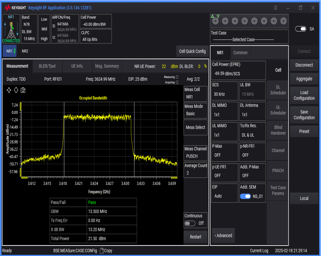
n78(3550-3700) SCS=30kHz DFT_QAM64 BW=100MHz Channel=641666 RB=270@0
