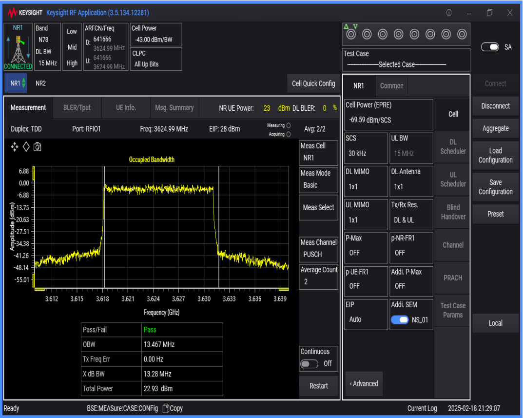
n78(3550-3700) SCS=30kHz DFT_QPSK BW=40MHz Channel=641666 RB=100@0
