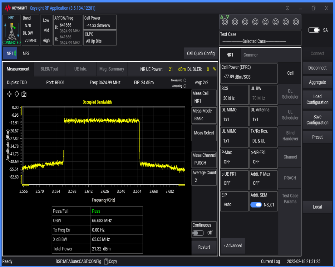
n78(3550-3700) SCS=30kHz DFT_QAM64 BW=80MHz Channel=641666 RB=216@0
