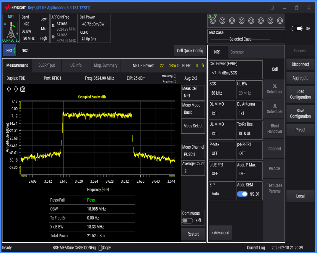
n78(3550-3700) SCS=30kHz DFT_QAM64 BW=50MHz Channel=641666 RB=128@0
