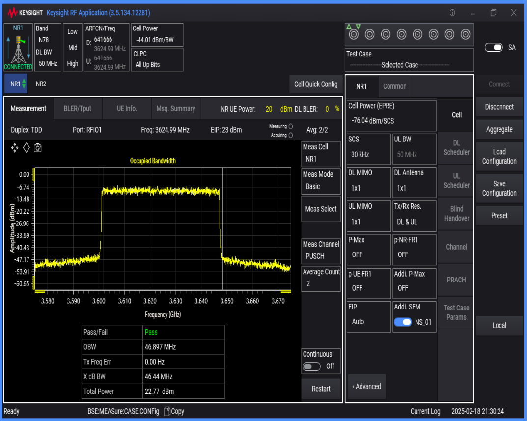
n78(3550-3700) SCS=30kHz DFT_QPSK BW=90MHz Channel=641666 RB=240@0
