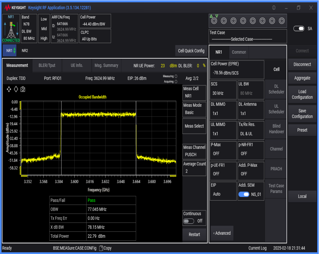
n78(3550-3700) SCS=30kHz DFT_QPSK BW=70MHz Channel=641666 RB=180@0
