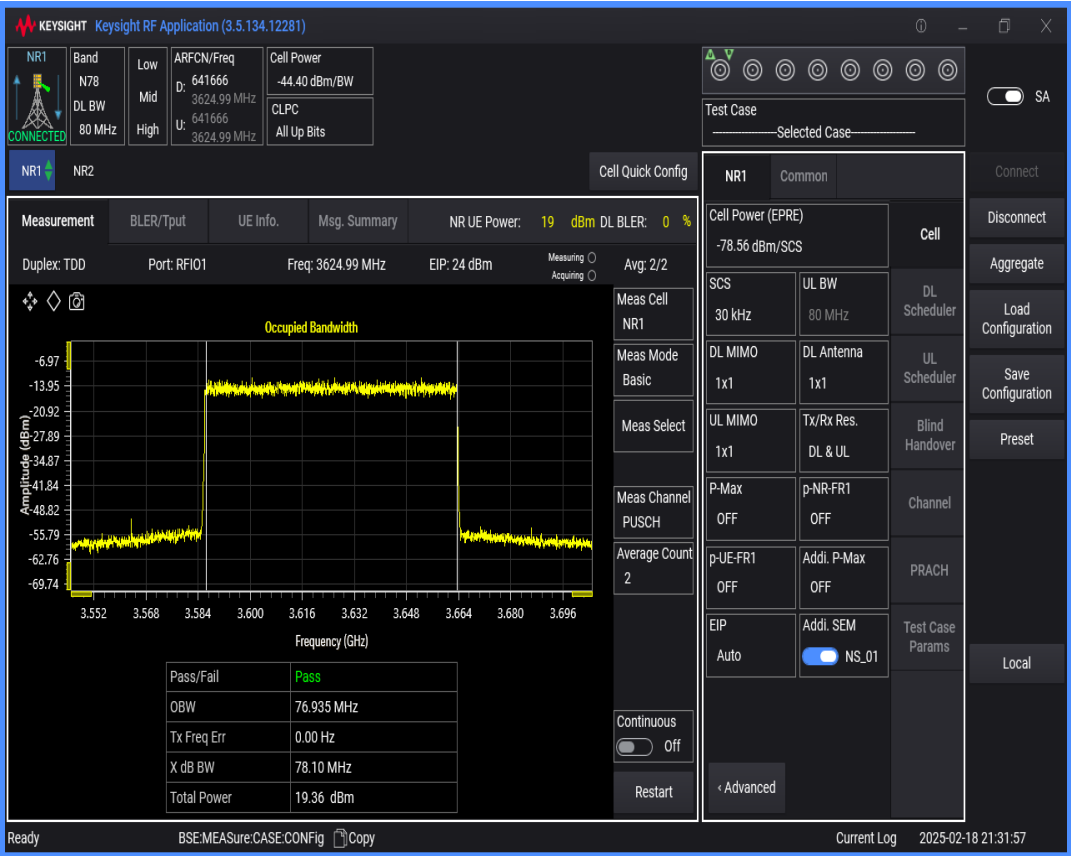
n78(3550-3700) SCS=30kHz DFT_QAM256 BW=90MHz Channel=641666 RB=240@0
