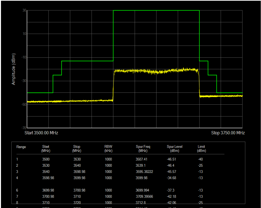
n78(3550-3700) SCS=30kHz CP_QPSK BW=100MHz Channel=643332 RB=1@272
