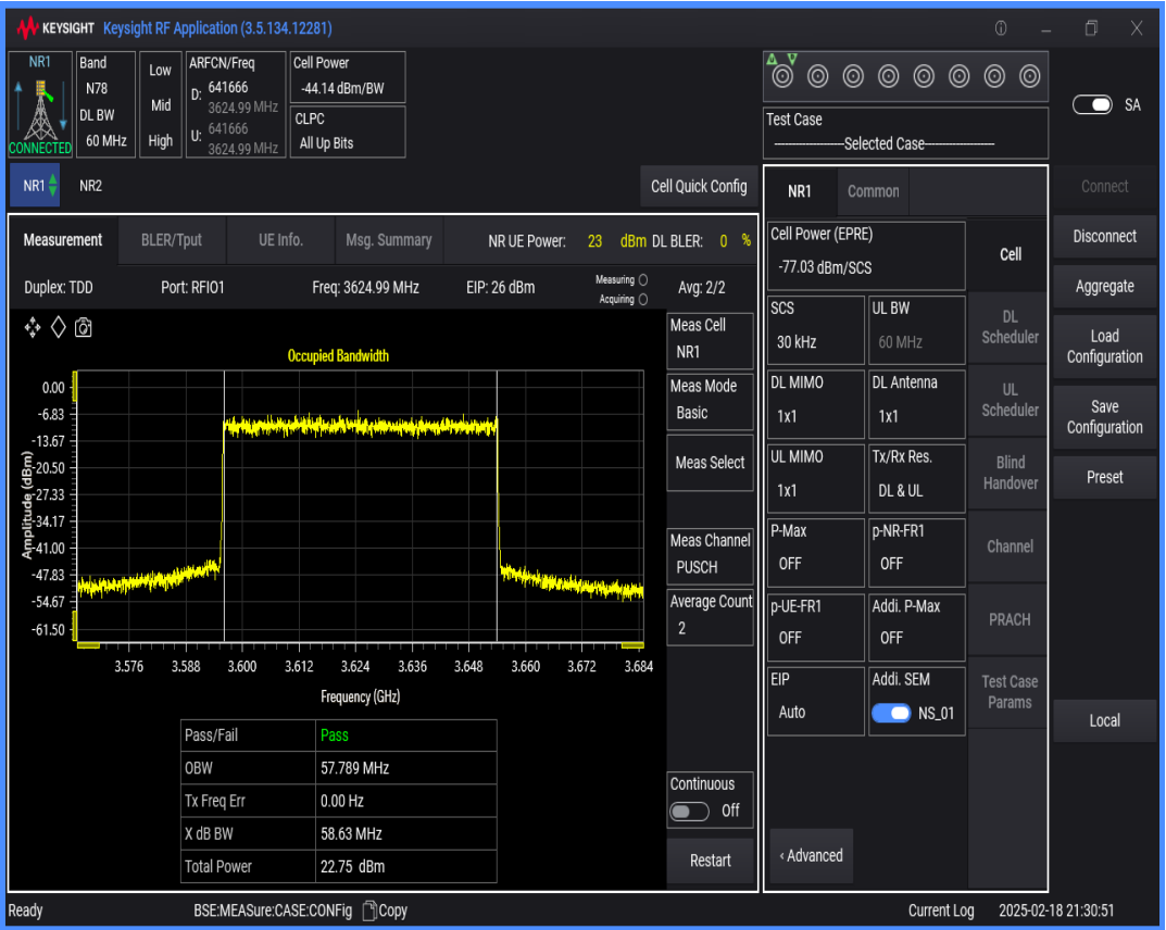
n78(3550-3700) SCS=30kHz DFT_QPSK BW=50MHz Channel=641666 RB=128@0
