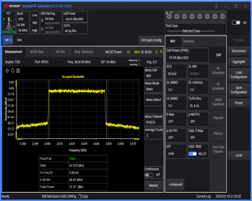
n78(3550-3700) SCS=30kHz DFT_QAM64 BW=40MHz Channel=641666 RB=100@0
