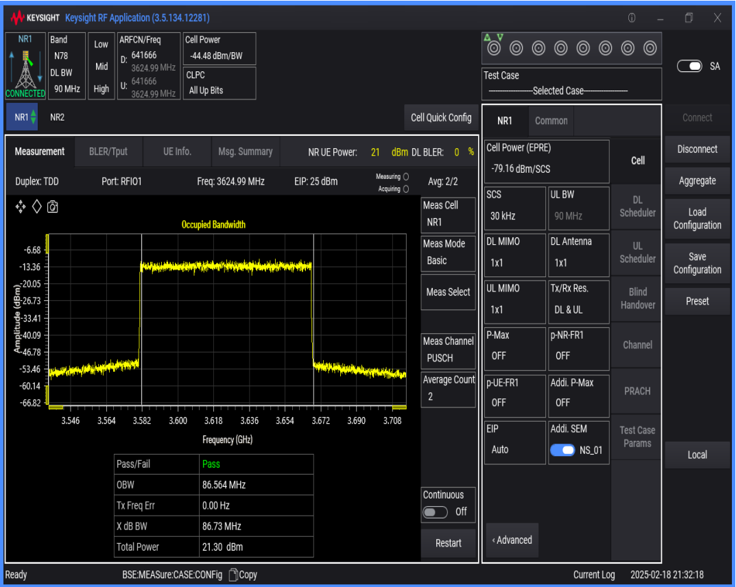
n78(3550-3700) SCS=30kHz DFT_QPSK BW=10MHz Channel=641666 RB=24@0
