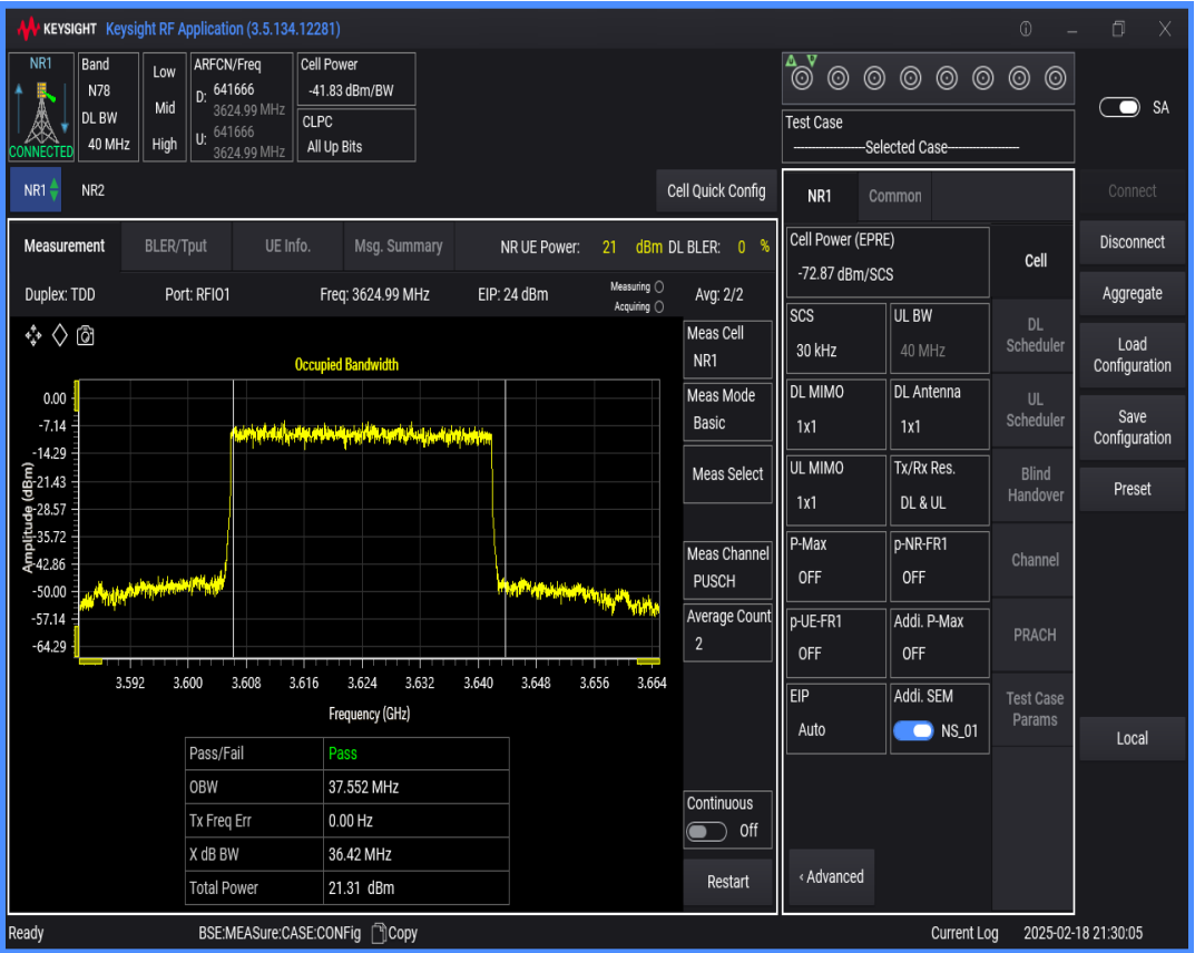
n78(3550-3700) SCS=30kHz DFT_QAM64 BW=60MHz Channel=641666 RB=162@0
